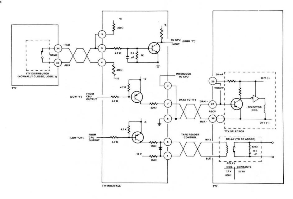
Figure 10-6 TTY Interface Circuit
