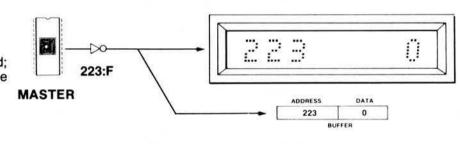
4. DUP/VER Buffer-to-Copy Buffer data is inverted prior to display; in DUP, Copy PROM is programmed with inverted data.
