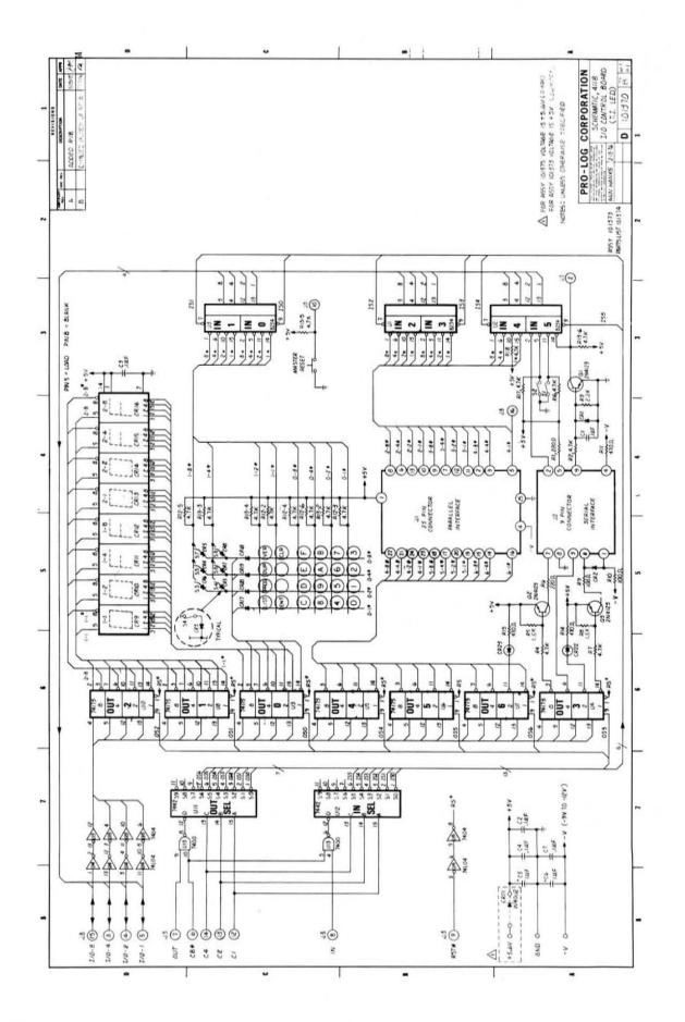
Schematic; 4118 I/O Control Board (T.I. LED)
