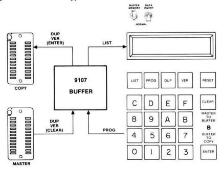
Figure 6-1 M900B Control Panel
