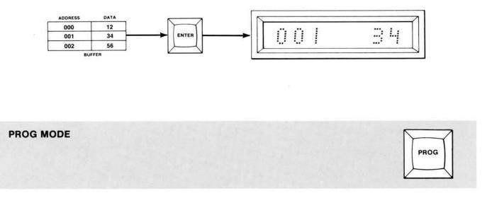
In PROG mode, the display now shows the 3-digit address specified to be the start location, and awaits an operator entry of data from the keyboard.
