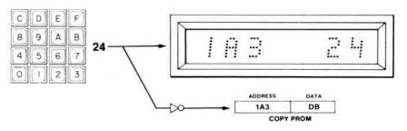
3. DUPLICATE Master to Copy True Master PROM and corrections displayed; inverted data programmed into Copy.
