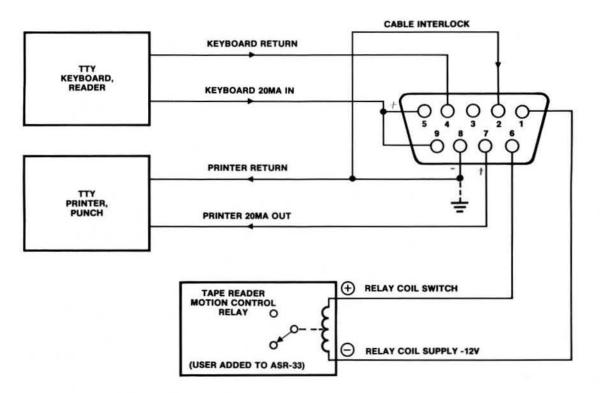
Figure 10-1 Serial Interface Connector Block Diagram
