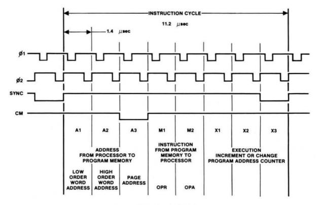
Figure 15-2 Control Timing
