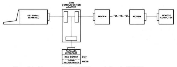
Figure 8-1 Interconnection for 9108 Communications to M900B Programmer
