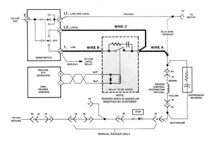
Figure 10-11 TTY Modification (Manual Reader)
