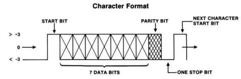
**Even Parity Enable (EPE)** - Selects whether even or odd parity is generated. The M304 is shipped in the even parity enable position. To select odd parity, remove jumper between E19, E20, and install between E20, E21. Parity is not used by the M900B when receiving. However, it must be sent either ODD, EVEN or fixed.
