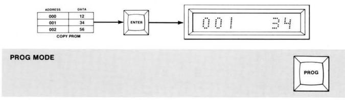
In PROG mode, the display now shows the address specified to be the start location, and awaits an operator entry of data from the keyboard.
