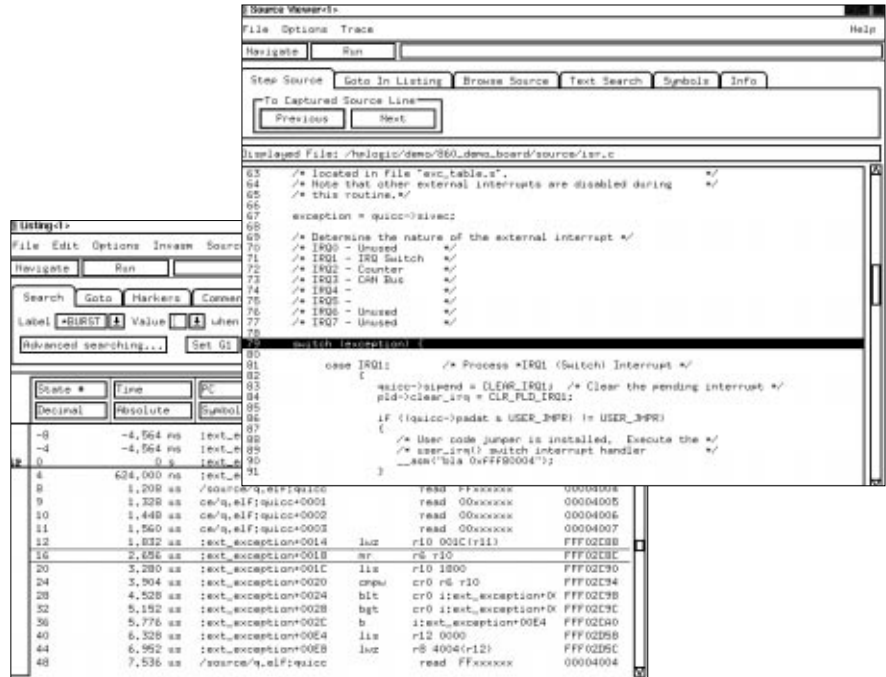
Figure 8: Inverse Assembled Trace Time-Correlated to Source Code Using the HP Source Correlation Tool Set
