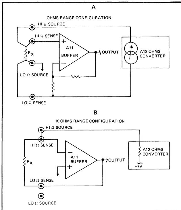
Figure 3-2. OHMS AND K OHMS RANGE CONFIGURATION
