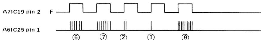
Correct input but incorrect outputs are indicative of counter malfunction.
