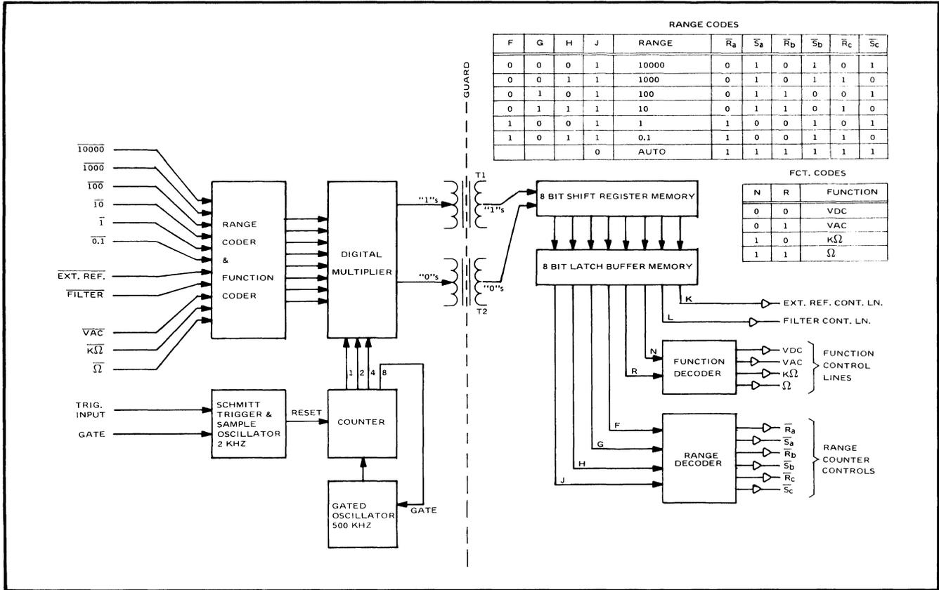
Figure 6-1. 8400A REMOTE CONTROL UNIT BLOCK DIAGRAM
