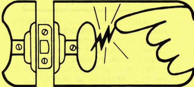
Some semiconductors and custom IC's can be damaged by electrostatic discharge during handling. This notice explains how you can minimize the chances of destroying such devices by:
