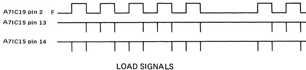
If the load commands are correct, then something may be wrong with the operation of one of the shift registers. If replacement does not solve the problem, one of the shift register output may be shorted.
