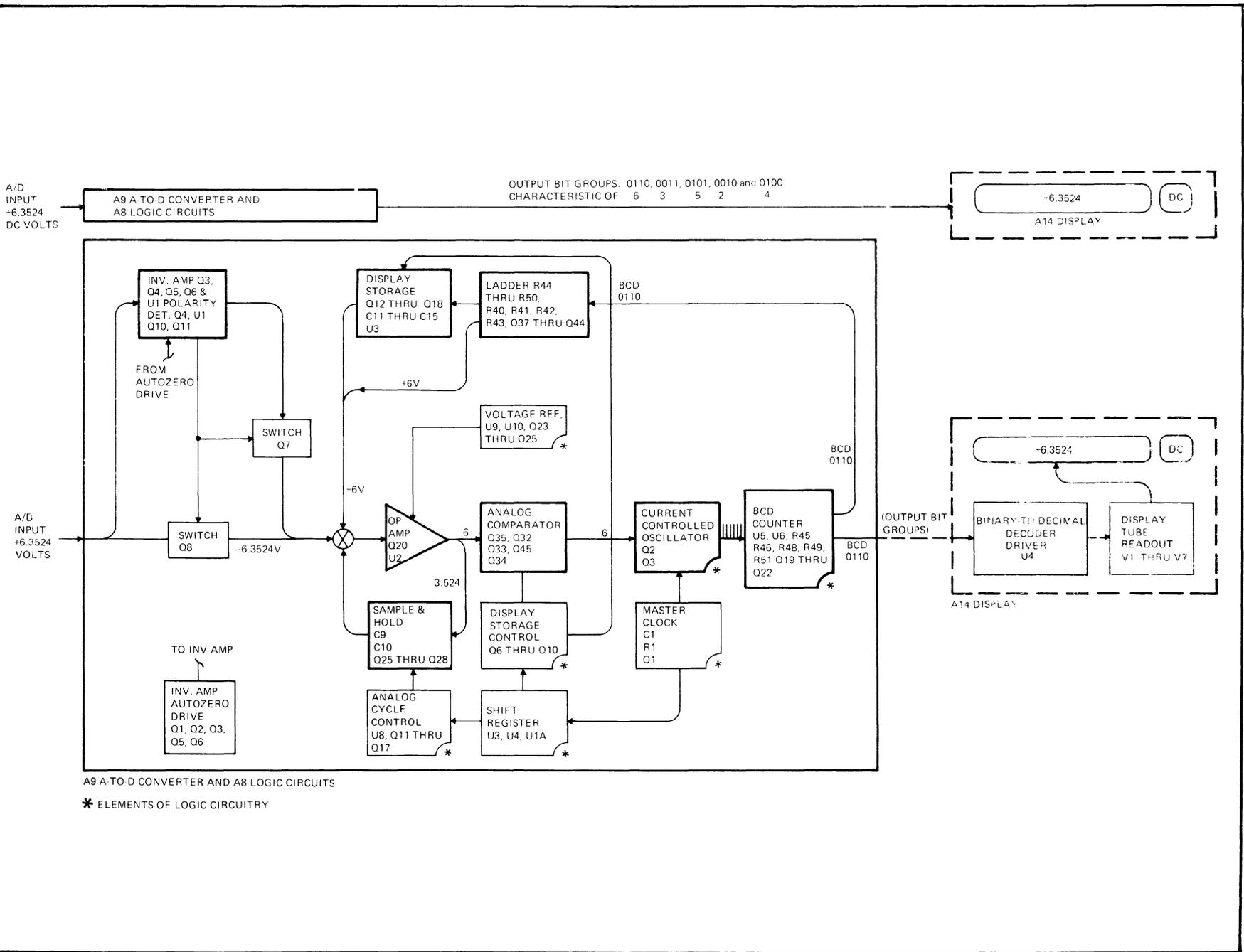
3-43. The polarity detector consists of flip-flop Q10, Q11, and associated circuitry. The flip/flop employs base triggering, which is applied through diode CR6 to the base of Q10. The gate signal, gate 4, is applied to the emitters of Q10 and Q11 and enables the detector during the A sub-period of the measure period. During the remainder of the measure period, the plus and minus gates (Q8 and Q7, respectively) are turned off and the polarity information is retained by the display circuitry.
