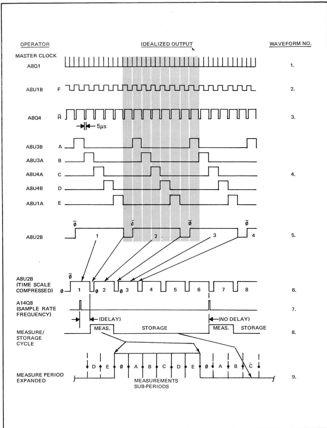
Figure 3-9. DVM TIMING AND SYNCHRONY DIAGRAM (SHEET 1)
