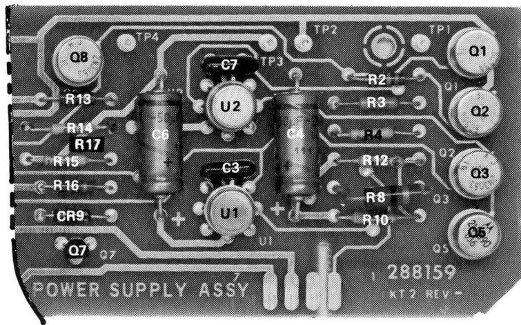
Figure 5-2. POWER SUPPLY PCB ASSEMBLY
