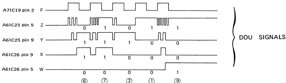
Again, correct counter operation is indicative of a problem in registration gates IC22, IC23 and IC24.
