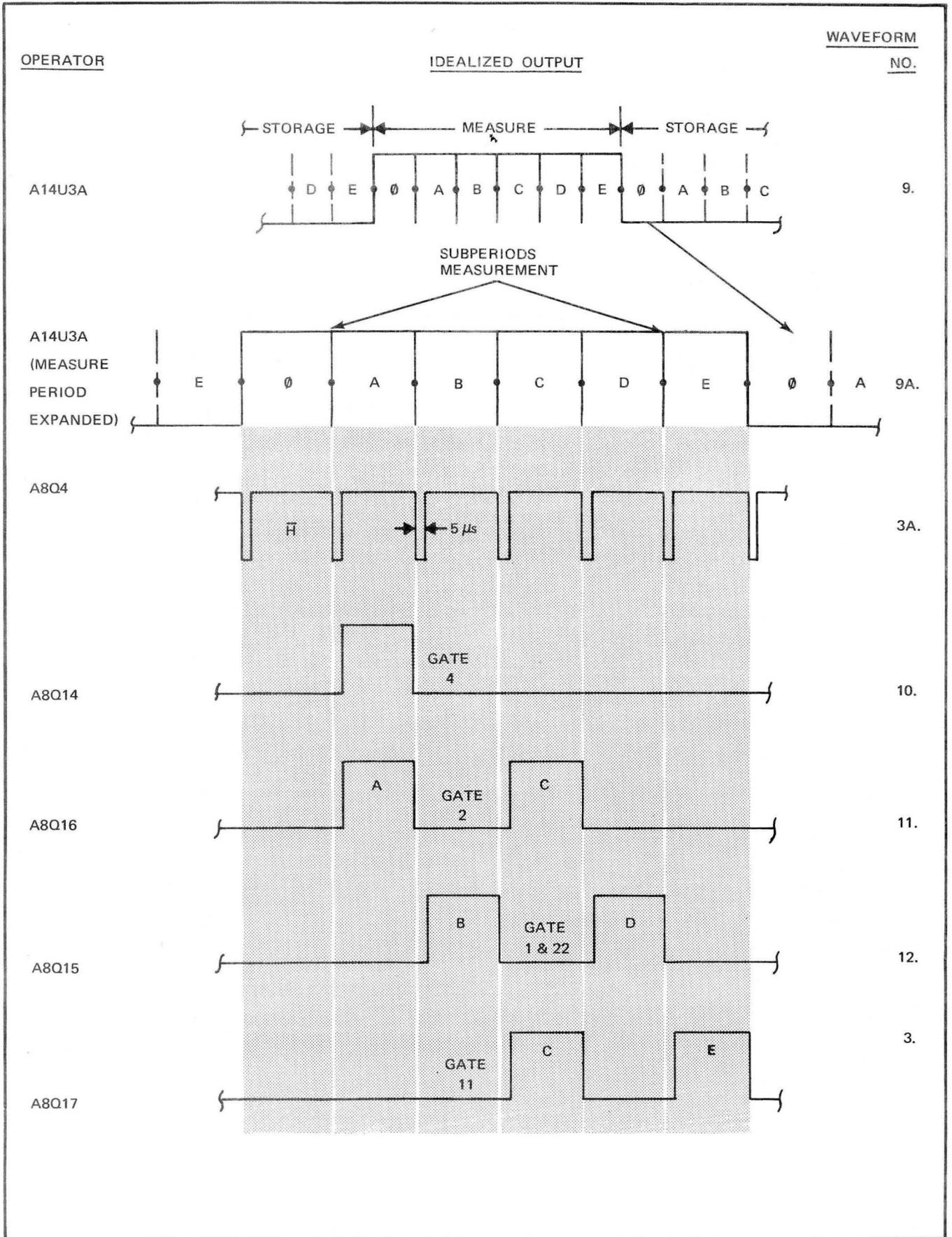
Figure 3-9. DVM TIMING AND SYNCHRONY DIAGRAM (SHEET 2)
