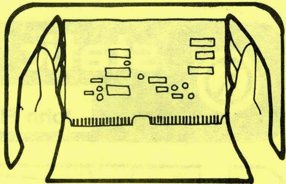
8. WHEN REMOVING PLUG-IN ASSEMBLIES, HANDLE ONLY BY NON-CONDUCTIVE EDGES AND NEVER TOUCH OPEN EDGE CONNECTOR EXCEPT AT STATIC-FREE WORK STATION. PLACING SHORTING STRIPS ON EDGE CONNECTOR HELPS TO PROTECT INSTALLED SS DEVICES.
