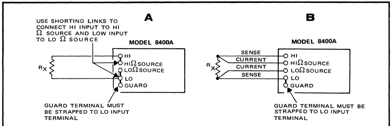
Figure 2-11. PROPER GUARD CONNECTIONS FOR (A) 2-TERMINAL  $\Omega$  MEASUREMENTS WHEN SIGNAL LEADS ARE SHORT AND (B) 4-TERMINAL  $\Omega$  MEASUREMENTS ON 10 $\Omega$  THROUGH 10,000 $\Omega$  RANGES
