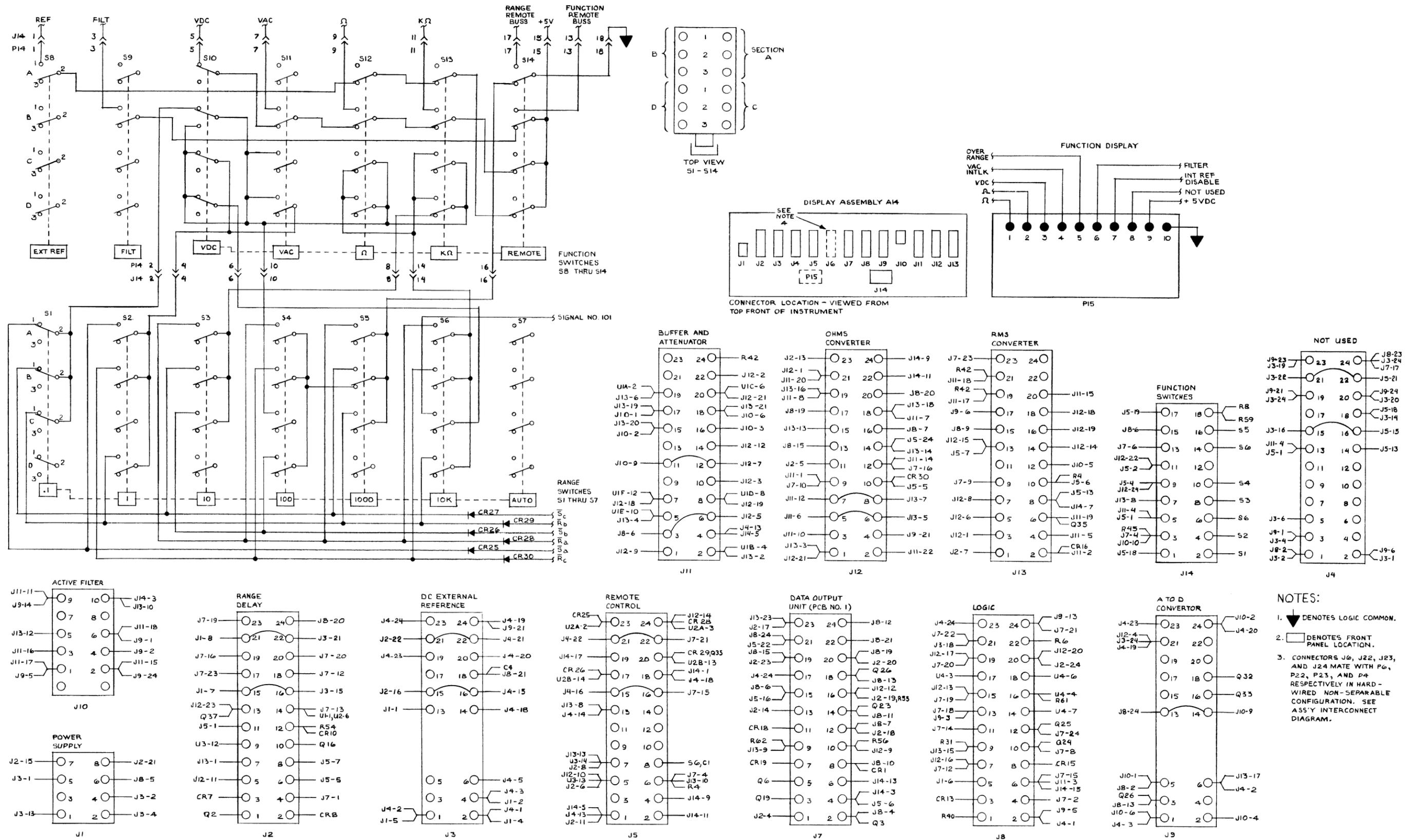
FIGURE 8-16 A14 DISPLAY PCB ASSEMBLY SHEET 1 of 2 (8400A)
