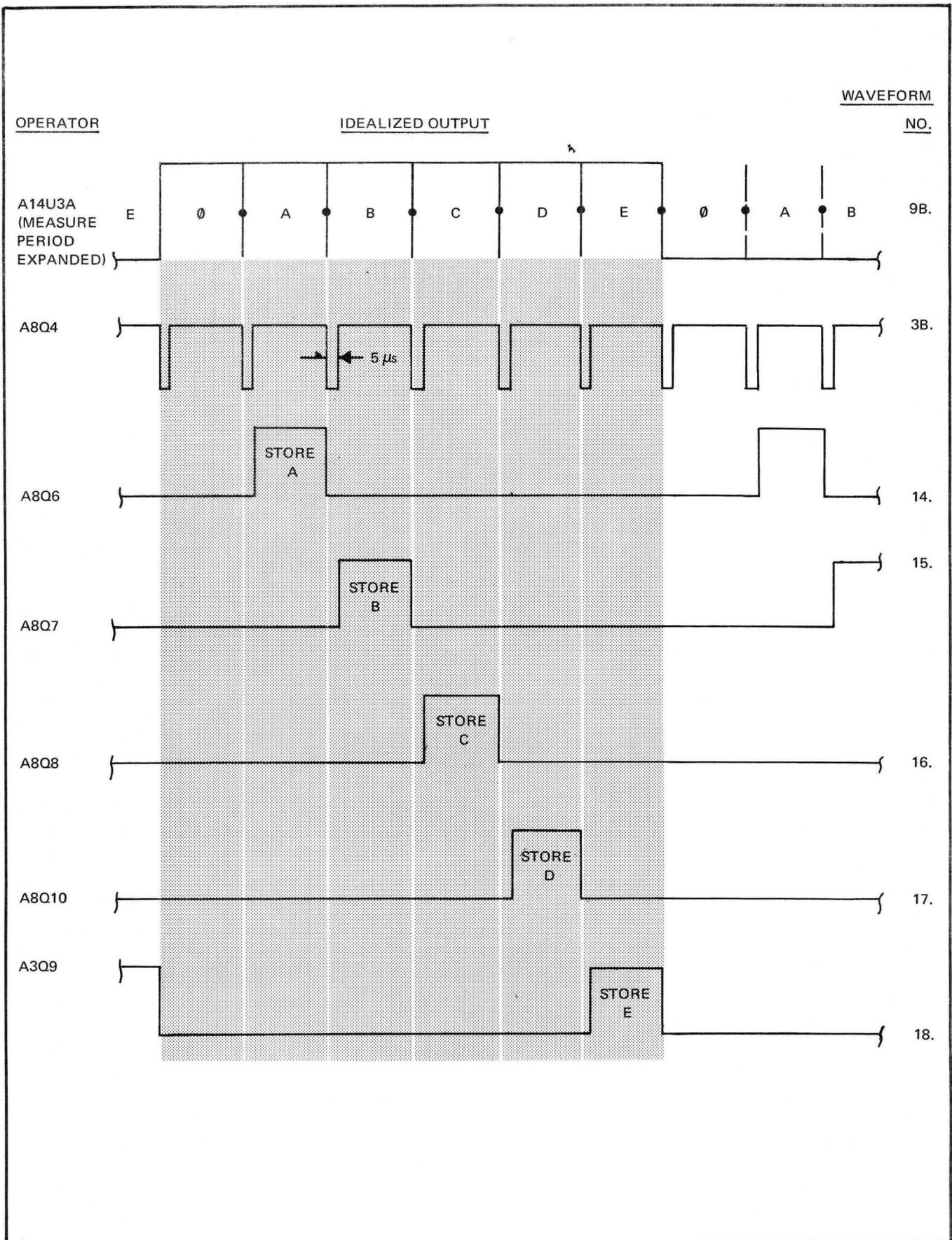
Figure 3-9. DVM TIMING AND SYNCHRONY DIAGRAM (SHEET 3)
