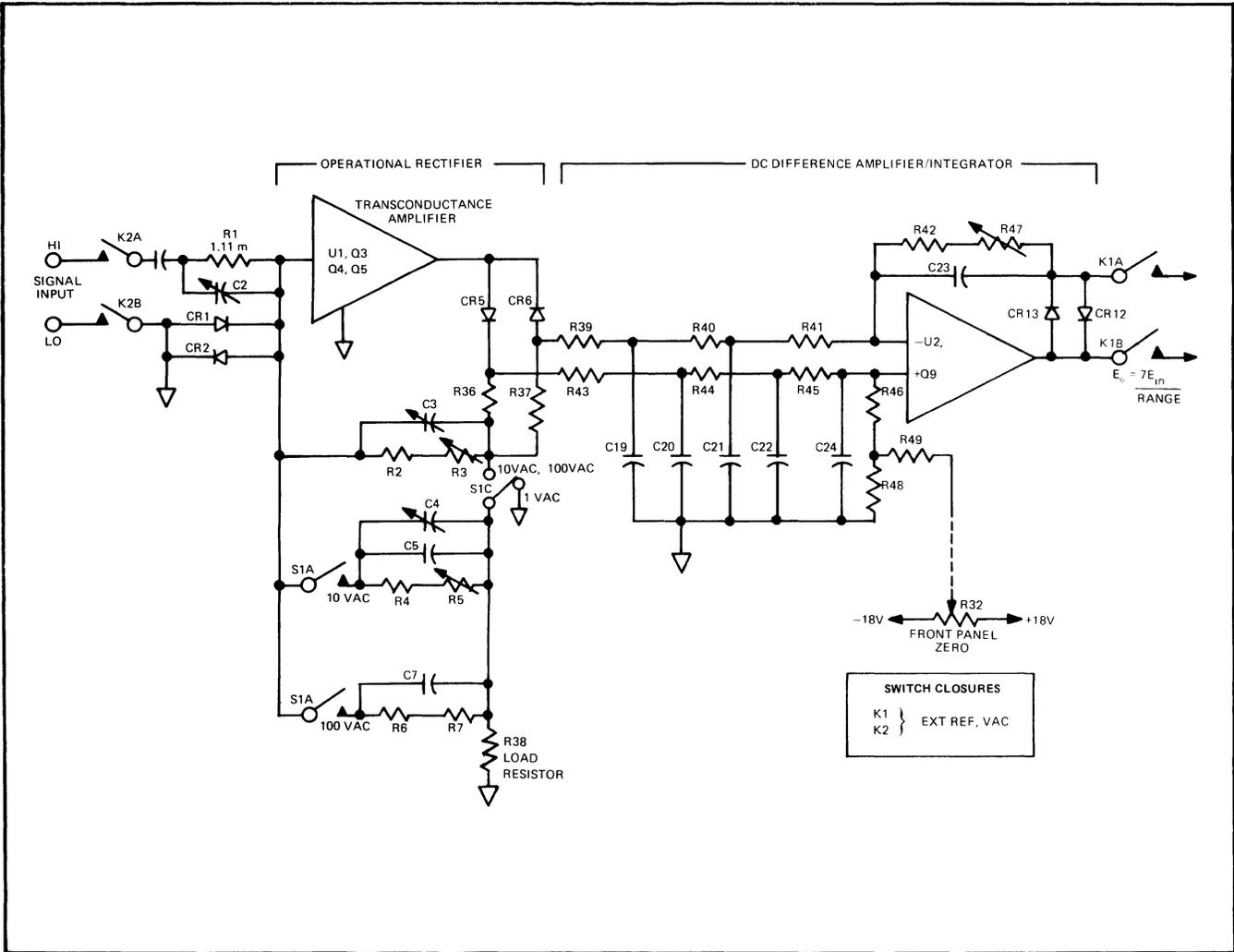
Figure 6-1. BLOCK DIAGRAM AC EXTERNAL REFERENCE CONVERTER.
