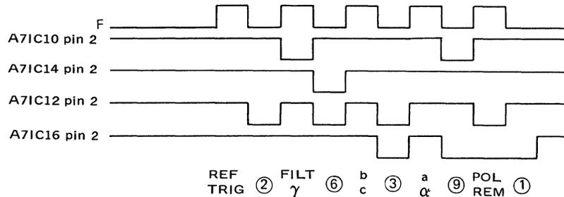
4. **DOU LOAD COMMANDS CORRECT?** Refer to the following load signals. Use the same setup as in part 3 of this figure. A dual-trace scope is useful.
