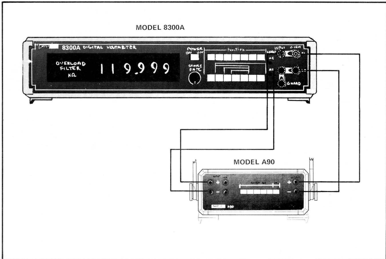
Figure 6-7. EQUIPMENT CONNECTIONS – .1 MA AND 1 MA RANGE CHECKS
