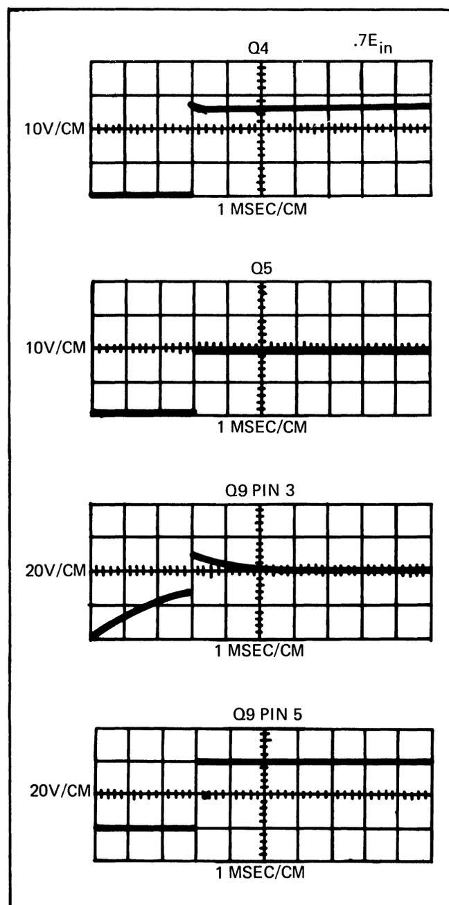
Figure 4-24. DC External Reference Stylized Waveforms
