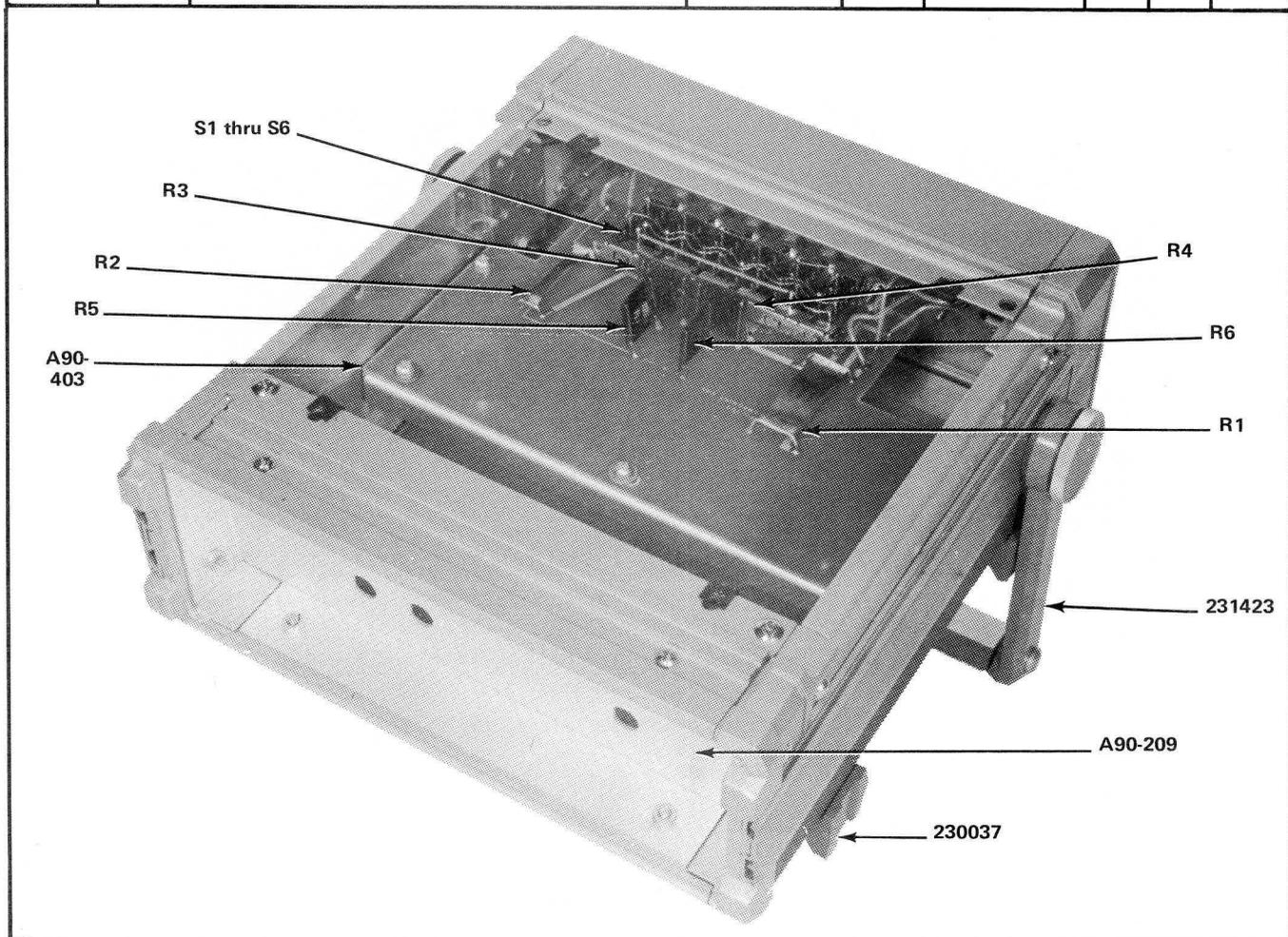
Figure 6-9. MODEL A90 CURRENT SHUNT (Sheet 2 of 2)
