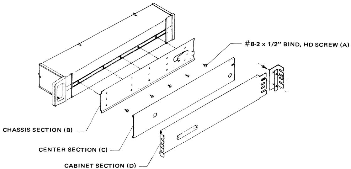
1. REMOVE SIDE TRIM DECAL AND BOTTOM FEET FROM INSTRUMENT.
