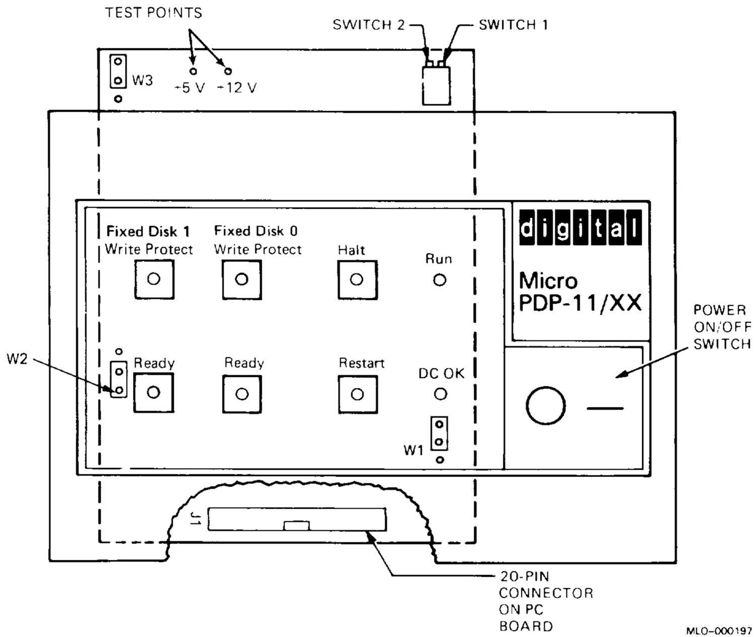
Table 1-1 describes the functions of the controls and indicators on both the 4- and 6-button control panels.
