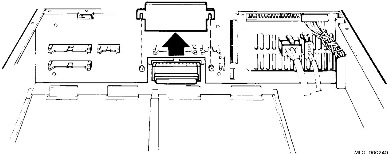
3. Disconnect the RQDX interconnect cable behind the access door opening. Move the cable to the side, to provide working room.
