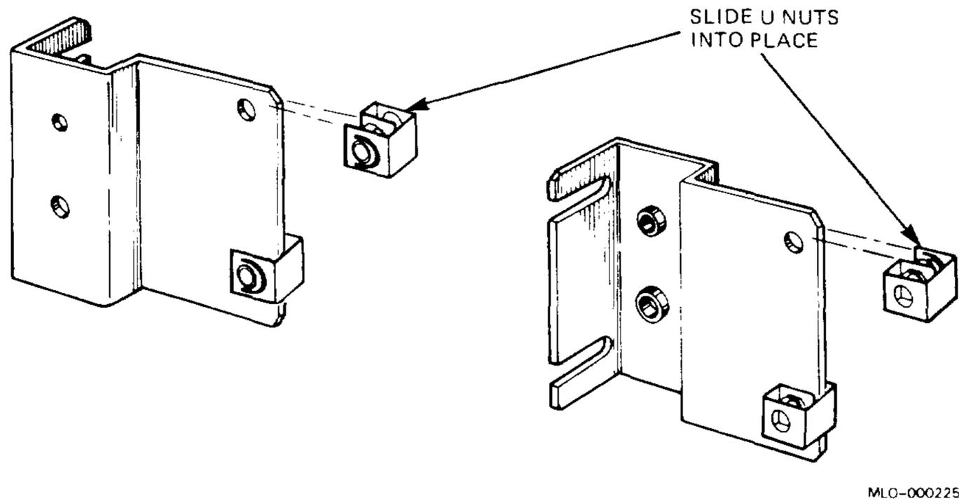
3. Mount the left and right rear brackets onto the rails (Figure 2-19). Use four Phillips machine screws with lock washers.
