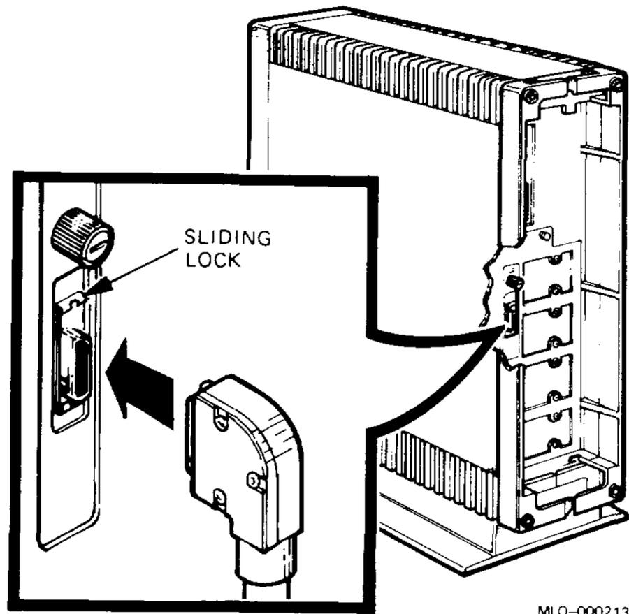
2. Connect the other end of the cable to one of the following devices:
