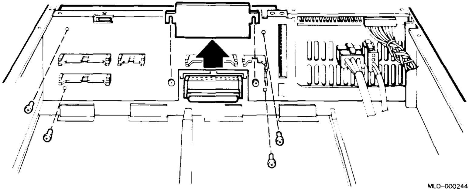
13. Pivot the left side (CD rows) of the backplane assembly 45 degrees toward the rear, then lift the backplane straight up (Figure 3-13).
