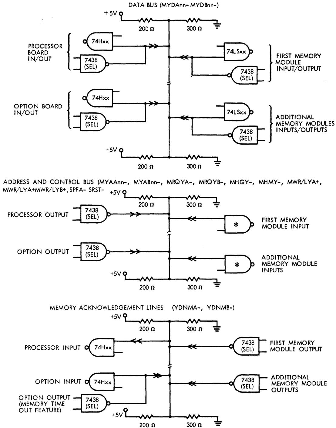
\*FOR MYAAnn-, MYABnn-, MHGY-, MHMY-, MWR/LYA+ MWR/LYB+, SPFA-, AND SRST- TYPE 74LSxx INTEGRATED CIRCUITS ARE USED. (nn- is 00 THROUGH 11)
