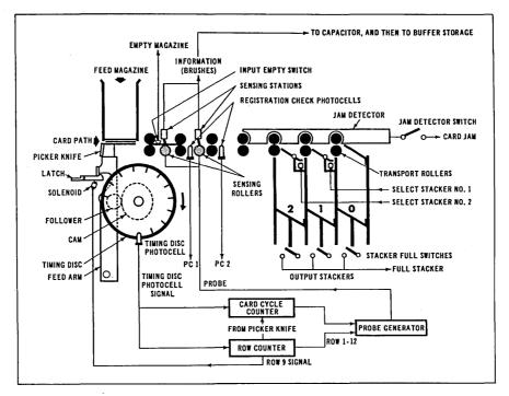
Figure 9 Electromechanical Schematic of Card Reader
