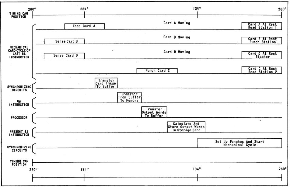
Figure 14 General Timing Diagram
