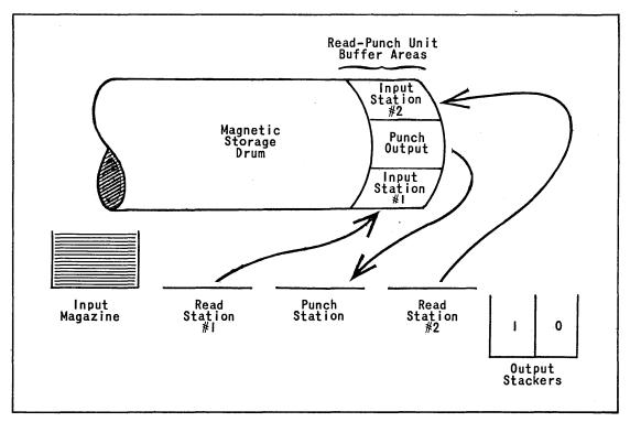
Figure 13 Functional Diagram Of The Read-Punch Unit
