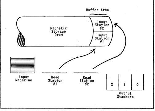
Figure 2 Functional Diagram Of The High-Speed Reader
