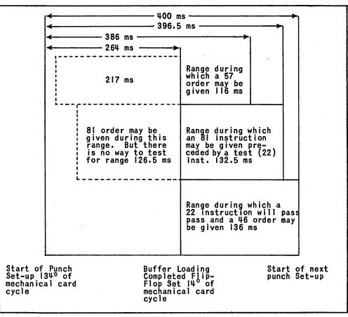
Figure 19 Diagram of Read-Punch Operating Cycle
