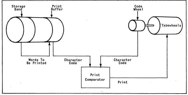
Figure 23 General Block Diagram of Print Operation
