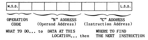
The "m" address is usually the address of a word in storage. The "operation code" tells the computer what to do with this word; and the "c" address is the storage location of the next instruction word. These fields may have different significance for some special instructions.
