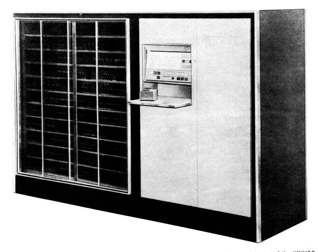
The **CENTRAL PROCESSOR** is the control center of the UNIVAC Solid-State Computer. It houses the arithmetic and logical circuitry, the data storage system, the power supply system, and the operator's panel and keyboard.
