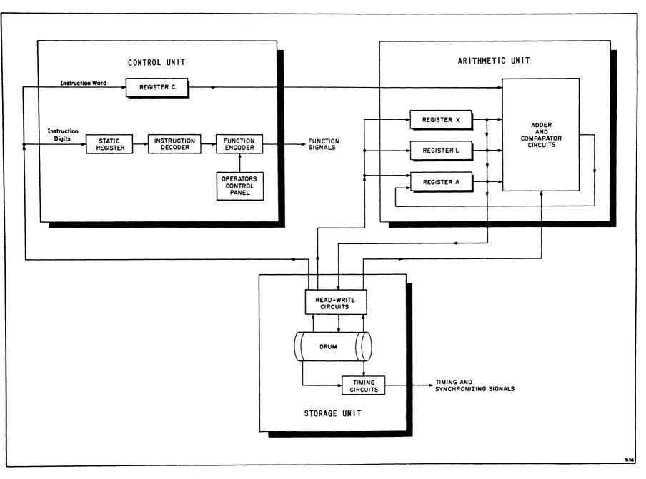
Figure 4. Central Processor Units
