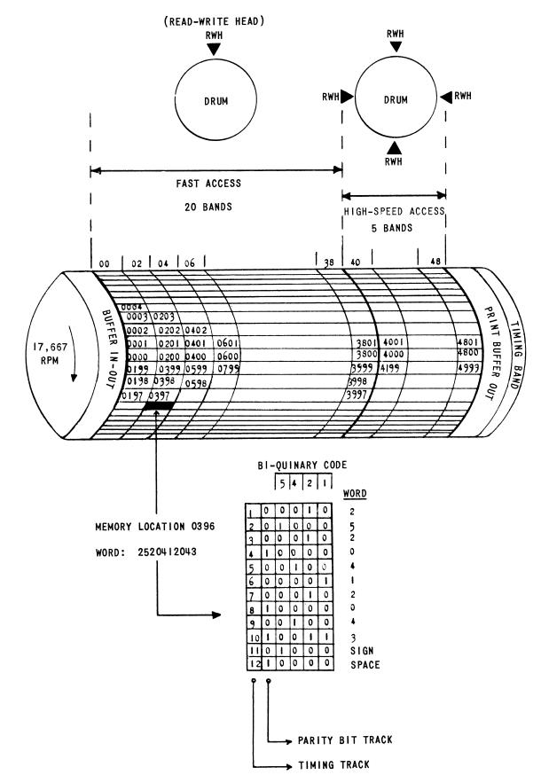
Figure 1. Magnetic Storage Drum
