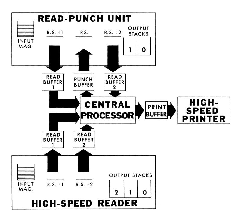
Figure 3. Buffer Operation
