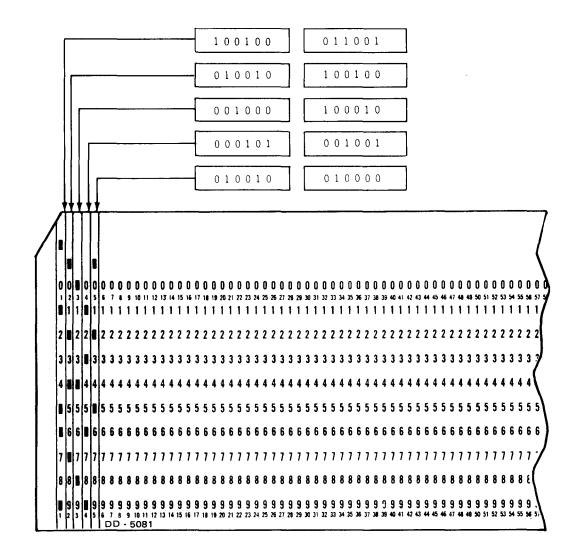
Figure 6-6. Relationship of Data Bytes to Card Punches (Image Mode)
