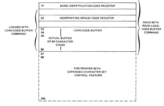
Figure 7—6. Load Code Buffer Array
