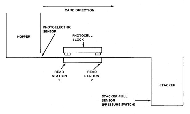
Figure 5—4. Card Path Through Card Reader
