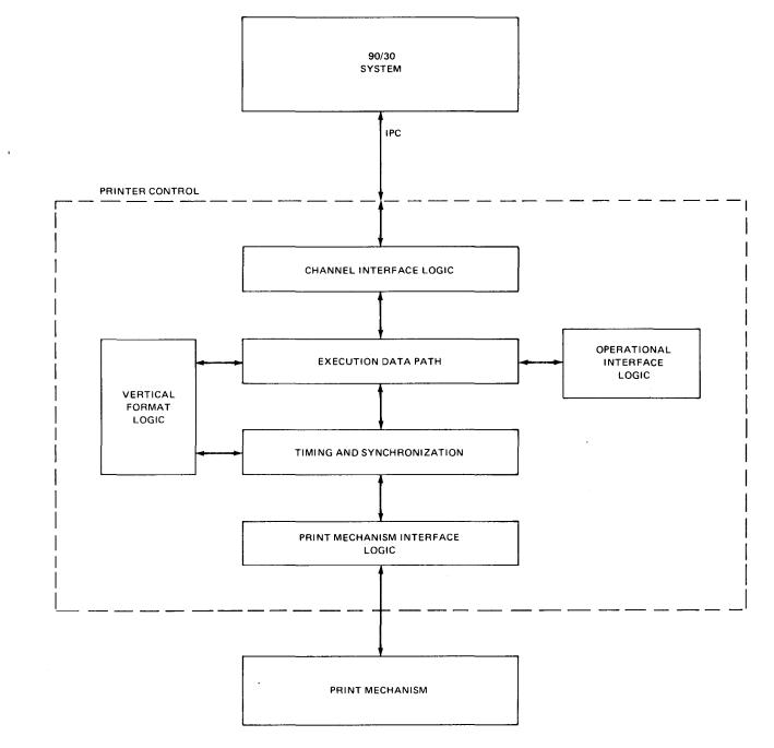
Figure 7-4. Printer Control Circuitry
