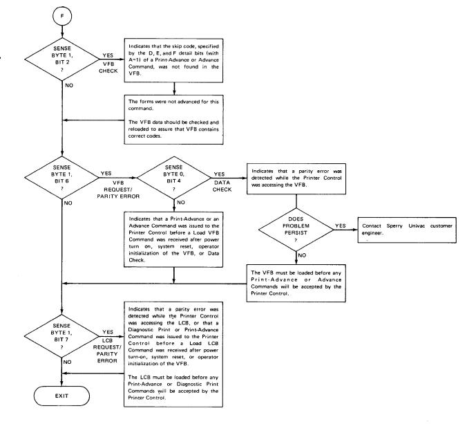
Figure 7—18. Buffer Error Recovery Flowchart (Part 2 of 2)
