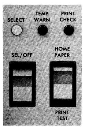
Figure 4—6. Console Printer Operator Panel
