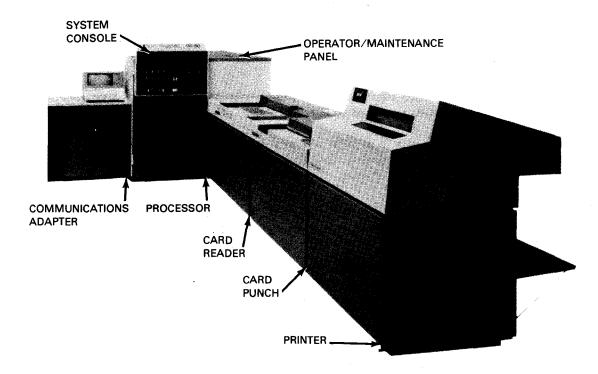
Figure 1—1. 90/30 System With Integrated Peripheral Devices
