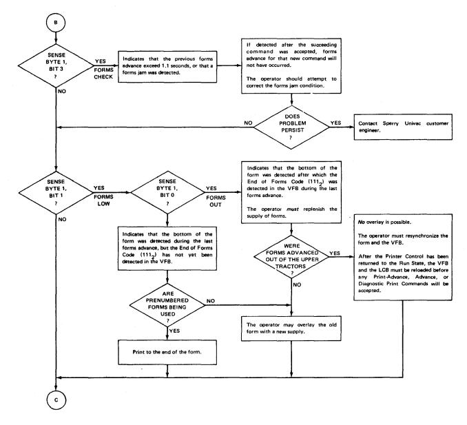
Figure 7-17. Equipment Check Error Recovery Flowchart (Part 1 of 2)
