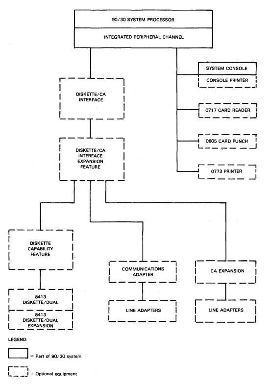
Figure 2-1. Configuration of Integrated Peripheral Devices Used With Integrated Peripheral Channel
