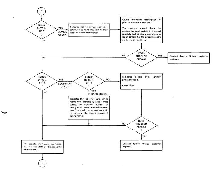
Figure 7—17. Equipment Check Error Recovery Flowchart (Part 2 of 2)
