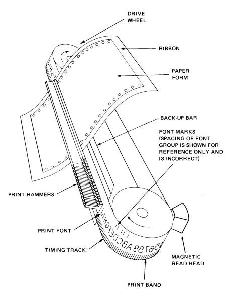
Figure 7—11. Print Function, Schematic Diagram
