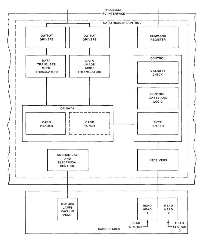
Figure 5-3. Card Reader Control, Block Diagram
