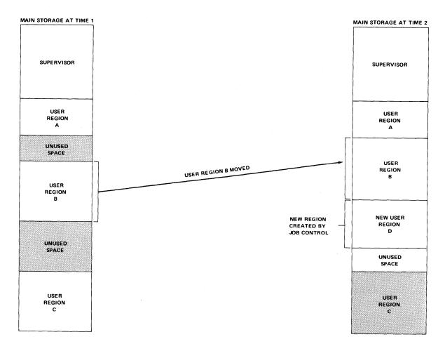
Figure 6-1. Main Storage Compaction by Rollout/Rollin (moving only)
