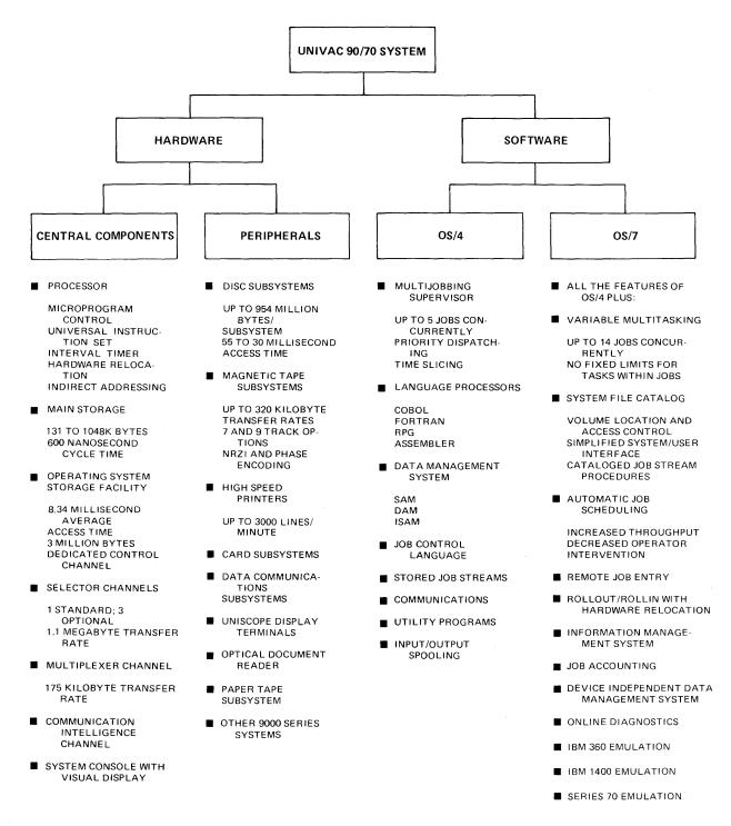
Figure 2-1. Highlights of UNIVAC 90/70 System Hardware and Software
