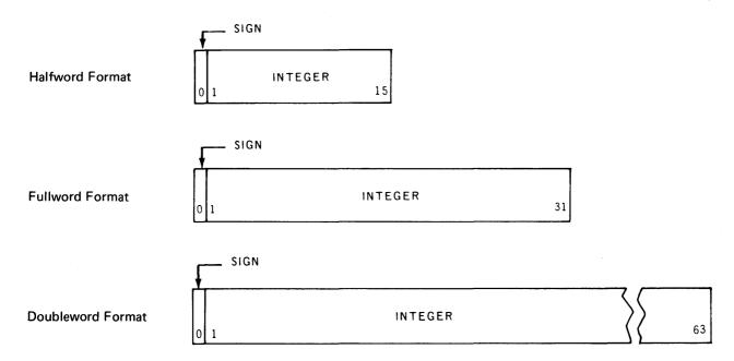
When held in one of the 16 general registers, a fixed-point number is generally treated as a 32-bit operand. When a halfword fixed-point number is called from storage and loaded into a register, the sign is extended to the left to fill the fullword register. The contents of the register are then handled as a fullword operand in fixed-point arithmetic operations.
