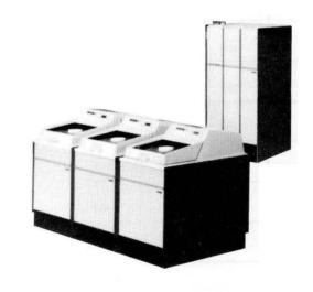
UNIVAC 8411/8414 Disc Subsystem
