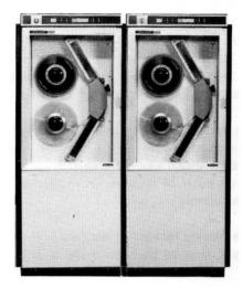
The UNISERVO VI-C Magnetic Tape Subsystem is a low cost magnetic tape subsystem which comprises a control and from two to eight magnetic tape units. The master/slave concept is employed in the logic of the UNISERVO VI-C Magnetic Tape Subsystem. The master unit, having the power supply and control circuitry, governs the functions of up to three slave magnetic tape units. However, all units are treated alike from a programming or operating system viewpoint.
