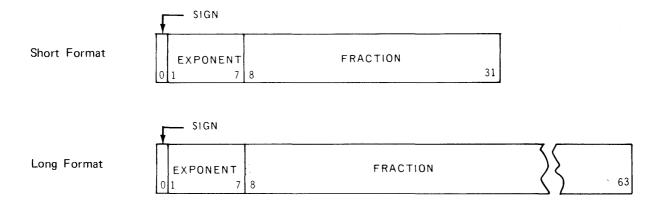
The floating-point instruction set provides for loading, adding, subtracting, comparing, multiplying, dividing, storing, and sign control of short or long format operands. Short format operands provide faster processing and require less storage space than long format operands. Long format operands provide greater precision in computation.
