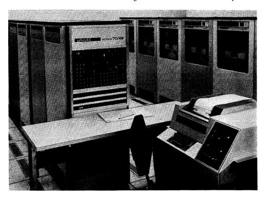
The Series 70/46 Time-Sharing System is the virtual-memory version of the medium-scale 70/45 system. A 70/46 can service up to 48 users at remote terminals while concurrently processing up to 14 independent batch-mode jobs. Force between RCA and UNIVAC, RCA will continue to manufacture Series 70 hardware for the next several years under a complicated structure of royalty payments, OEM relationships, service agreements, etc.
