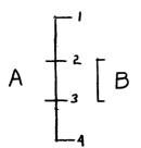
Monitoring will be done in Mode A from points 1 through 2, in Mode B from points 2 through 3, in Mode A from points 3 through 4. After point 4 the program will resume operation in highspeed mode.
