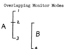
Monitoring will be done in Mode A from point 1 to point 2, in Mode B from points 2 through 4, and in Mode A again from point 4 until and unless the program happens to return to a point between points 1 and 3. Mode A cannot be terminated (unless canceled) until the instruction at point 3 is actually executed.
