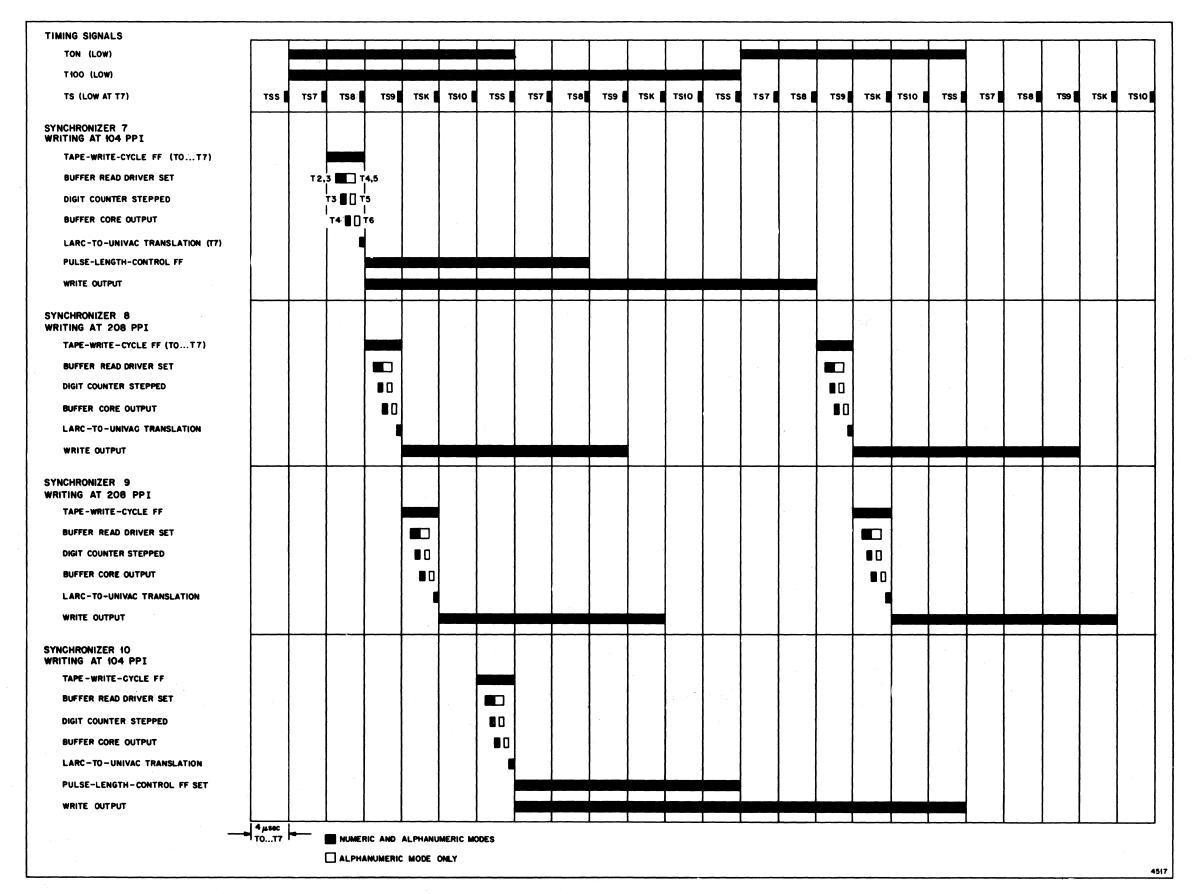
Figure 5-1. Write Cycle Timing, Larc System, Serial 1 The signal that sets the write-sprocket flip-flop is delayed for 0.5  $\mu$ sec and tests STUEA from the output odd-even checker. If an error was detected in the translated combination, all seven of the write-output flip-flops are set, thereby replacing the translated combination with a combination consisting of all 1's.
