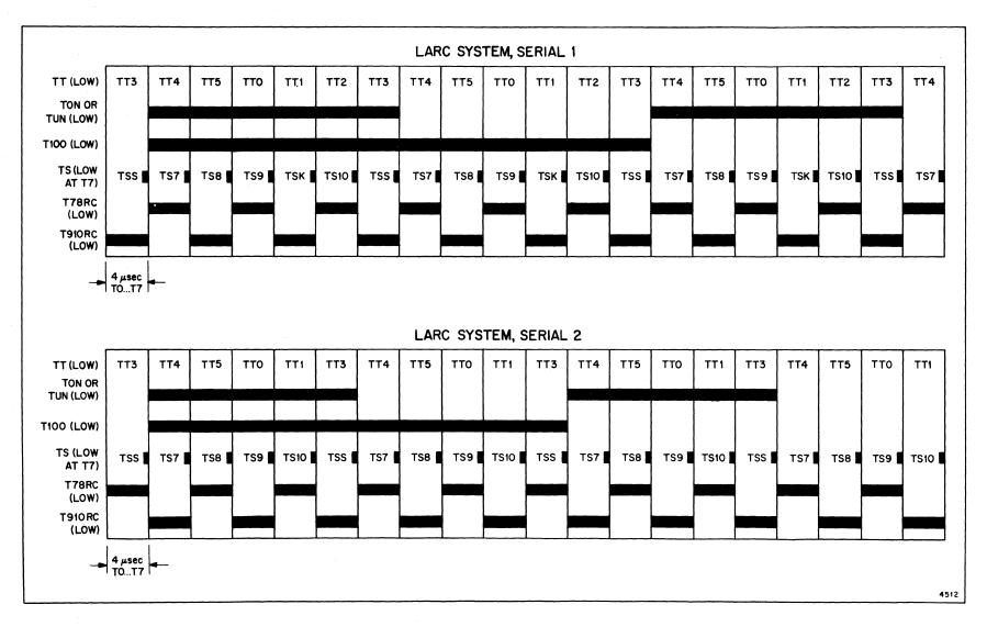
Figure 3-4. Tape Timing Signal Generator Outputs (Larc System, Serials 1 and 2)
