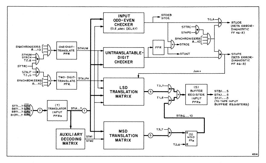
Figure 3-6. Univac-to-Larc Translator and Input Checker (D 807 853...855)
