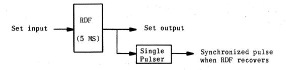
A single pulser following an RDF produces a synchronized output pulse when the RDF recovers.
