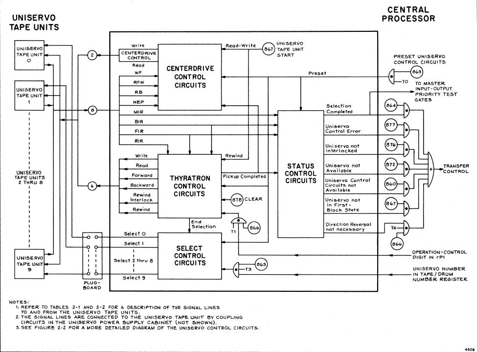
Figure 2-1. Uniservo Control Circuits, Block Diagram
