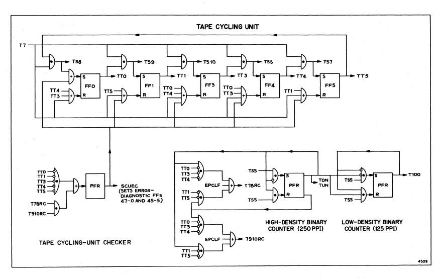
Figure 3-3. Tape Timing Signal Generator in Larc System, Serial 2 (D807 950)
