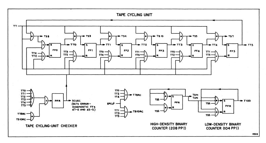
Figure 3-2. Tape Timing Signal Generator in Larc System, Serial 1 (D807 850)
