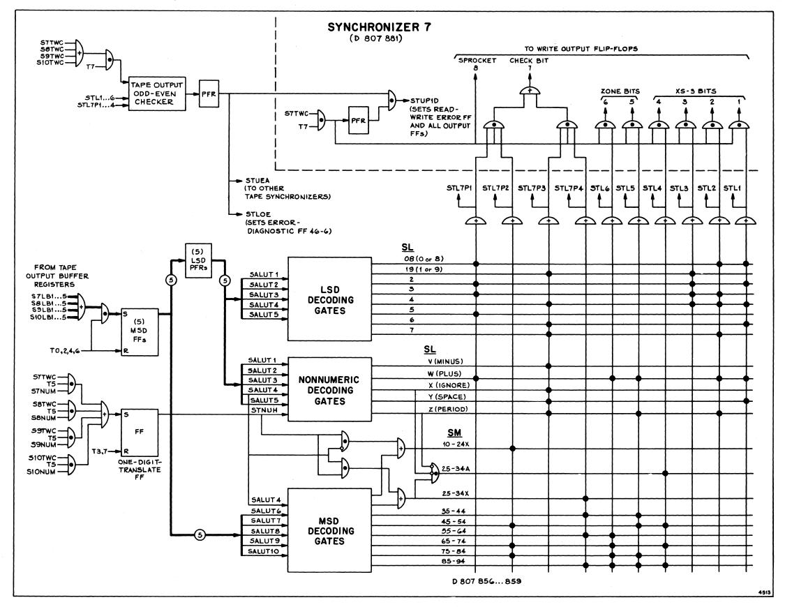
Figure 3-5. Larc-to-Univac Translator and Output Checker and the MSD is read out 1  $\mu$ sec later, at T6. Since both digits of a twodigit combination must be translated simultaneously, the LSD must be delayed to await the arrival of the MSD before being translated.
