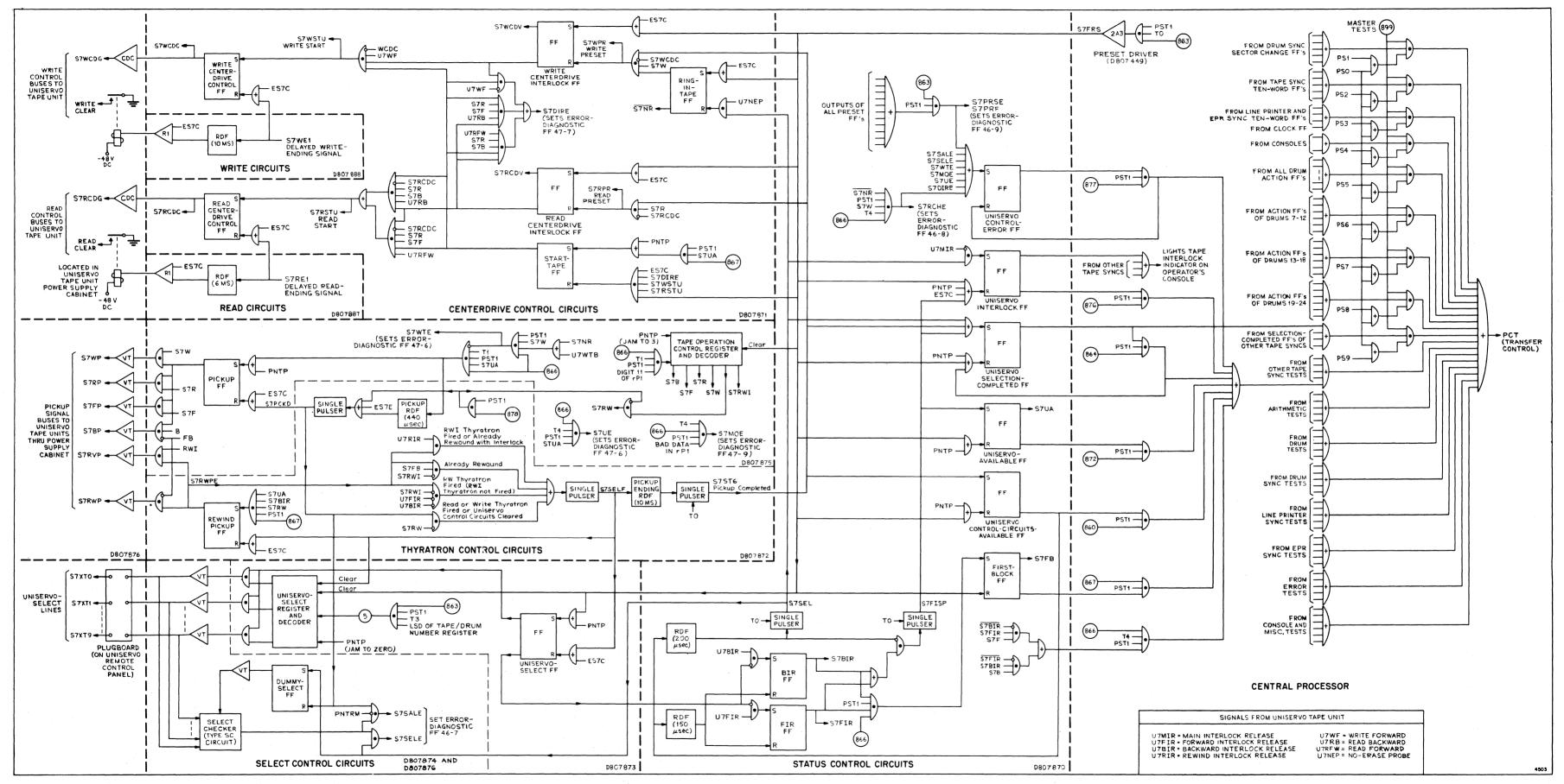
Figure 2-2. Uniservo Control Circuits, Simplified Logic Diagram
