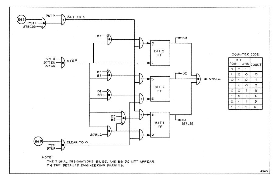
Figure 6-3. Univac Blockette Counter (D 807 888)
