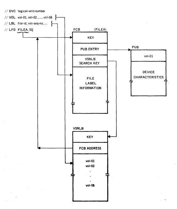
Figure 3--3. Examples of Control Block File Linkage (Part 1 of 2)
