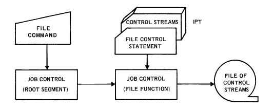
Figure 2-1. Job Entry in a Tape Operating System
