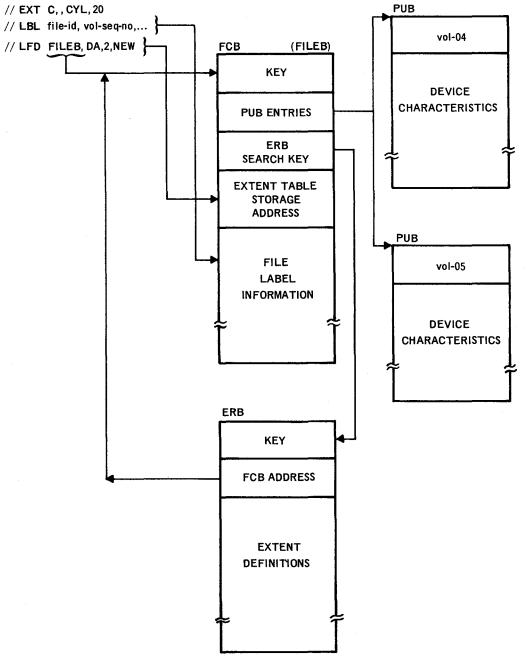
Figure 3-3. Examples of Control Block File Linkage (Part 2 of 2)
