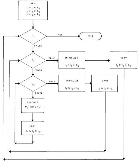
Figure 6-2. PERFORM Logic: Varying Three Identifiers
