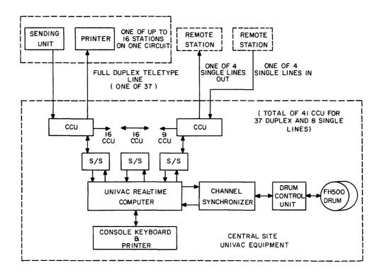
Figure 1. Univac 490 System Layout for Message Switching
