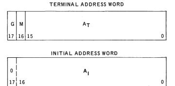
$A_T$ : The address of the last word in the buffer, less the high order address bit
