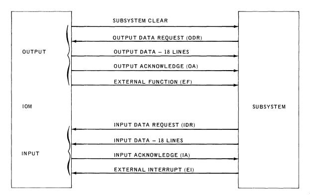
Figure 4–1. One I/O Channel
