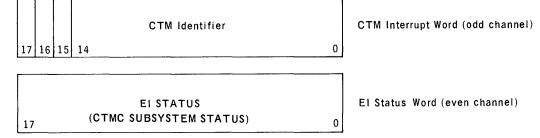
Bits 0-14 of the interrupt word contain the CTM identifier presented to the IOM by the CTM. Bit 15 is a one if the ESI BCW's are stored in the upper 65K of main storage. Bit 16 is a zero.
