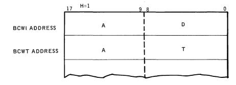
Upon the transfer of each character, the H bit is complemented by the hardware. If the transmission is from 1 to 0, the BCW address is modified as indicated by the G bit in the BCWT. Data transfers may begin on either halfword but must end on a fullword boundary with H = 0.
