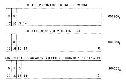
A normal update of BCWI occurs when buffer termination is detected. The final address value stored at the BCWI location for the foregoing example is:
