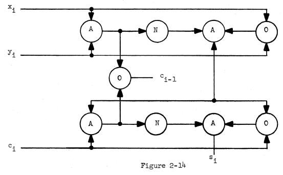
Logical Diagram for One Digital Position of a Binary Adder
