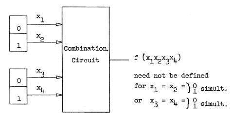
Figure 3-18 Don't Care Condition Circuit
