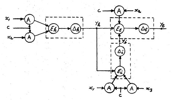
Figure 6-6 Synchronous Equivalent of the Subsection in Figure 6-5
