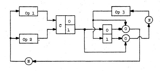
Figure 2-32 Circuit for Interlaced Sequencing
