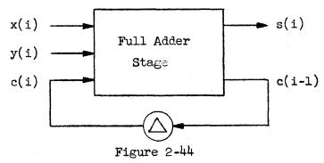
Serial Adder. All pulse trains are injected with the least significant digit first.
