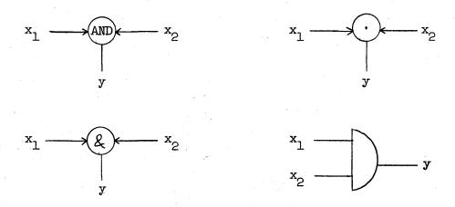
The generalization to multi-input AND's is evident.
