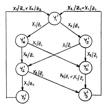
Figure 6-19 Reduced Machine Equivalent to That in Figure 6-18
