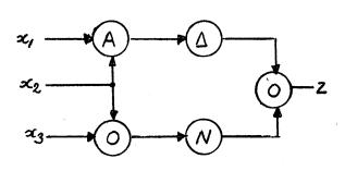
last section we choose a delay  $\Delta$  in the upper path such that  $\Delta \gg \hat{\circ}_{NOT}$ . This will certainly eliminate the transient in the 1,1,0  $\rightarrow$  1,6,0  $\rightarrow$  1,0,0 input transition. Unhappily this very modification now introduces a transient in the 1,0,0  $\rightarrow$  1,6,0  $\rightarrow$  1,1,0 input transition (all other input transitions are safe!).
