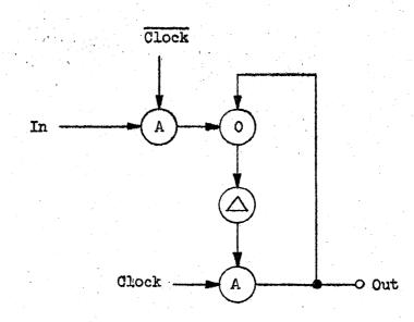
Figure 2-39 Latch Circuit
