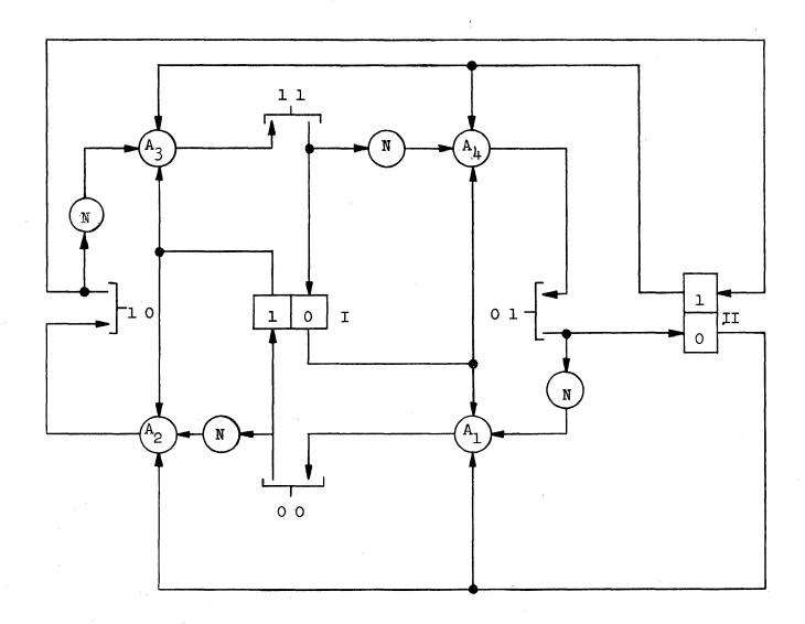
Figure 2-16 Four Step Sequencing Circuit
