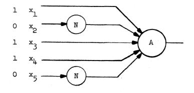
Figure 2-17 Decoder for a 10110 Combination
