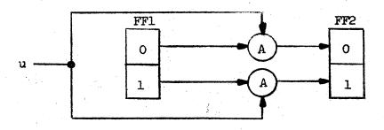
Figure 2-8 Double Gating -27When u is made a "l" (gates enabled), the AND circuit connected to the output of the left flipflop which is "l" will apply this to the corresponding input of the right flipflop. When u goes back to "0", the right flipflop stays set.
