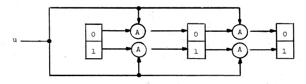
Figure 2-10 Shifting with a Single Register
