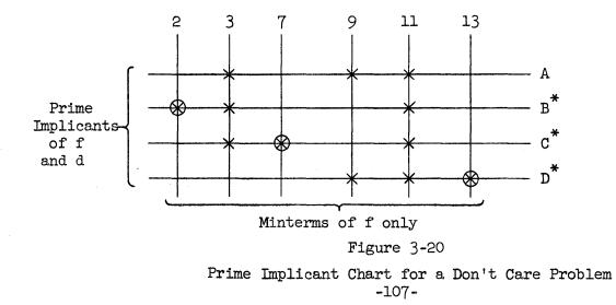
the function can be formed by taking B, C and D only i.e.
