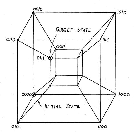
Figure 6-30 States Surrounding State (0,0,0,0) with Target State (0,1,1,1)
