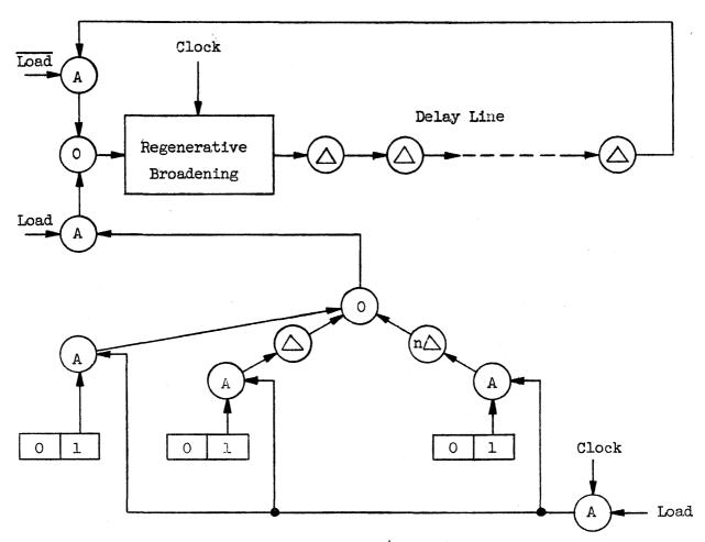
Figure 2-41 Loading of a Line from a Flipflop Register
