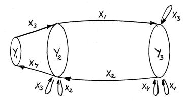
Figure 6-8 State Diagram for a Simple-minded Animal
