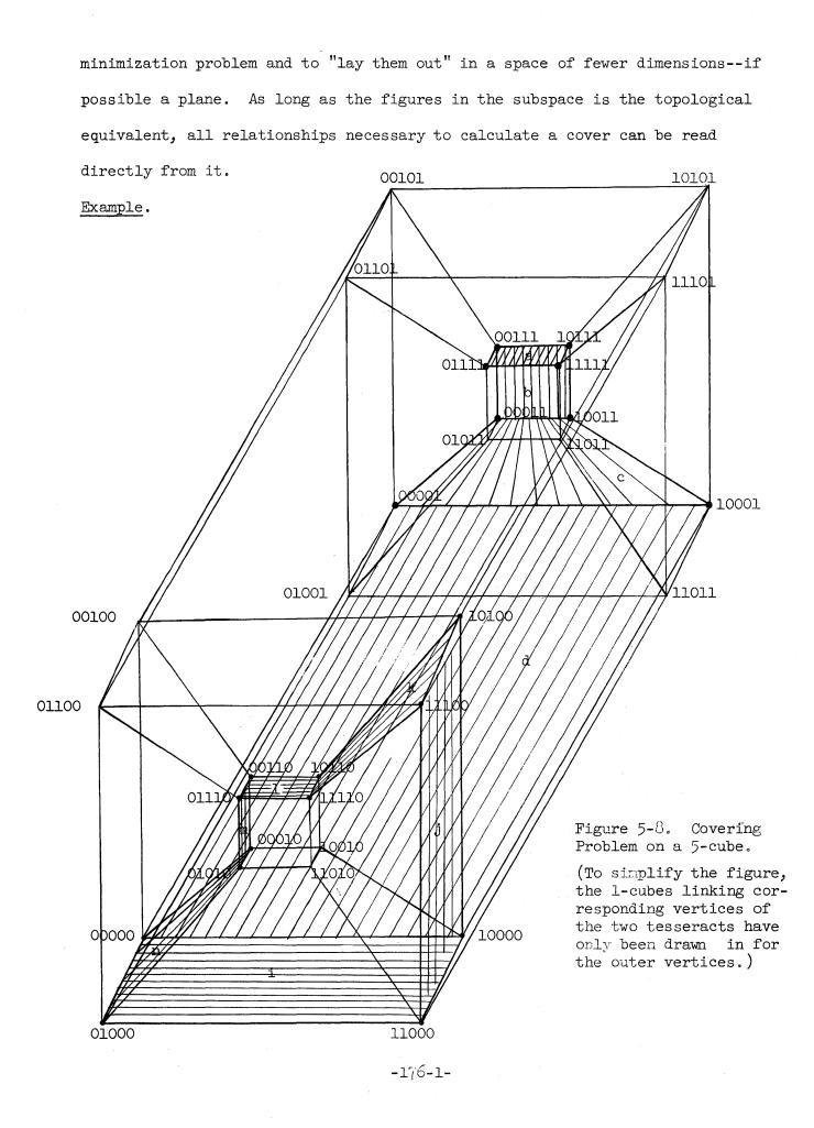
The complex indicate on the 5-cube in Fig. 5-8 is topologically equivalent to the one illustrated in Fig. 5-9. The squares denoted by a, b, c, d, i, j, k, l, m, n are all cocycles.
