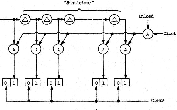
Figure 2-42 Unloading a Staticizer into a Flipflop Register
