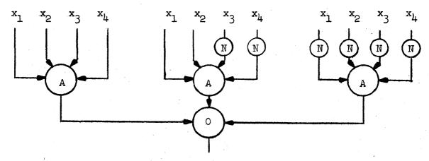
Figure 2-18 Circuit Detecting Several Input Combinations
