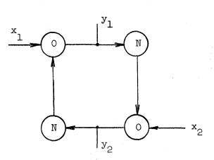
and  $x_2$  are both zero, this circuit still can exist in two "states": either  $y_1 = 1$ ,  $y_2 = 0$  or  $y_1 = 0$  and  $y_2 = 1$ . Which one is "held" depends on which x was last made a one.
