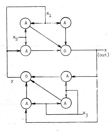
Figure 5-18 Combinational Circuit with Feedback simply apply  $x_3$  to two inputs of the lower majority element and it is evident that its output y simply follows  $x_3$  quite independently of the feedback from z. But this does not contradict the fact that we have a perfectly good feedback circuit.
