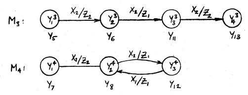
Figure 6-26 Partial State Diagrams
