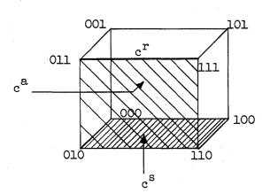
Let  $c^{r}$  and  $c^{s}$  be the cubes  $c^{r} = (xll)$   $c^{s} = (xx0)$ shown in Fig. 5-3. Then  $c^{r} * c^{s} = (xlx) = c^{a}$ , where  $c^{a}$  is also shown in the figure.
