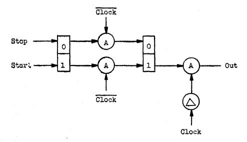
Figure 2-46 Stopping and Starting a Pulse Sequence
