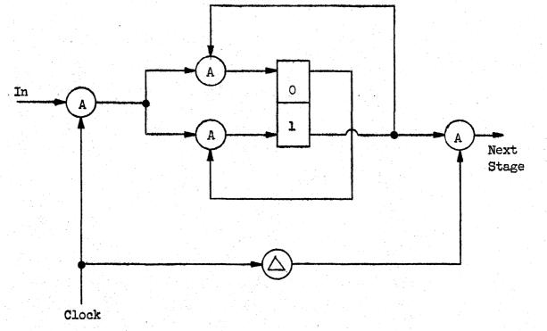
Figure 2-45 One Stage of a Synchronous Counter
