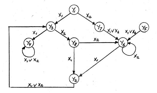
Figure 6-10b Encoded State Diagram
