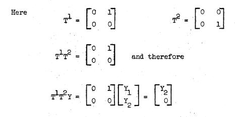
meaning that if we start in state  $Y_1$ , input sequence  $X_1X_2$  leads us to state  $Y_2$ , while if we start in  $Y_2$  the result is unspecified.
