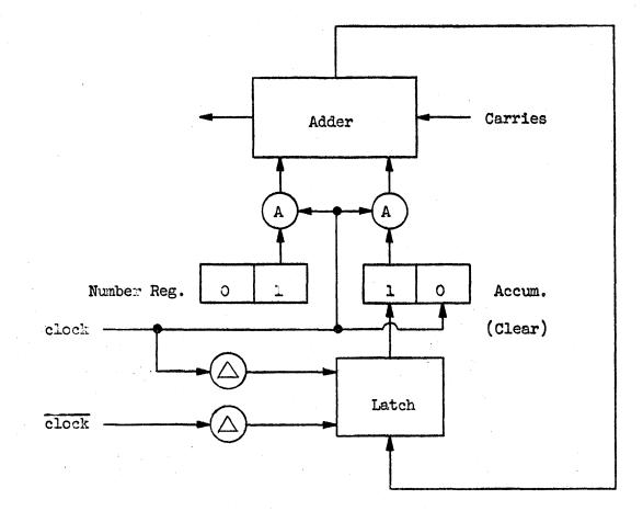
Figure 2-40 One Clock Period Adder Using a Latch
