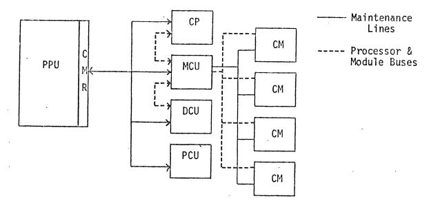
The CMR commands action to be taken, transfer of data directly to or from the unit addressed, or between Central Memory and the addressed unit, using dedicated pointers contained in low order CM. The appropriate status registers, section control cells, decode circuitry, and hard core circuits are contained in each of the addressed units. These circuits are tailored to the needs of the unit in which they reside and interface in a standard way with the CMR.
