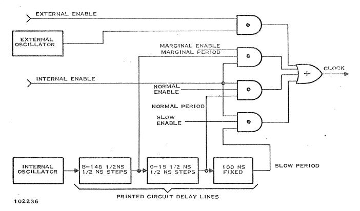
Logic Clock Module Block Diagram
