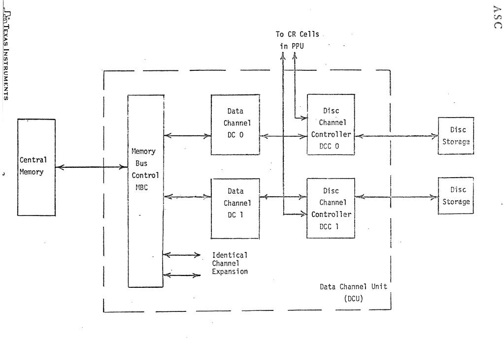
Figure 1. Data Channel Unit Block Diagram
