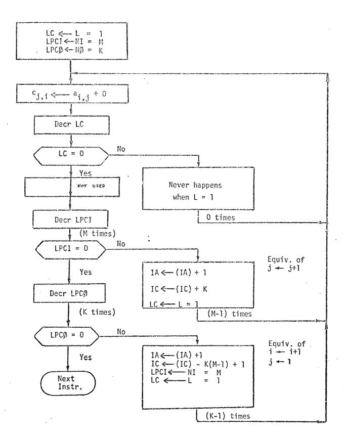
Figure 4. Flow chart for matrix transposition.
