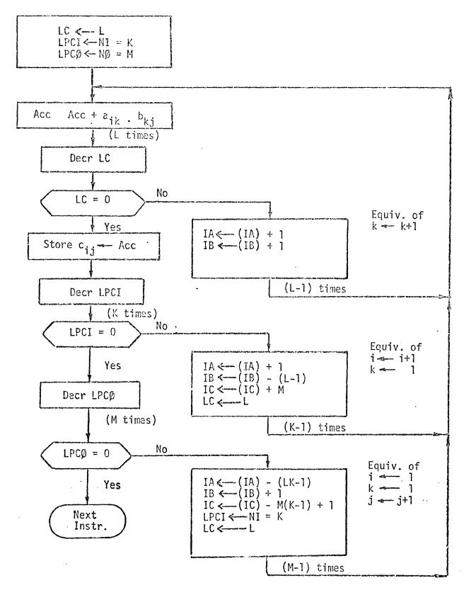
Figure 3. Flow chart for matrix multiplication in which the result is generated by columns instead of by rows as in example B
