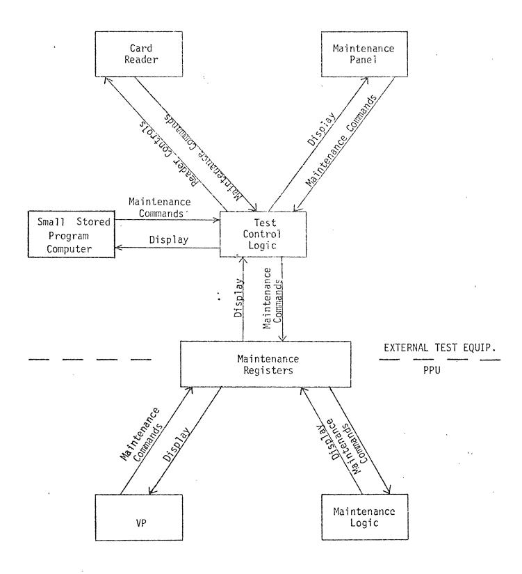
Figure 1. PPU Maintenance Hardware
