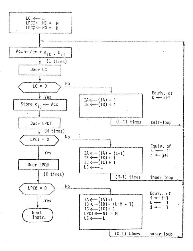
Figure 2. Flow chart for matrix multiplication of example A
