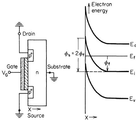
**Fig. 1.36.** MOSFET configuration with  $V_G$  negative and MOSFET energy-level diagram with  $V_G$  negative,  $Q_{SS} = 0$ ,  $Q_{Ox} = 0$ , and  $\Phi_{MS} = 0$ . The channel is inverted.
