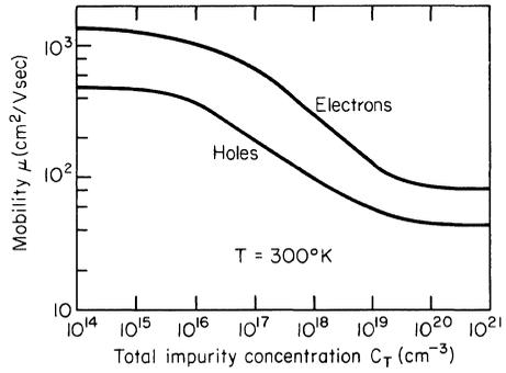
**Fig. 1.16.** Majority-carrier mobility values as a function of impurity concentration.<sup>7</sup>  $T = 300^\circ\text{K}$ .
