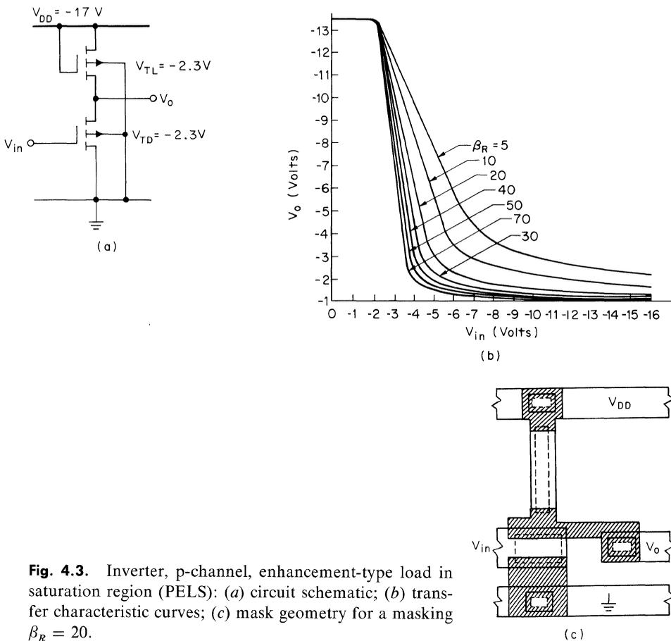
Fig. 4.3. Inverter, p-channel, enhancement-type load in saturation region (PELS): (a) circuit schematic; (b) transfer characteristic curves; (c) mask geometry for a masking  $\beta_R = 20$ .
