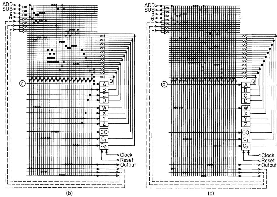
**Fig. 8.19.** Bit-serial adder/subtractor using PLA format (4-bits). (a) Functional logic net; (b) PLA implementation with *D*-type flip-flops only; (c) PLA implementation with shift registers substituted in the feedback circuit.
