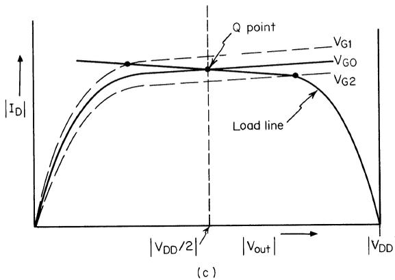
**Fig. 9.6.** (a) Discrete version of the enhancement-mode driver—depletion-mode load configuration; (b) integrated circuit version of the enhancement-mode driver—depletion-mode load configuration; (c) intersection of depletion-mode load line with driver device characteristics.
