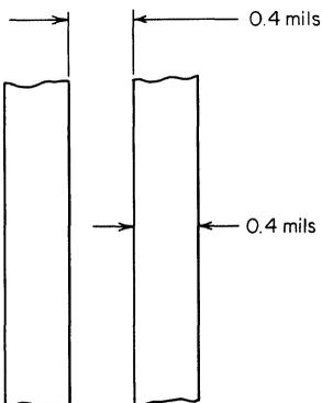
Fig. 3.13. Metal width and metal spacing.
