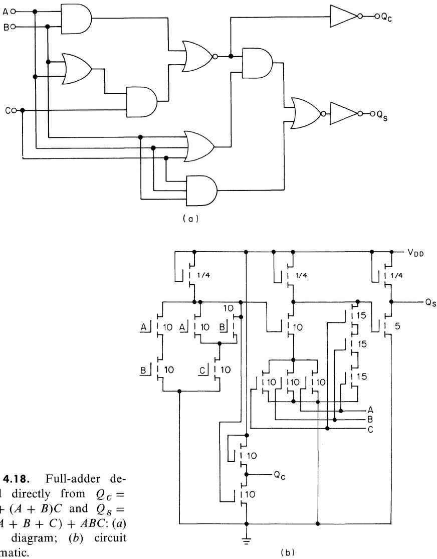
**Fig. 4.18.** Full-adder derived directly from  $Q_c = AB + (A + B)C$  and  $Q_s = Q_c(A + B + C) + ABC$ : (a) logic diagram; (b) circuit schematic.
