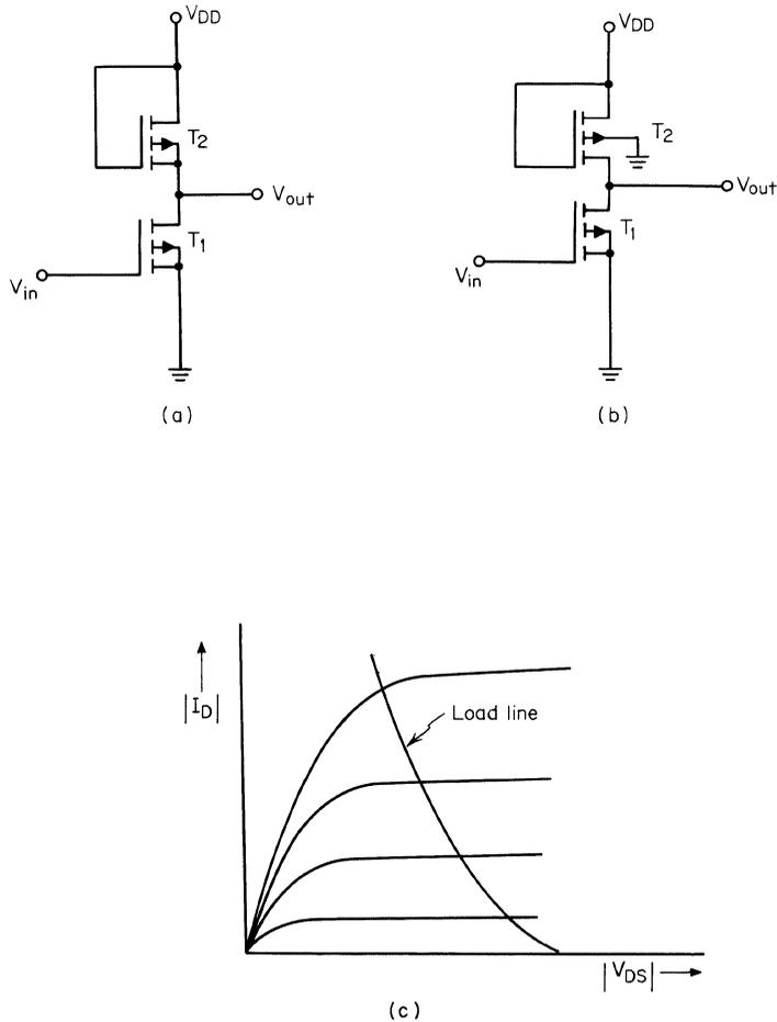
**Fig. 9.5.** (a) Discrete version of the enhancement-mode driver—enhancement-mode load configuration; (b) integrated circuit version of the enhancement-mode driver—enhancement-mode load configuration; (c) intersection of enhancement-mode MOSFET load line with driver device characteristics.
