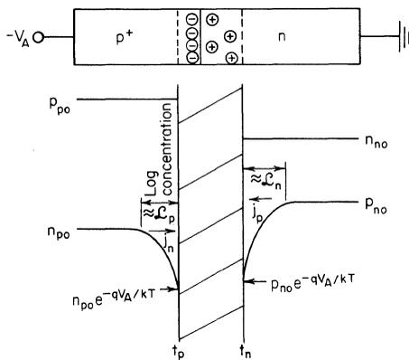
Fig. 1.26. Carrier concentration for the reverse-biased p-n junction.
