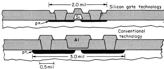
Fig. 2.6. Silicon gate versus aluminum gate structure.<sup>3</sup>
