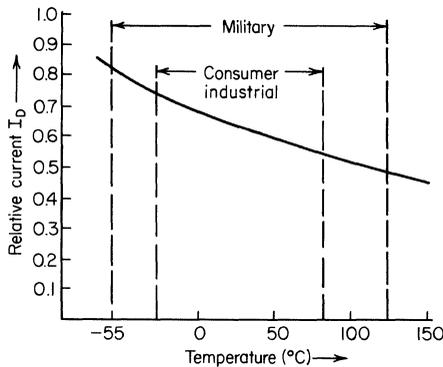
Fig. 3.4. Drain current as a function of temperature.
