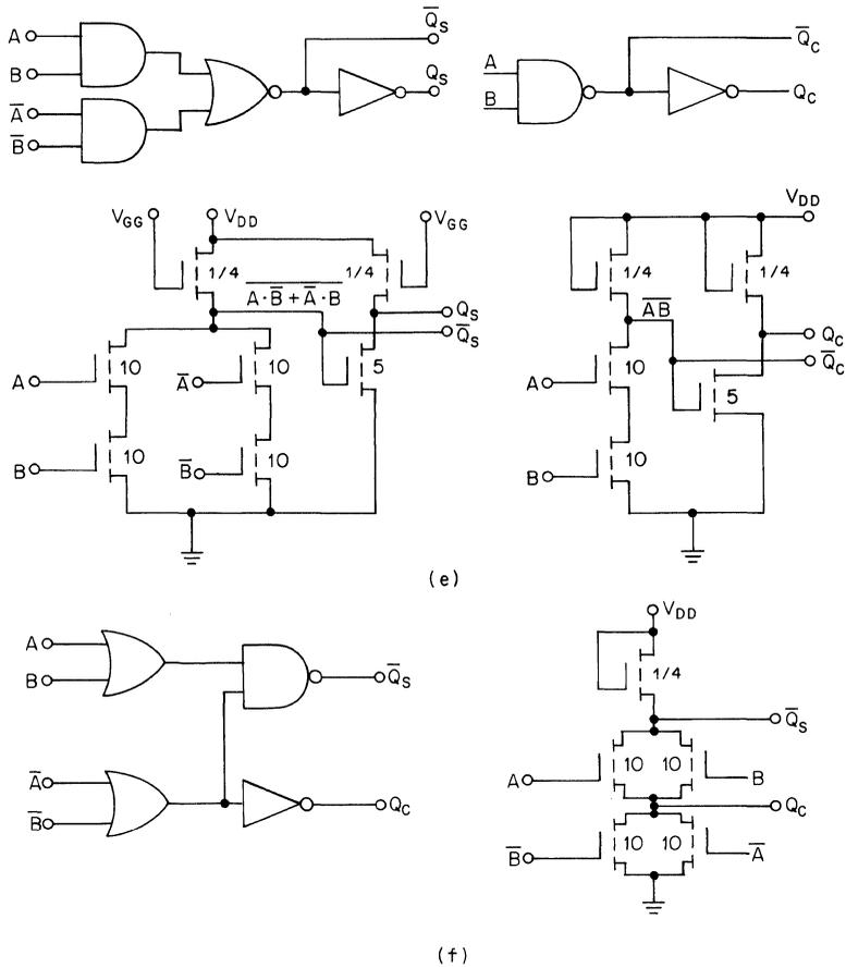
**Fig. 4.14.** Half-adder circuitry showing negative-logic equivalents; (a) all NOR gates; (b) all NOR gates with complemented logic inputs only; (c) all true levels with 16 devices; (d) all true levels with 11 devices; (e) both complemented and true logic levels available at the output; (f) low-device-count design.
