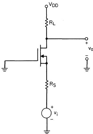
Fig. 9.23. Common-gate MOSFET configuration.
