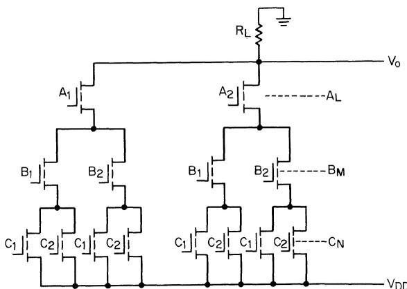
**Fig. 7.10.** Unconventional ROM circuit with a tree structure.
