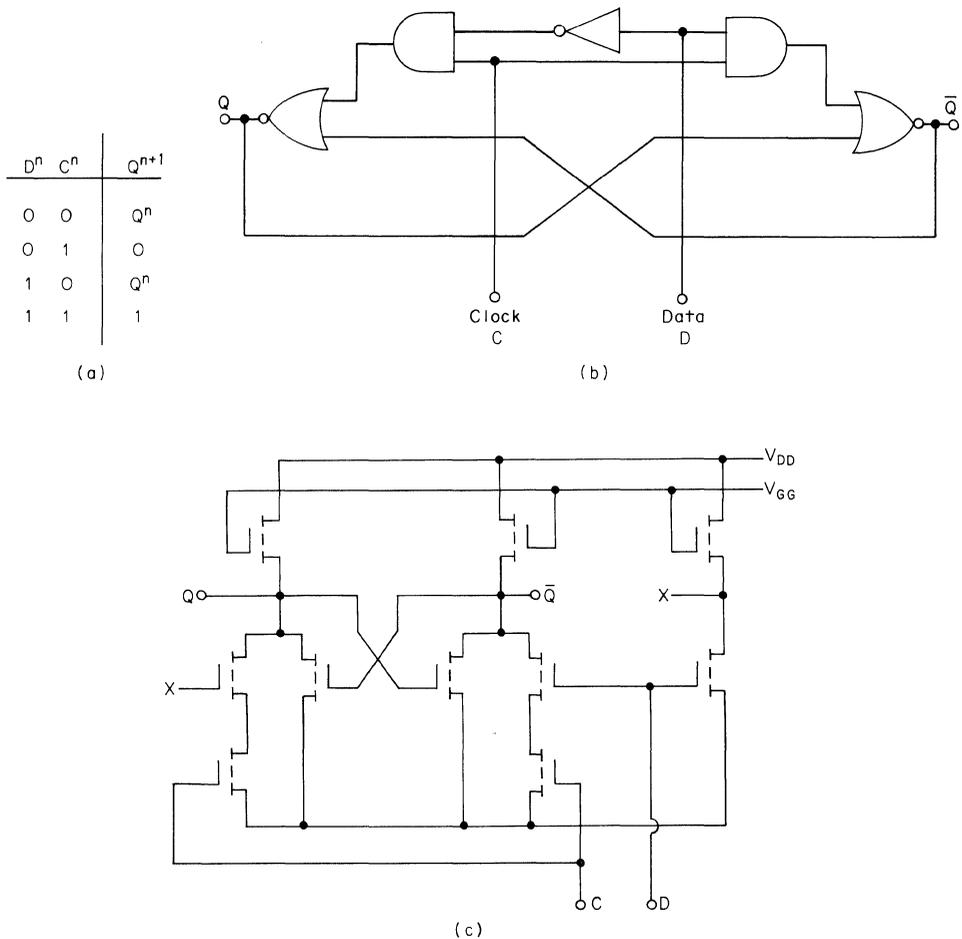
**Fig. 4.20.** Static logic latch: (a) truth table; (b) logic diagram; (c) PEELS circuit schematic.
