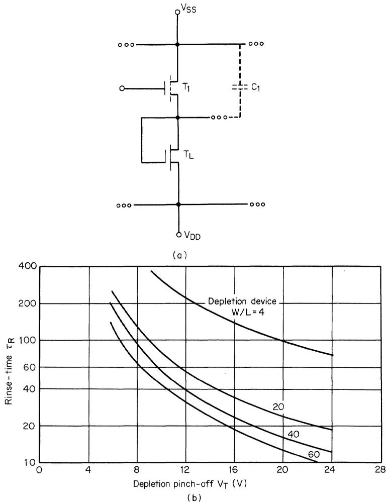
**Fig. 6.4.** Increased drive capability with low-impedance PDLT inverter: (a) circuit schematic; (b) rise-time  $t_R$  vs. threshold (pinch-off) voltage of the load device with  $W/L$  ratio of the depletion device as a parameter and  $C_1 = 0.5$  pF.
