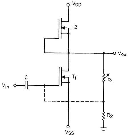
**Fig. 9.8.**  $Q$  point adjustment with negative feedback.
