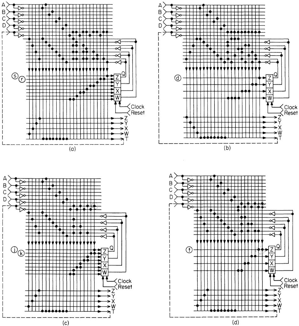
**Fig. 8.17.** Improved 4-bit, variable-modulo counter with reset-to-zero and feedback  $\bar{T}$ . (a) *S-R*-type flip-flops; (b) *D*-type flip-flops; (c) *J-K*-type flip-flops; (d) *T*-type flip-flops.
