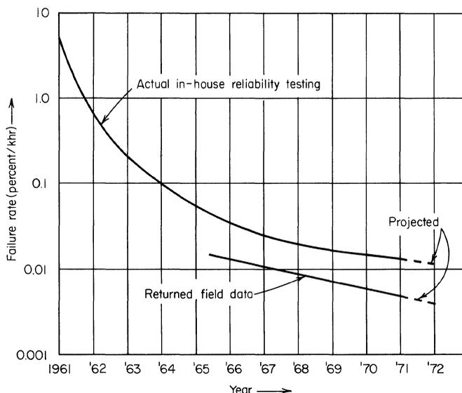
**Fig. 3.23.** Texas Instruments' bipolar integrated circuit failure-rate history.
