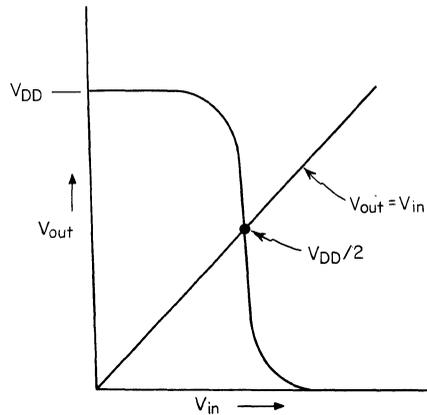
**Fig. 9.11.** Transfer characteristics of the complementary MOSFET configuration.
