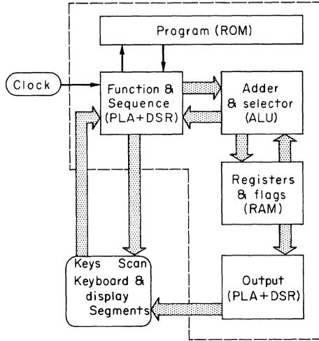
Fig. 10.19. Block diagram of the 1971 MOS calculator.
