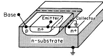
Fig. 2.10. Emitter-follower bipolar transistor on MOS chip.
