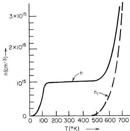
Fig. 1.10. Temperature dependence of electron concentration in n-type silicon.<sup>5</sup>
