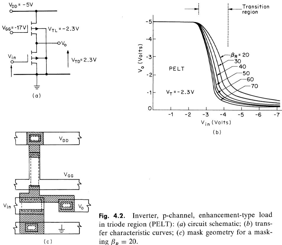
**Fig. 4.2.** Inverter, p-channel, enhancement-type load in triode region (PELT): (a) circuit schematic; (b) transfer characteristic curves; (c) mask geometry for a masking  $\beta_R = 20$ .
