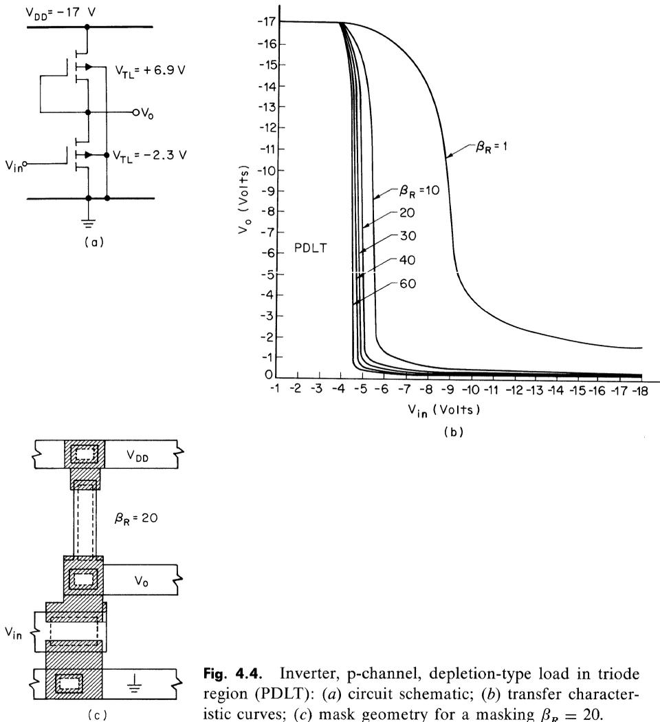
**Fig. 4.4.** Inverter, p-channel, depletion-type load in triode region (PDLT): (a) circuit schematic; (b) transfer characteristic curves; (c) mask geometry for a masking  $\beta_R = 20$ .
