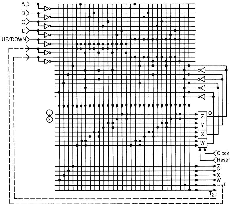
Fig. 8.18. Four-bit up/down, variable-modulo counter using PLA array.
