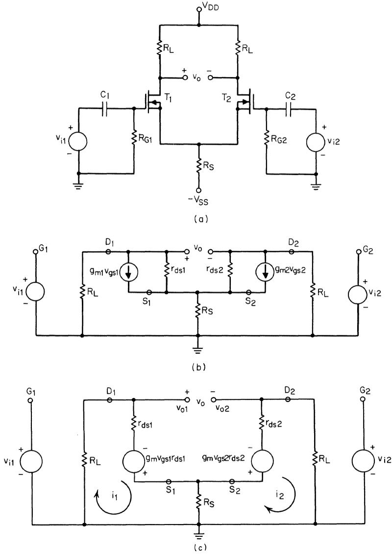
**Fig. 9.31.** (a) MOSFET differential amplifier; (b) small-signal equivalent circuit for MOSFET differential amplifier; (c) transformed small-signal equivalent circuit for MOSFET differential amplifier.
