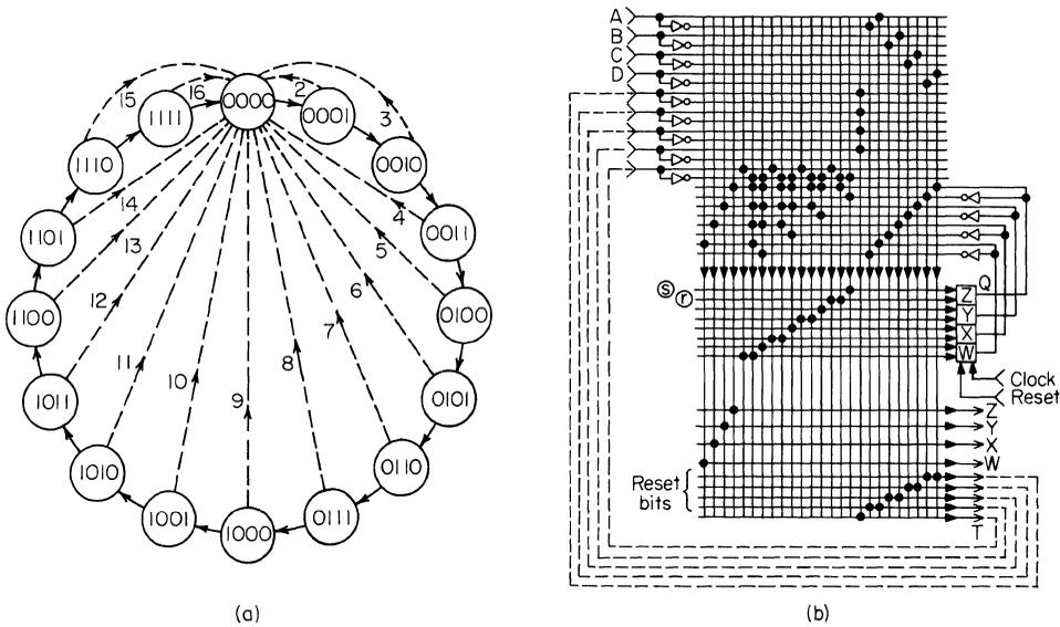
**Fig. 8.16.** Four-bit, variable-modulo counter with reset-to-zero and count-out determined by input control bits and feedback  $T$ . (a) Transition sequence; (b)  $S$ - $R$ -type flip-flops.
