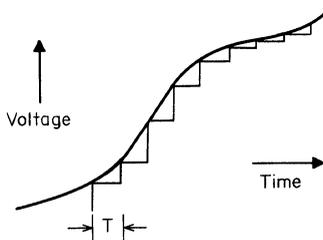
**Fig. 9.32.** (a) Idealized electronic delay line<sup>18</sup>; (b) voltage versus time at the input and output of first section of the electronic delay line.<sup>18</sup>
