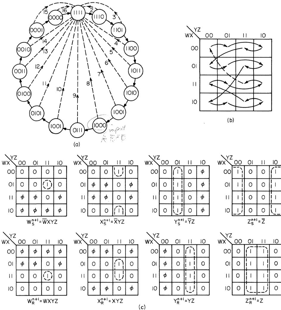
**Fig. 8.14.** Design sequence for a 4-bit, variable-modulo counter. (a) Transition sequence; (b) transition diagram for the modulo-16 counter; (c) multiple, 4-bit Karnaugh maps for modulo-16<sub>10</sub> and R-S-type flip-flops.
