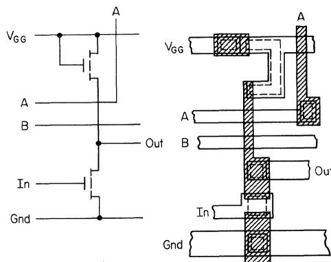
**Fig. 3.5.** Basic inverter circuit. Cross-hatched regions denote p-diffused areas. Dotted lines denote thin-oxide delineation. Solid lines surrounding dotted lines denote thick-oxide delineation. Clear regions denote aluminum lead patterns.
