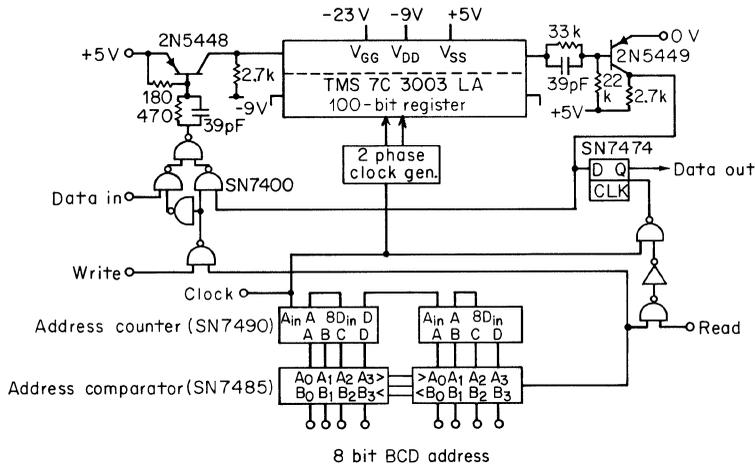
Fig. 5.26. Scratch-pad type memory with bipolar control circuitry.
