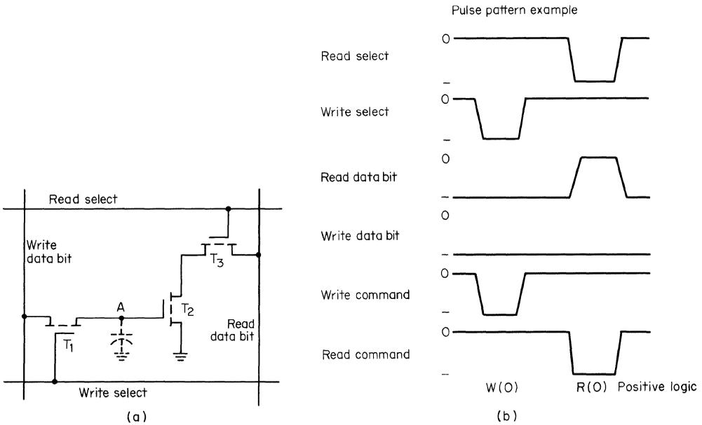
**Fig. 7.15.** Three-transistor dynamic RAM cell: four lines per cell for  $2\phi$ : (a) schematic circuit; (b) pulse pattern example; (c) refresh and data I/O.
