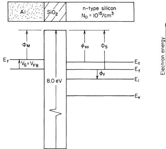
**Fig. 1.40.** Flat-band condition for the aluminum-SiO<sub>2</sub>-silicon system ( $N_D = 10^{15}/\text{cm}^3$ ).
