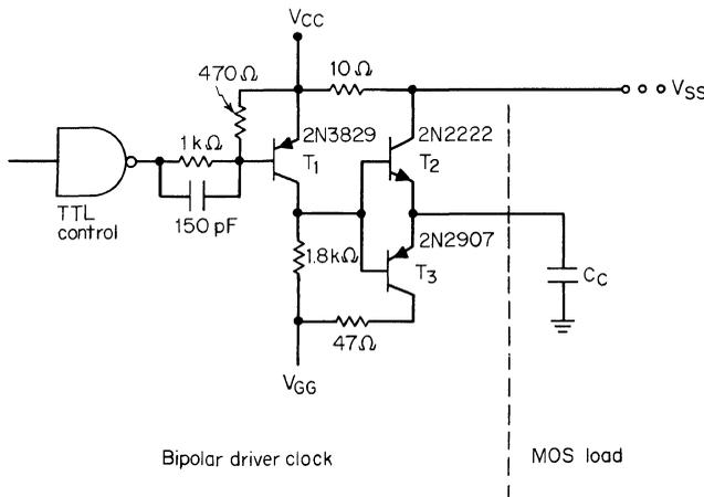
Fig. 6.13. Clock circuit using complementary bipolar transistors.
