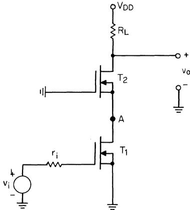
**Fig. 9.27.** The MOSFET cascode configuration (discrete version).
