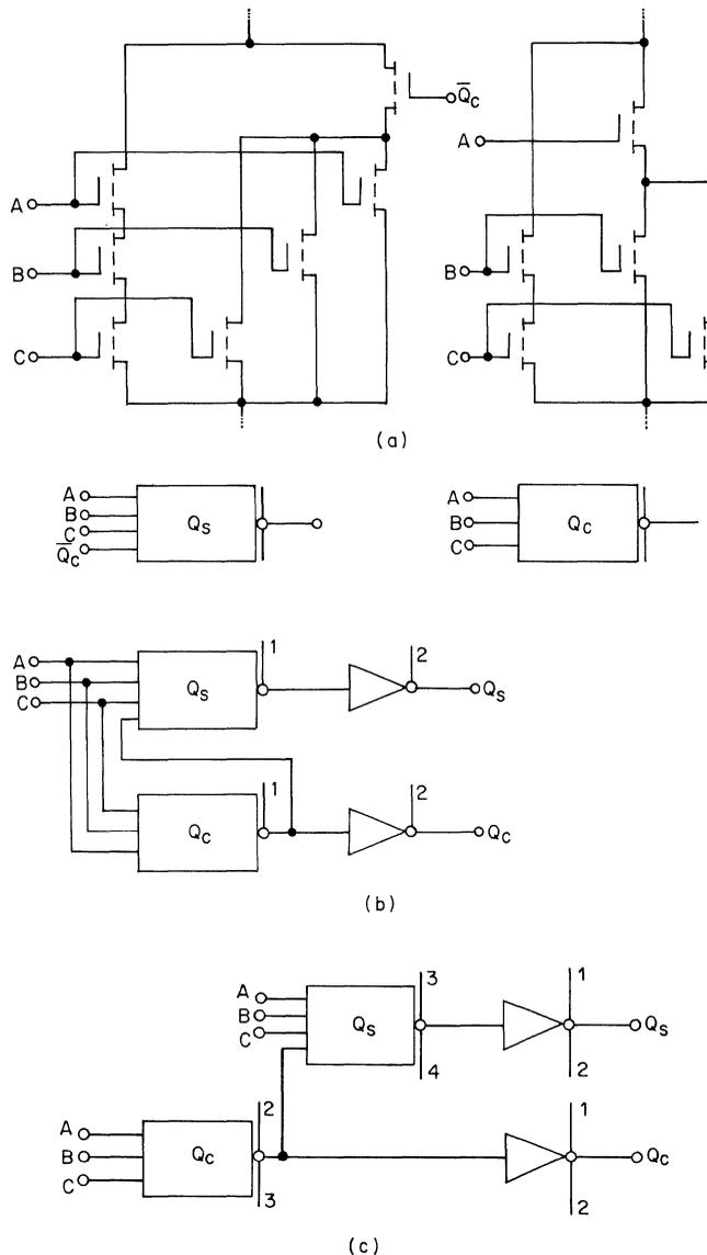
**Fig. 5.23.** Full-adder circuit: (a) sum  $Q_s$  and carry  $Q_c$  logic net for multiphase circuit implementation; (b) typical two-phase type II logic net; (c) typical four-phase logic net.
