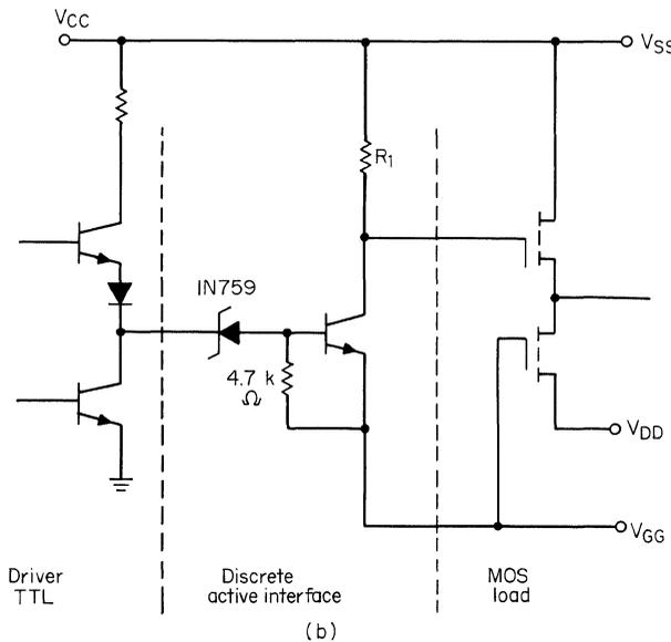
**Fig. 6.6.** Interface circuitry with increased logic swing for driving MOS circuitry from a bipolar driver. MOS substrate is at a voltage  $V_{CC}$  level: (a) inverter with base-limiting resistor; (b) inverter with Zener voltage translation.
