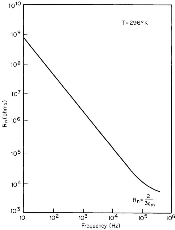
**Fig. 9.14.** Input noise resistance for the MOSFET as a function of frequency (p-channel device).<sup>10</sup>
