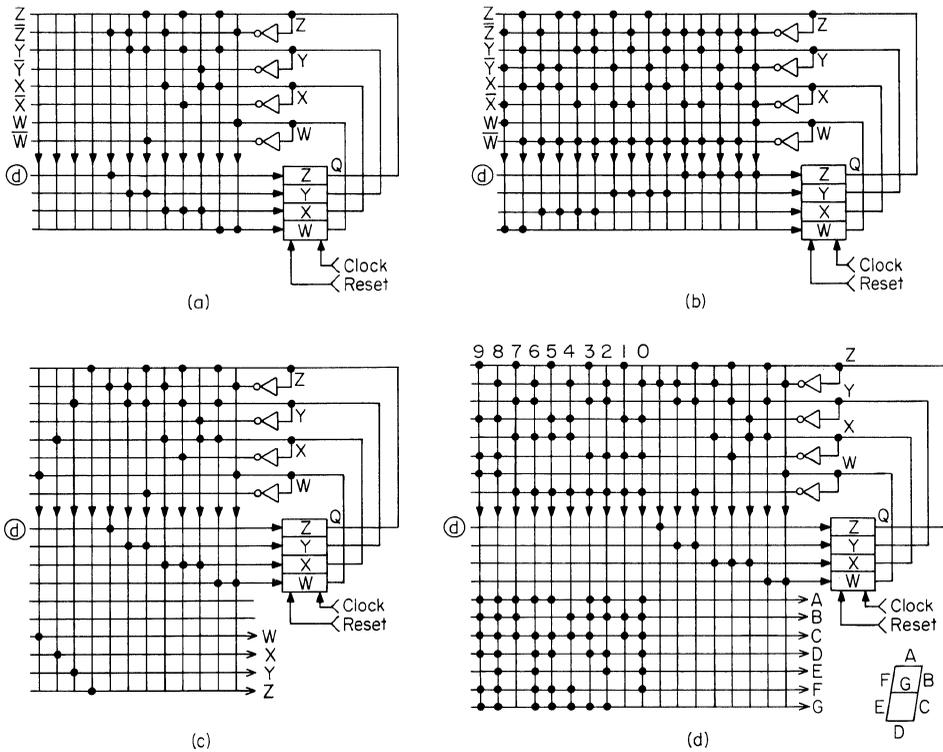
**Fig. 8.8.** PLA-logic schematic for modulo-10 counter using *D*-type flip-flops. (a) PLA design using the reduced logic from the Karnaugh maps of Fig. 8.7c; (b) PLA design without benefit of the reduced logic; (c) counter output decoded for binary code; (d) counter output decoded to drive a seven-segment display.
