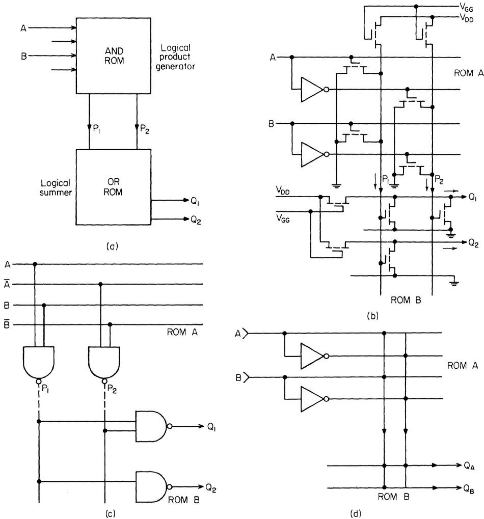
**Fig. 8.3.** Coupled arrays for implementing static logic:  $Q_1 = AB + \bar{A}\bar{B}$  and  $Q_2 = AB$ . (a) Block diagram; (b) circuit schematic; (c) standard-logic schematic; (d) array-logic schematic.
