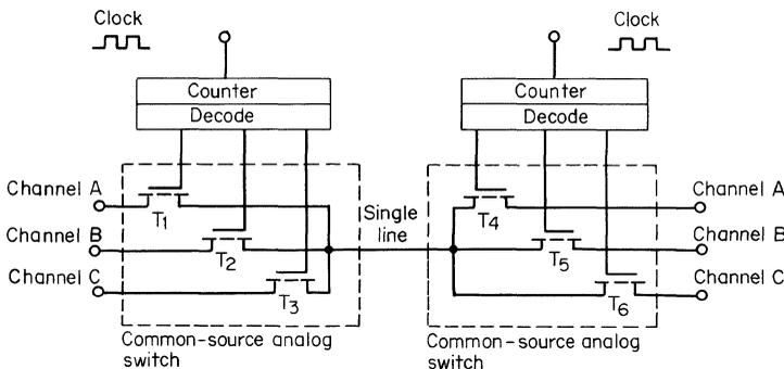
**Fig. 9.41.** Common-source analog switch used for multiplexing.
