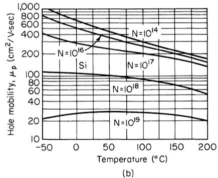
**Fig. 1.17.** Electron and hole mobility values in silicon as a function of temperature for various impurity concentrations.<sup>9</sup>
