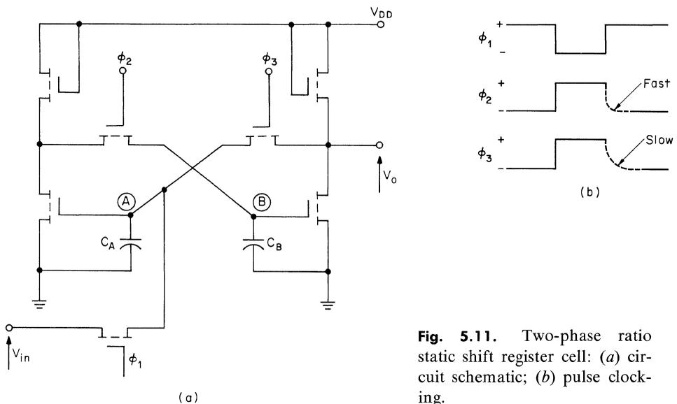
**Fig. 5.11.** Two-phase ratio static shift register cell: (a) circuit schematic; (b) pulse clocking.
