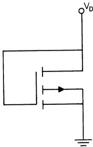
Fig. 1.50. MOSFET with gate connected to drain.
