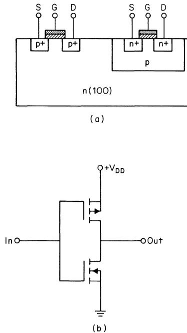
Fig. 2.12. (a) CMOS structure; (b) CMOS cell.
