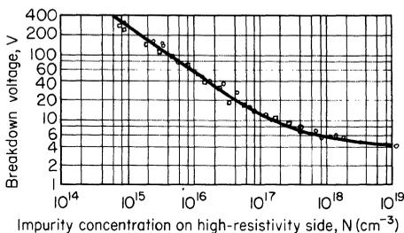
Fig. 1.32. The breakdown voltage of a silicon step junction ( $n^+p$  or  $p^+n$ ) as a function of impurity concentration on the lightly doped side.<sup>20</sup>
