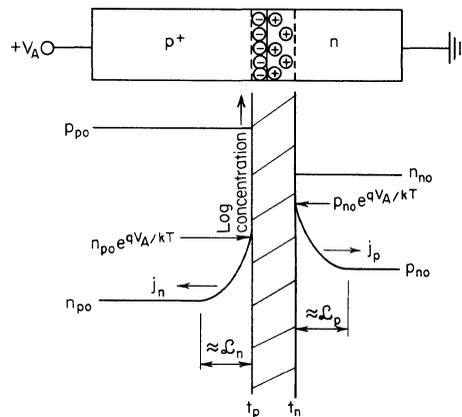
**Fig. 1.24.** Carrier concentration for the forward-biased p-n junction.
