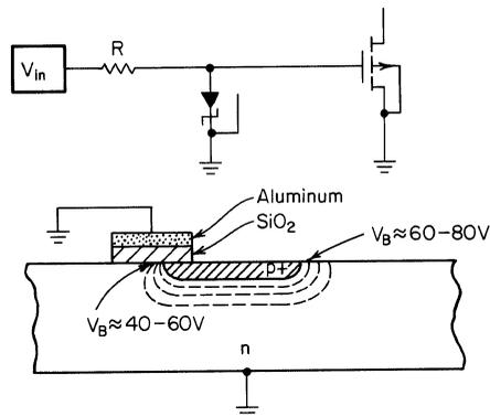
Fig. 3.19. p<sup>+</sup>-n diode and field plate input protection.
