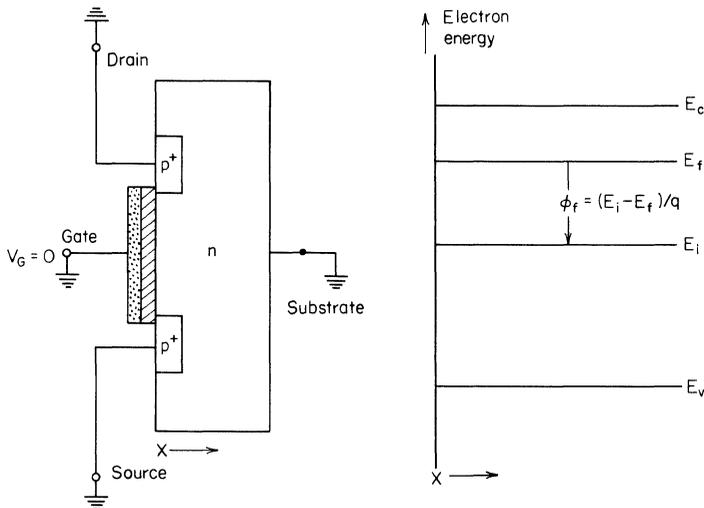
**Fig. 1.35.** MOSFET configuration with gate, source, drain, and substrate at ground potential with accompanying energy-level diagram for device terminals grounded and  $Q_{SS} = 0$ ,  $Q_{ox} = 0$ , and  $\Phi_{MS} = 0$ .
