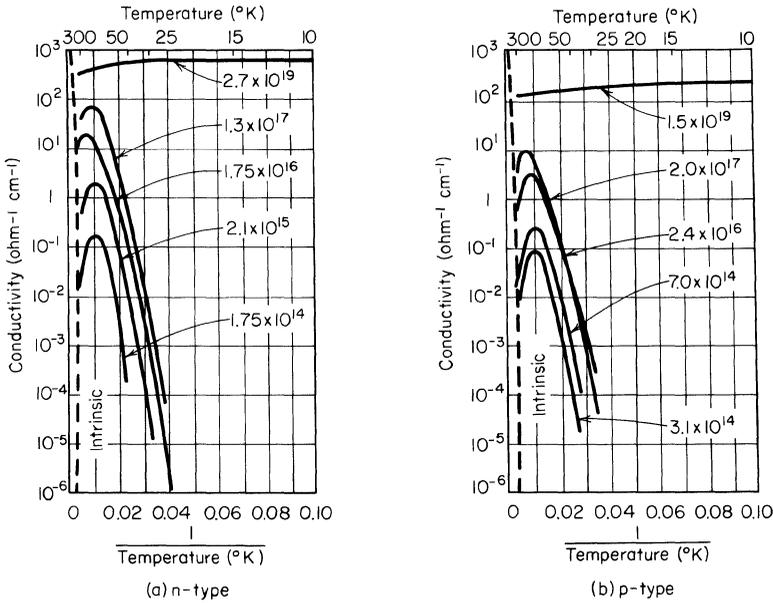
**Fig. 1.19.** Silicon conductivity versus temperature for various impurity concentrations.<sup>10</sup>
