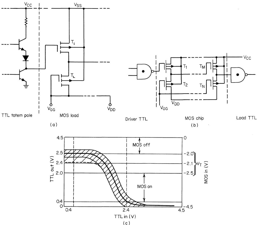
**Fig. 6.1.** Typical bipolar TTL circuits direct-coupled: (a) bipolar TTL driving an MOS PELT inverter; (b) MOS chip showing external TTL circuits connected at input and output; (c) interface transfer characteristics indicating noise-margin problem.
