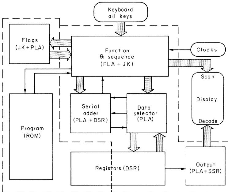
Fig. 10.18. Block diagram of the 1970 MOS calculator.
