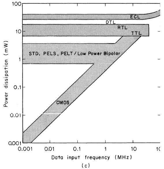
**Fig. 4.9.** Transient response for inverters: (a) lower (driver) device conducting; (b) upper (load) device conducting. The electrical beta ratio  $\beta_R = 20$ , and parameters are given in Tables 4.3 and 4.4; (c) representative power dissipation values for static gates as a function of data input frequency.
