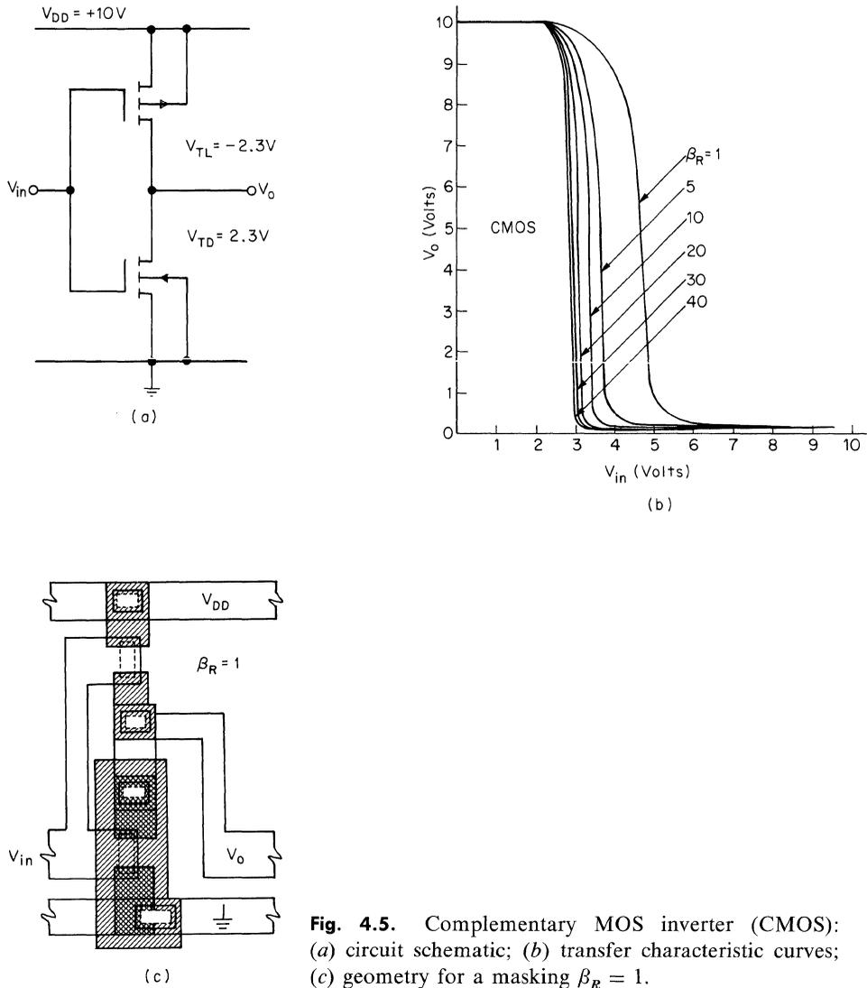
**Fig. 4.5.** Complementary MOS inverter (CMOS): (a) circuit schematic; (b) transfer characteristic curves; (c) geometry for a masking  $\beta_R = 1$ .
