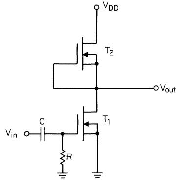
Fig. 9.7. The n-Channel depletion-mode driver—depletion-mode load configuration.
