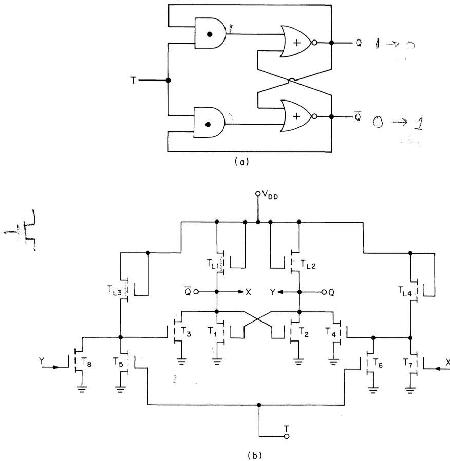
Fig. 4.22. Alternative  $T$ -type static flip-flop circuit: (a) logic diagram; (b) PELS circuit schematic.
