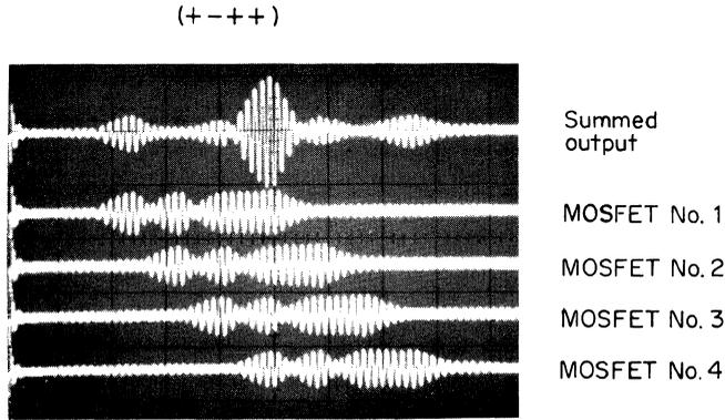
**Fig. 9.36.** Correlation of a 4-bit Barker sequence with MOSFET surface-wave array.<sup>22</sup>
