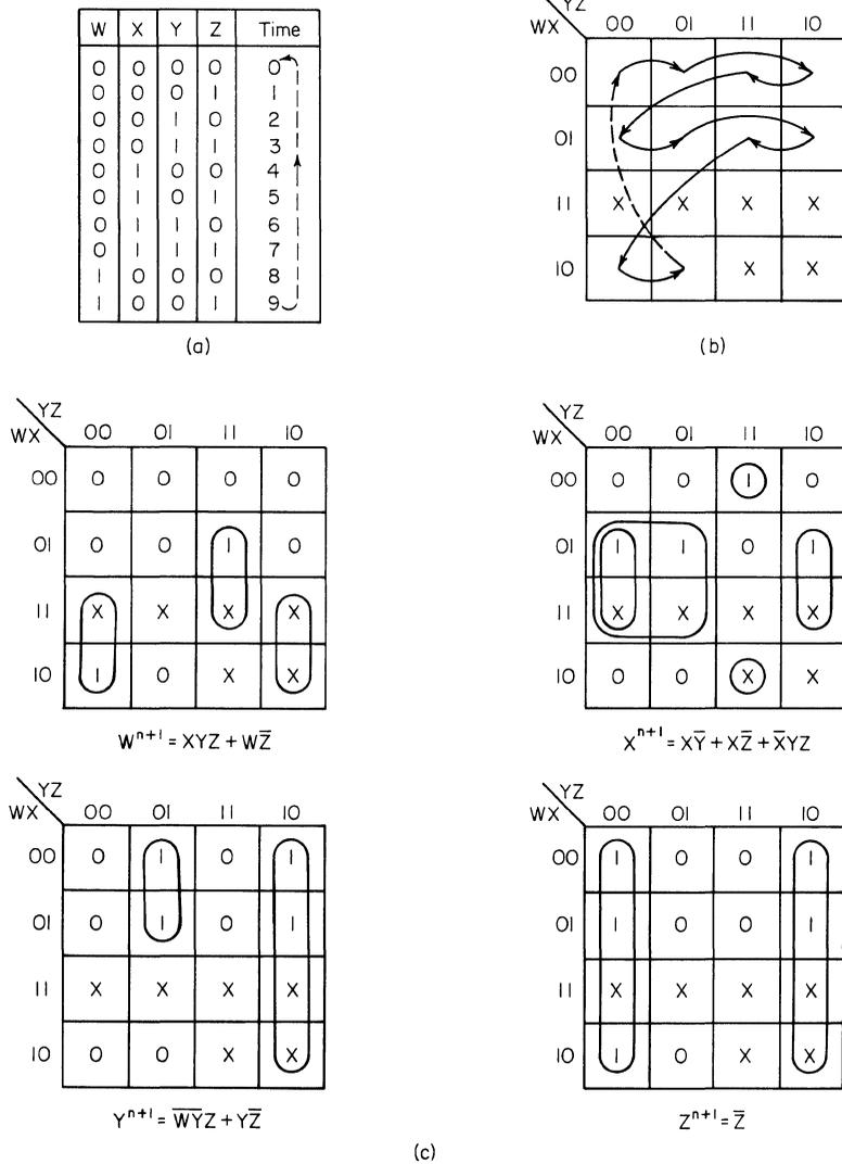
**Fig. 8.7.** Design sequence for a PLA counter of modulo-10 and using *D*-type flip-flops. (a) Transition sequence; (b) transition diagram; (c) multiple, 4-bit Karnaugh maps with logic functions for *D*-type flip-flops.
