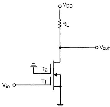
**Fig. 9.15.** MOSFET cascode stage featuring the dual gate.
