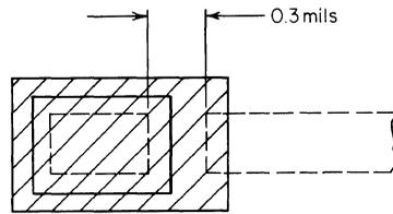
Fig. 3.14. Contact-to-gate separation.
