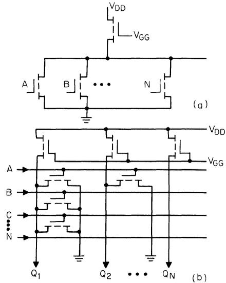
**Fig. 7.4.** ROM matrix provides single-level logic: (a) equivalent column circuit; (b) matrix for implementing negative logic.  $Q_1 = A + B + C$ .
