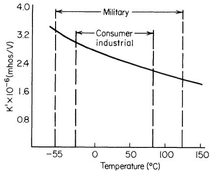
**Fig. 3.3.**  $K'$  as a function of temperature.
