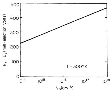
**Fig. 1.12.**  $E_f - E_i$  vs. impurity doping level  $N_D$ .
