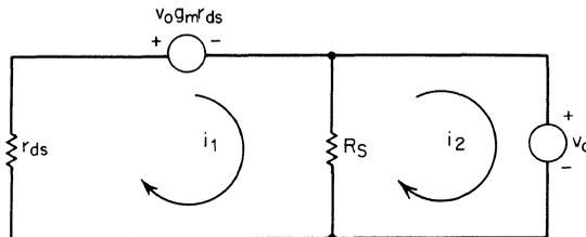
**Fig. 9.22.** Circuit for analysis of the common-drain configuration.
