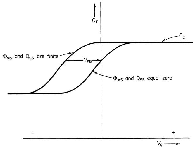
Fig. 1.45. Translation of C-V characteristic through  $V_{FB}$ .
