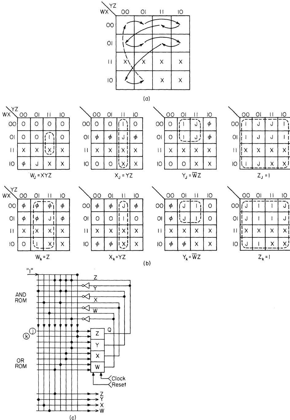
**Fig. 8.10.** Design sequence for a PLA counter of modulo-10 and using a *J-K*-type flip-flop. (a) Transition diagram; (b) 4-bit Karnaugh maps; (c) PLA-logic diagram with decoding for weighted binary output.
