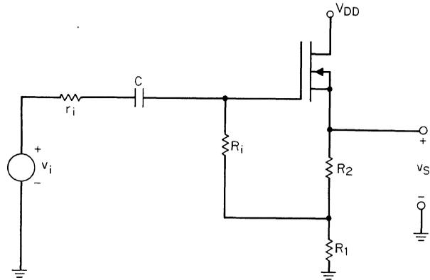
Fig. 9.4. The self-biasing method for the depletion-mode MOSFET.
