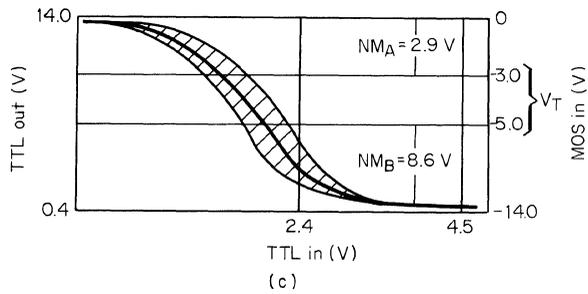
**Fig. 6.5.** Increased logic swing obtained for MOS from a TTL data source using proper selection of  $V_{SS}$  and  $V_{GG}$ : (a) circuit schematic; (b) noise-margin relationship for  $V_{SS} = 8\text{ V}$ ; (c)  $V_{SS} = 14\text{ V}$ .
