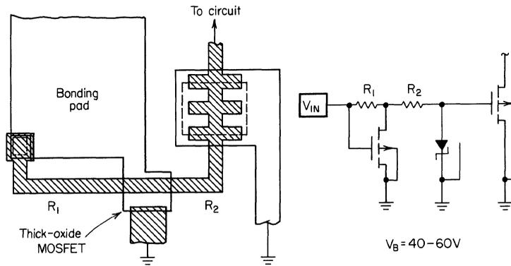
**Fig. 3.20.** p<sup>+</sup>-n diode, field plate and thick-oxide MOSFET input protection.
