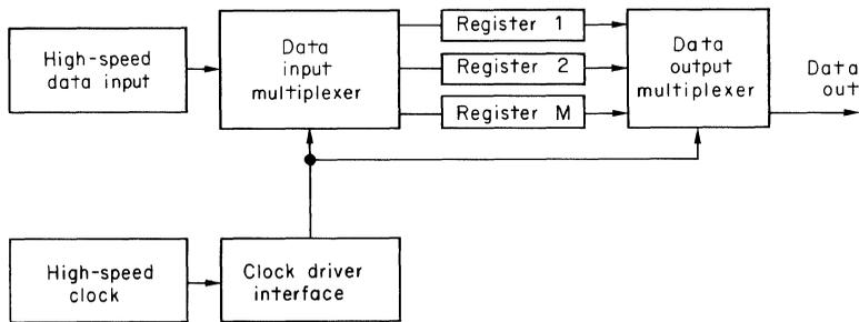
**Fig. 5.15.** High-speed data system.  $M$  separate shift registers, each shifting  $F_0$  bits per second, are used in the multiplexing circuit to obtain an overall data transfer rate of  $MF_0$  bits per second.
