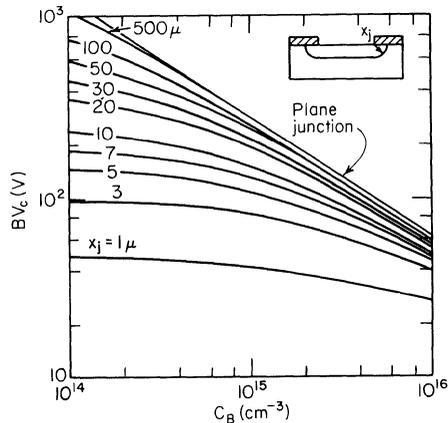
Fig. 1.34. Breakdown voltage of planar one-sided step junctions possessing various radii of curvature.<sup>21</sup>
