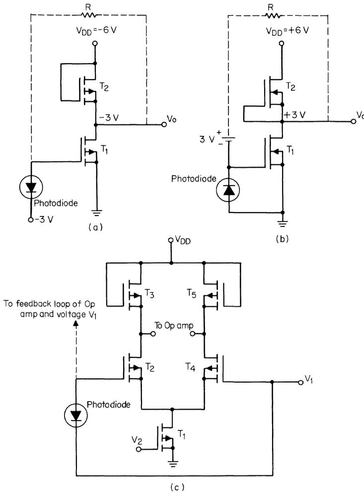
**Fig. 9.38.** (MOSFET amplifier front end for camera control. (a) p-channel enhancement-mode input pair; (b) n-channel depletion-mode input pair; (c) p-channel enhancement-mode differential input pair.
