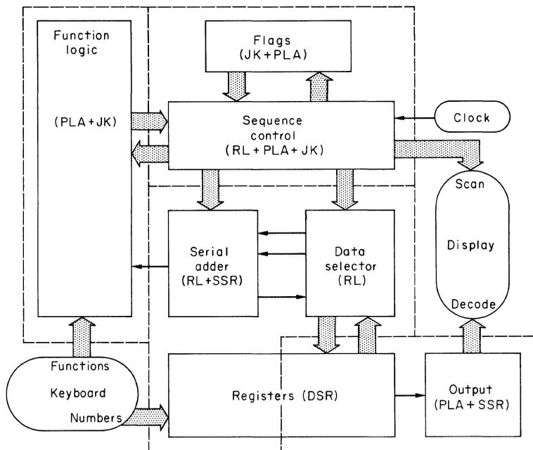
Fig. 10.17. Block diagram of the 1969 MOS calculator.
