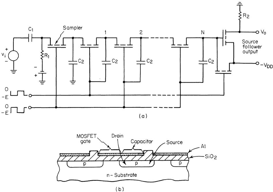
Fig. 9.33. (a) MOS/LSI version of the electronic delay line (bucket brigade)<sup>20</sup>; (b) cross section of a portion of the MOS/LSI electronic delay line.<sup>20</sup>
