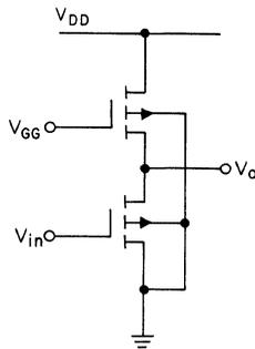
Fig. 4.1. Basic inverter circuit with common substrate.
