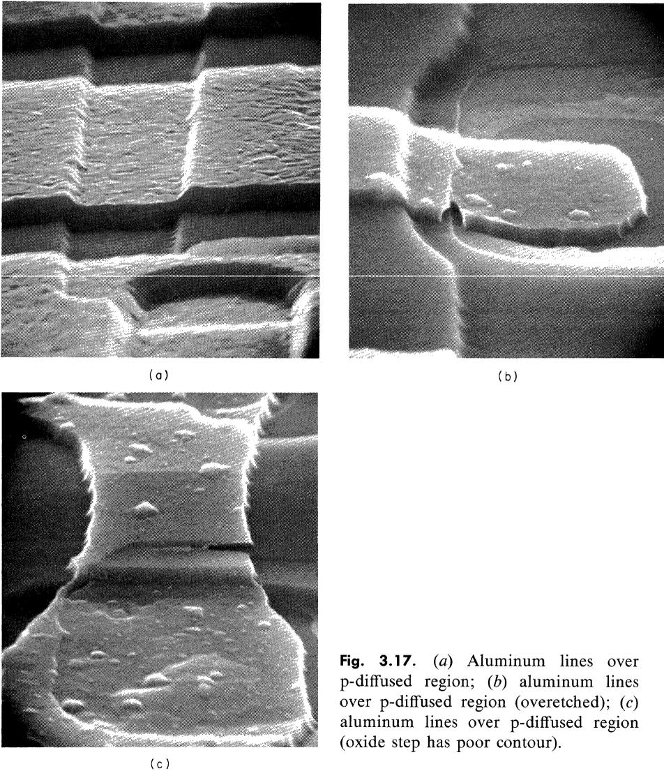
**Fig. 3.17.** (a) Aluminum lines over p-diffused region; (b) aluminum lines over p-diffused region (overetched); (c) aluminum lines over p-diffused region (oxide step has poor contour).
