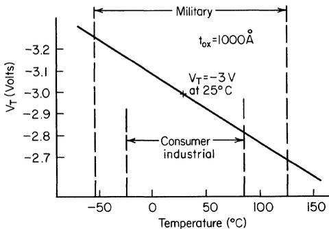
Fig. 3.2.  $V_T$  as a function of temperature.
