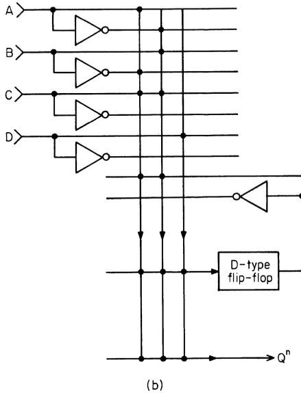
**Fig. 8.6.** PLA for implementing a clocked, pulse-clamping function with more complex data input trigger. The data trigger is  $A \oplus B + D$ . (a) Standard-logic schematic; (b) PLA-logic schematic.
