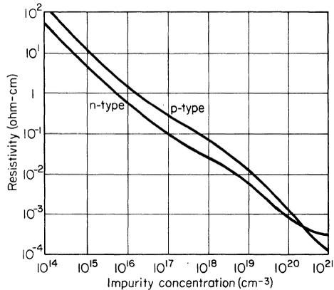
**Fig. 1.20.** Silicon resistivity at 300°K as a function of impurity concentration.<sup>11</sup>
