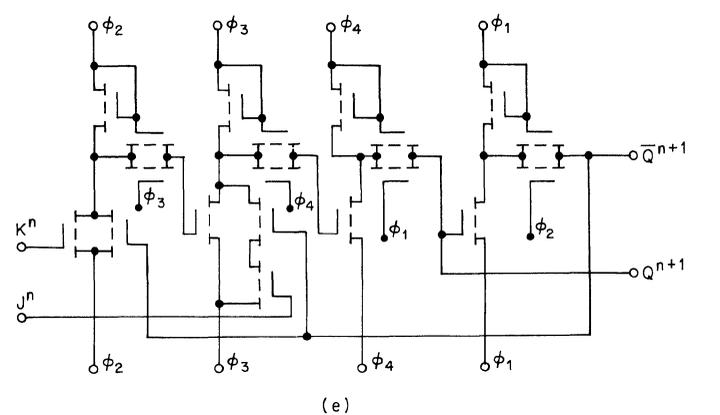
**Fig. 5.19.** *J-K* flip-flop;  $Q^{n+1} = J\bar{Q}^n + \bar{K}Q^n$ : (a) general circuit schematic; (b) logic implementation with  $2\phi$  ratio elements; (c) two-phase circuit schematic; (d) logic implementation with  $4\phi$  ratioless elements; (e) four-phase type circuit schematic.
