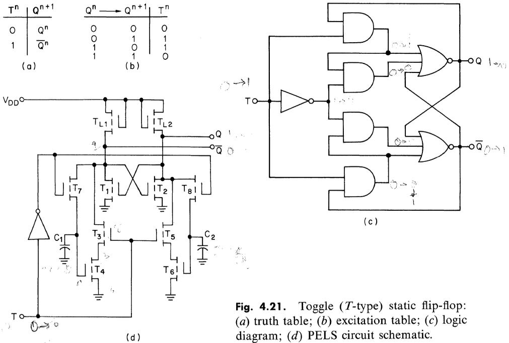
**Fig. 4.21.** Toggle (*T*-type) static flip-flop: (a) truth table; (b) excitation table; (c) logic diagram; (d) PEELS circuit schematic.
