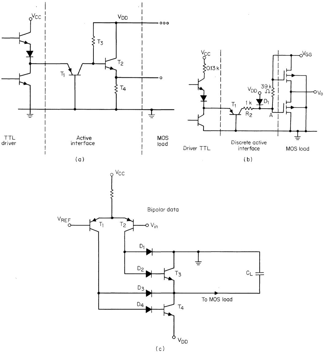
**Fig. 6.7.** Bipolar interface circuitry with increased logic swing for MOS load. MOS substrate is at system ground potential. (a) two-transistor translator; (b) single-transistor interface with diode pull-to- $V_{DD}$ ; (c) complementary drivers with increased drive capability.
