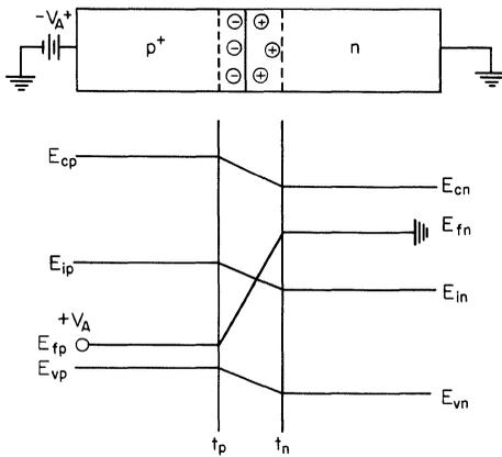
Fig. 1.25. Energy-level diagram for the p-n junction with applied forward bias.
