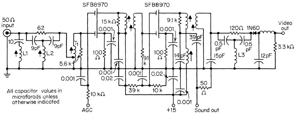
Fig. 9.43. TV receiver IF amplifier employing dual-gate MOSFETs.<sup>26</sup>
