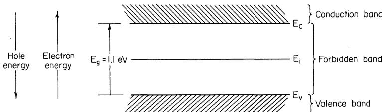
Fig. 1.7. Energy-level structure of silicon.
