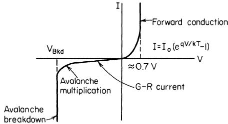
Fig. 1.31. General current-voltage characteristics of the silicon diode.
