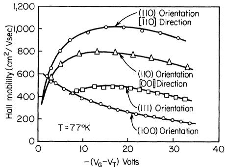
**Fig. 1.58.** Experimental values of inversion-layer hole mobility versus effective gate voltage ( $V_G - V_T$ ) for  $T = 77^\circ\text{K}$ .<sup>28</sup>
