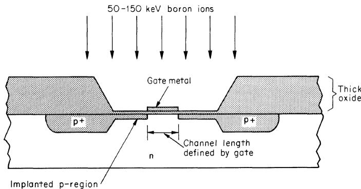
**Fig. 2.7.** Ion implantation of source and drain regions.
