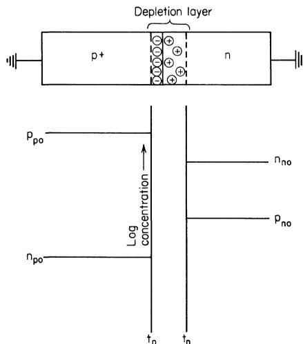
**Fig. 1.23.** Carrier concentration for the zero-biased p-n junction.
