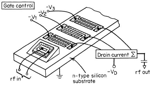
**Fig. 9.34.** Schematic of the MOSFET tapped delay line.<sup>22</sup>
