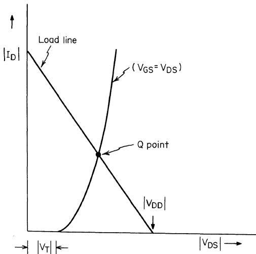
Fig. 9.3.  $Q$  point establishment with diode biasing.
