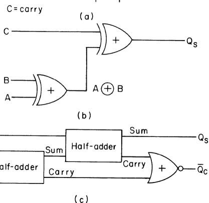
**Fig. 4.16.** Full-adder design: (a) truth table; (b) sum derived from dual XOR gates; (c) dual half-adders provide complete full-adder function.
