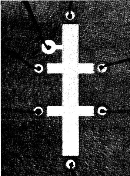
**Fig. 1.56.** p-channel enhancement-mode MOSFET in Hall geometry for measuring surface carrier mobility.<sup>28</sup>
