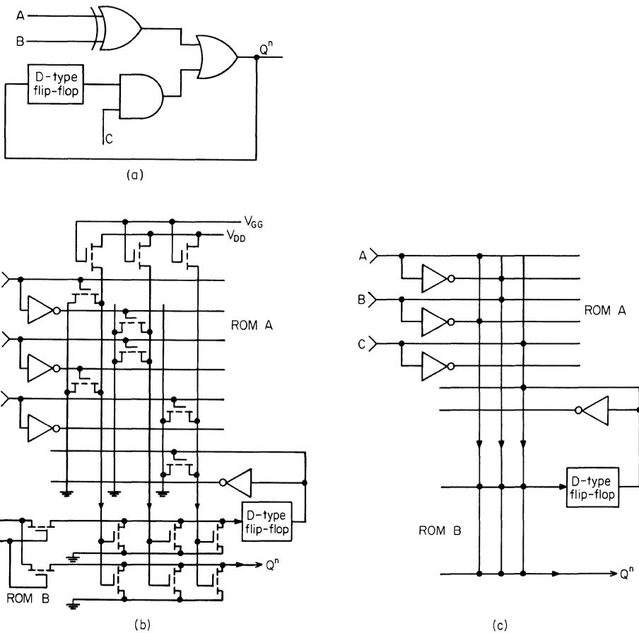
**Fig. 8.5.** PLA for implementing a pulse-clamping function with a clock and data trigger. An exclusive-OR ( $A \oplus B$ ) data input is used as a trigger. (a) Standard-logic schematic; (b) circuit schematic; (c) PLA-logic schematic.
