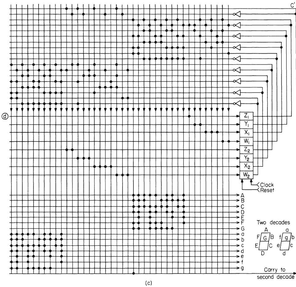
**Fig. 8.9.** PLA design sequence for the second digit of a modulo-100 counter in an application requiring a seven-segment decimal output. (a) Transition diagram for second decade; (b) multiple, 5-bit Karnaugh maps with logic functions for *D*-type flip-flops; second decade; (c) PLA-logic schematic with decoding for two (seven-segment) decimal digits.
