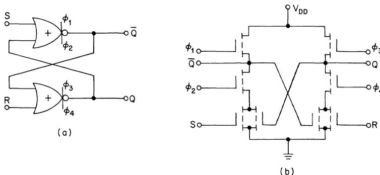
**Fig. 5.13.** Four-phase ratioless (type I) static element: (a) logic diagram; (b) circuit schematic.
