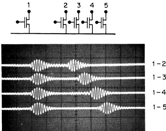
**Fig. 9.35.** Demonstration of the variable delay-line characteristics of the MOSFET detector array. Horizontal scale is 0.5 second per division.<sup>22</sup>
