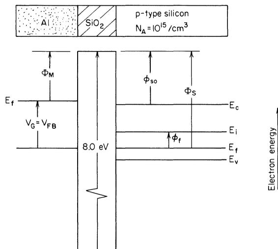
**Fig. 1.41.** Flat-band condition for the aluminum-SiO<sub>2</sub>-silicon system ( $N_A = 10^{15}/\text{cm}^3$ ).
