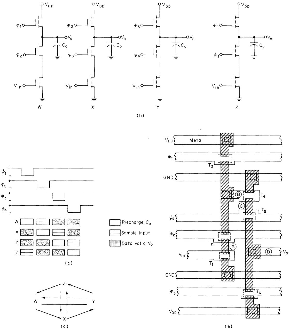
**Fig. 5.4.** Four-phase ratioless type I shift register: (a) circuit schematic; (b) phasing circuit combinations; (c) timing of pulses for (b); (d) permitted fan-outs; (e) layout geometry for 1  $W$ -bit.
