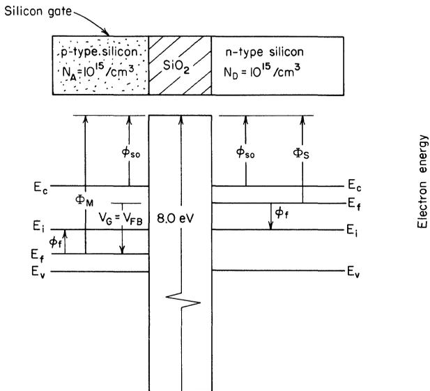
**Fig. 1.42.** Flat-band condition for the silicon gate ( $N_A = 10^{15}/\text{cm}^3$ )-SiO<sub>2</sub>-silicon system ( $N_D = 10^{15}/\text{cm}^3$ ).
