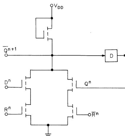
**Fig. 5.22.** Latching function:  $Q^{n+1} = DR + \bar{R}Q^n$ ; circuit implementation.
