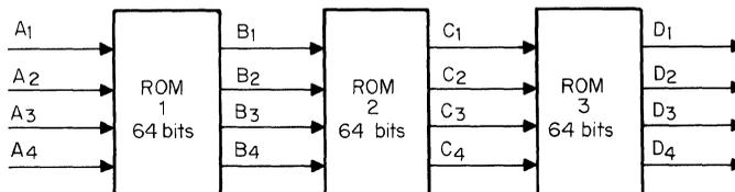
Fig. 7.7. Multiple levels of logic are obtained by stringing ROMs in sequence.
