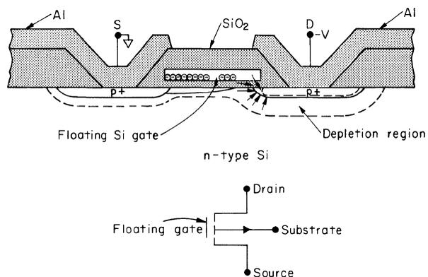
Fig. 2.14. The floating gate FAMOS structure.<sup>6</sup>
