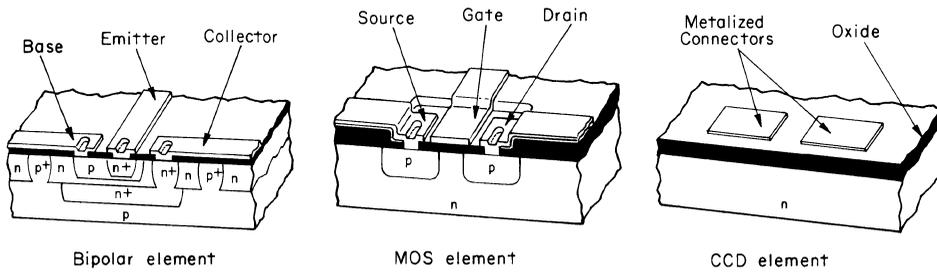
**Fig. 2.16.** Comparison of bipolar, MOSFET, and charge-coupled devices in cross-sectional view.<sup>7</sup>
