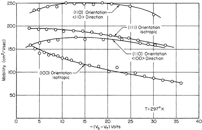
**Fig. 1.57.** Experimental values of inversion-layer hole mobility versus effective gate voltage ( $V_G - V_T$ ) for  $T = 297^\circ\text{K}$ .<sup>28</sup>
