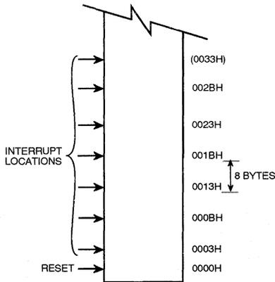
The interrupt service locations are spaced at 8-byte intervals : 0003H for External Interrupt 0, 000BH for Timer 0, 0013H for External Interrupt 1, 001BH for Timer 1, etc. If an interrupt service routine is short enough (as is often the case in control applications), it can reside entirely within that 8-byte interval. Longer service routines can use a jump instruction to skip over subsequent interrupt locations, if other interrupts are in use.
