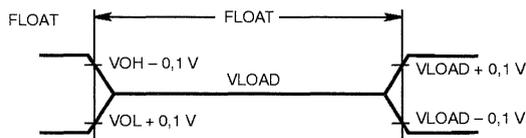
For timing purposes as port pin is no longer floating when a  $100 \text{ mV}$  change from load voltage occurs and begins to float when a  $100 \text{ mV}$  change from the loaded  $VOH/VOL$  level occurs.  $I_{OL}/I_{OH} \geq \pm 20 \text{ mA}$ .
