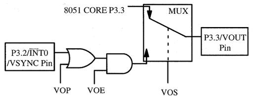
Figure 4. HSYNC and VSYNC outputs block diagram
