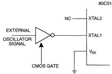
Rise and fall times are dependent on the external loading that each pin must drive. They are often taken to be something in the neighborhood of 10 nsec, measured between 0.8 V and 2.0 V.
