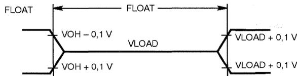
For timing purposes as port pin is no longer floating when a 100 mV change from load voltage occurs and begins to float when a 100 mV change from the loaded  $V_{OH}/V_{OL}$  level occurs.  $I_{OL}/I_{OH} \geq \pm 20$  mA.
