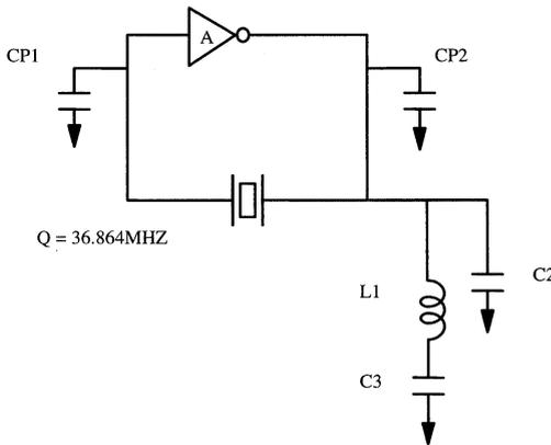
**Figure 1. Typical application with a third overtone crystal**
