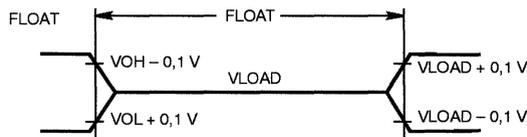
For timing purposes as port pin is no longer floating when a 100 mV change from load voltage occurs and begins to float when a 100 mV change from the loaded  $V_{OH}/V_{OL}$  level occurs.  $I_{OL}/I_{OH} \geq 20$  mA.
