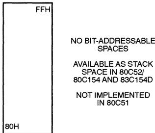
Figure 9 gives a brief look at the Special Function Register (SFR) space. SFRs include the Port latches, timers, peripheral controls, etc. These registers can only be accessed by direct addressing. In general, all C51 microcontrollers have the same SFRs as the 80C51, and at the same addresses in SFR space. However, enhancements to the 80C51 have additional SFRs that are not present in the 80C51, nor perhaps in other proliferation of the family.
