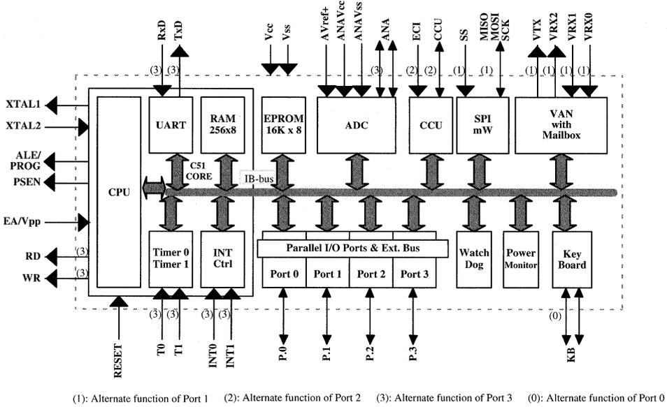
Figure 1. TSC8051A30 Block Diagram
