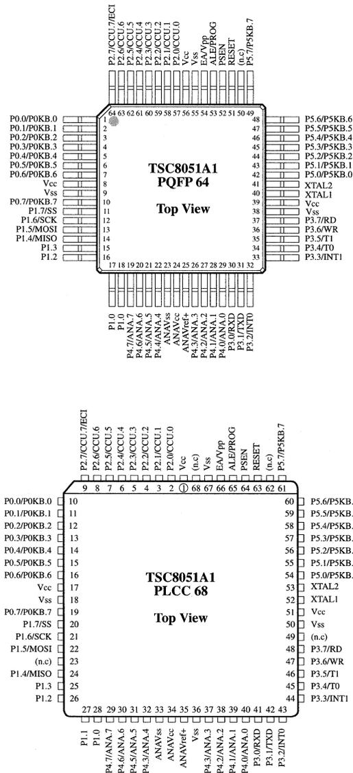
Figure 3. TSC8051A1 Pin Configuration
