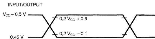
AC inputs during testing are driven at  $V_{CC} - 0.5$  for a logic "1" and  $0.45 V$  for a logic "0". Timing measurements are made at  $V_{IH \text{ min}}$  for a logic "1" and  $V_{IL \text{ max}}$  for a logic "0".
