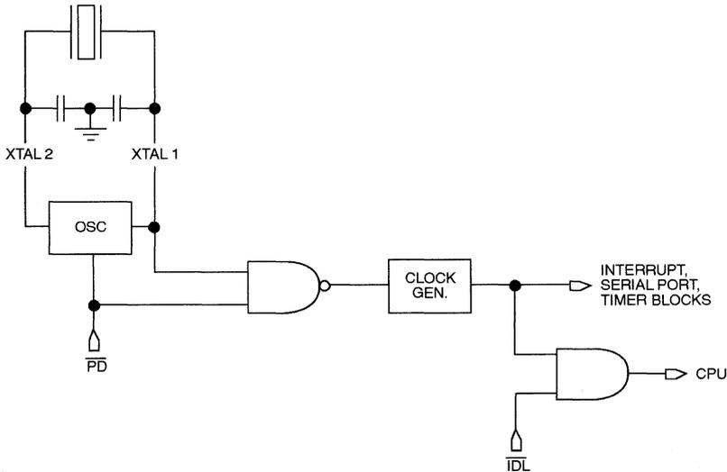
The only exit from Power Down is a hardware reset. Reset redefines all the SFRs, but does not change the on-chip RAM.
