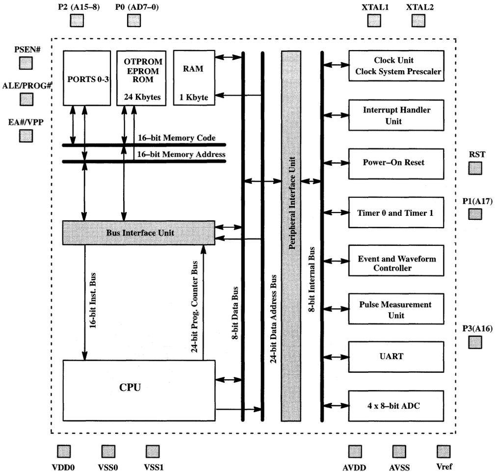
Figure 1. TSC80251A1 Block Diagram
