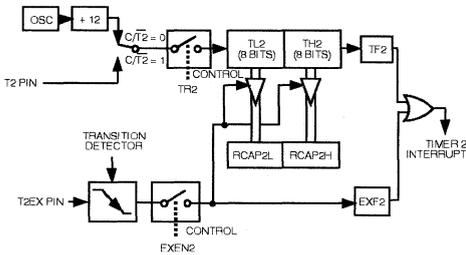
In the auto-reload mode there are again two options, which are selected by bit EXEN2 in T2CON. If EXEN2 = 0, then when Timer 2 rolls over it does not only set TF2 but also causes the Timer 2 register to be reloaded
