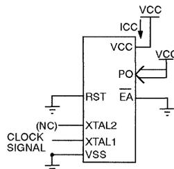
**Figure 10. ICC Test Condition, Active Mode.**
