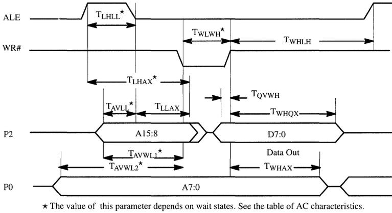
**Figure 6. External Write Data Bus Cycle in Page Mode**
