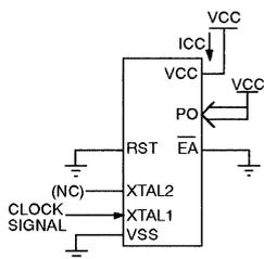
**Figure 16. ICC Test Condition, Power Down Mode.**
