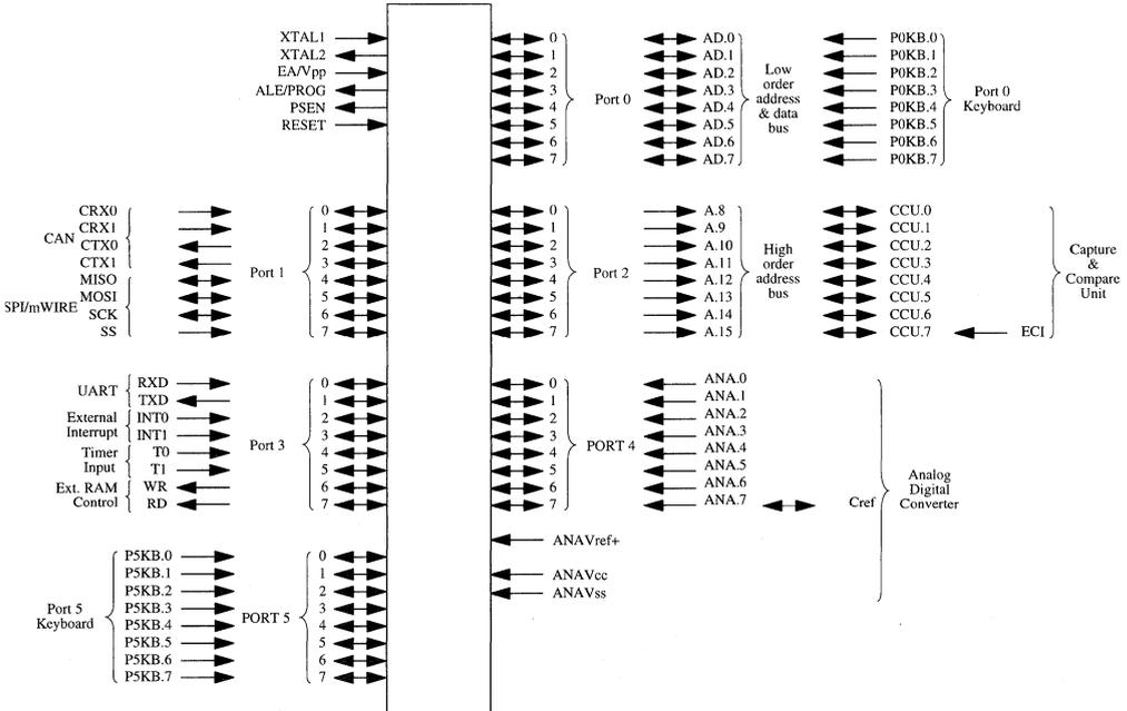
**Figure 2. TSC8051A11 pin functions**
