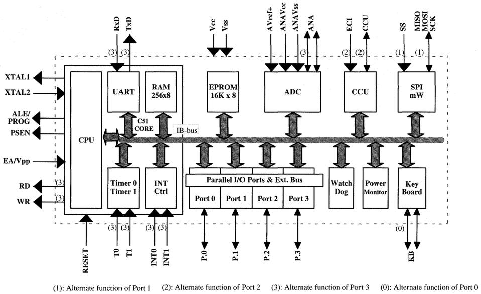
Figure 1. TSC8051A2 Block Diagram
