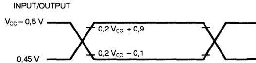
AC inputs during testing are driven at  $V_{cc} - 0.5$  for a logic "1" and 0.45 V for a logic "0". Timing measurements are made at  $V_{IH}$  min for a logic "1" and  $V_{IL}$  max for a logic "0".
