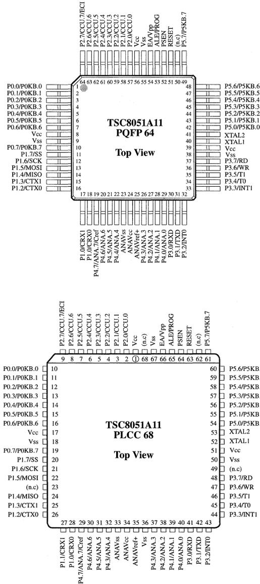
Figure 3. TSC8051A11 pin configuration
