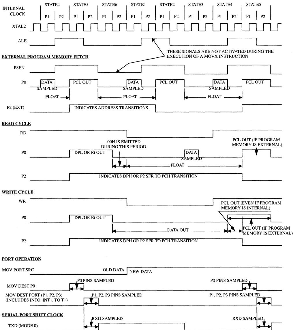
This diagram indicates when signals are clocked internally. The time it takes the signals to propagate to the pins, however, ranges from 25 to 125ns. This propagation delay is dependent on variables such as temperature and pin loading. Propagation also varies
