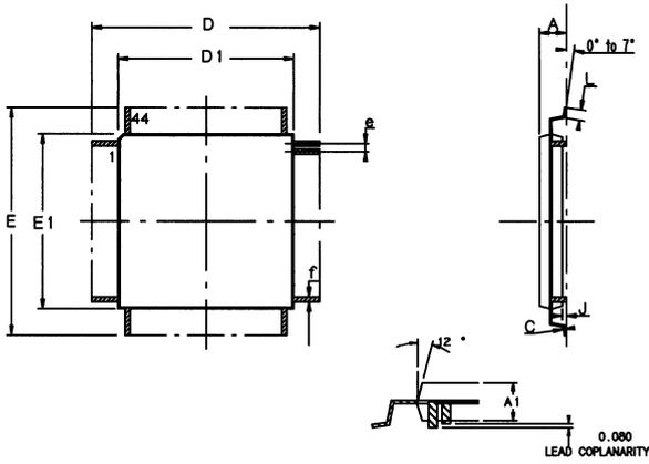
**Figure 7. TQFP Package Size**
