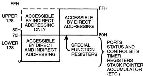
The Lower 128 bytes of RAM are present in all C51 devices as mapped in Figure 7. The lowest 32 bytes are grouped into 4 banks of 8 registers. Program instructions call out these registers as R0 through R7. Two bits in the Program Status Word (PSW) select which register bank is in use. This allows more efficient use of code space, since register instructions are shorter than instructions that use direct addressing.
