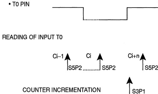
The counter will only evolve if a level 1 is detected during state S5P2 of cycle  $C_i$  and if a level 0 is detected during state S5P2 of cycle  $C_i + n$ .
