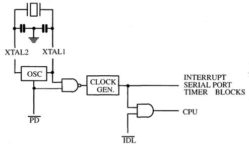
Figure 3. Idle and Power Down Hardware.
