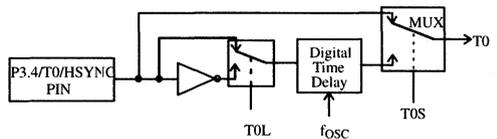
**Figure 16. T0/HSYNC input block diagram**
