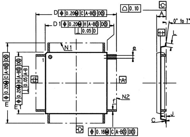
Figure 8. PQFP Package Size
