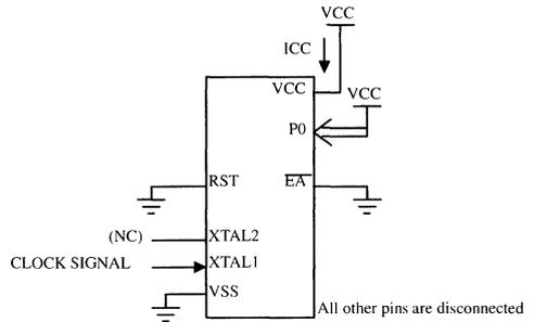
**Figure 18. ICC Test Condition, Idle Mode.**
