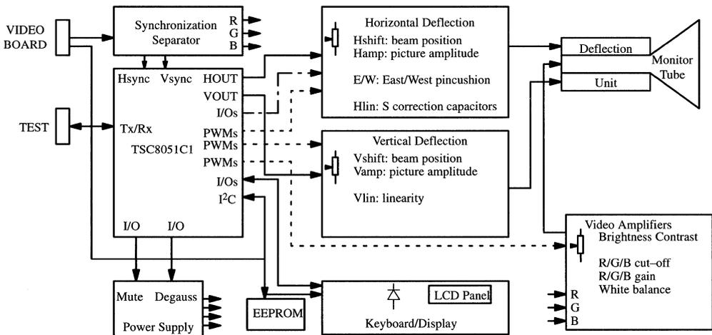
Figure 1. Autosync monitor block diagram with the TSC8051C1
