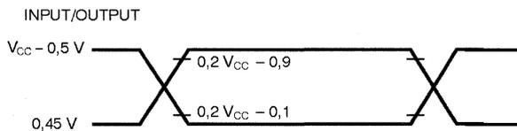
AC inputs during testing are driven at  $V_{CC} - 0.5$  for a logic "1" and 0.45 V for a logic "0". Timing measurements are made at  $V_{IH}$  min for a logic "1" and  $V_{IL}$  max for a logic "0".
