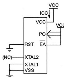
**Figure 15. ICC Test Condition, Active Mode.**
