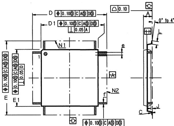
Figure 4. PQFP Package Size
