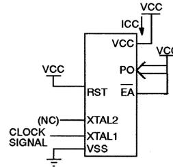
**Figure 9. ICC Test Condition, Power Down Mode.**
