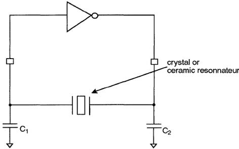
The Figure 34. shows the use of a crystal working on an overtone 3 resonance.
