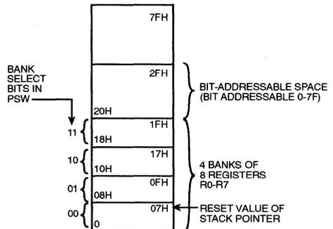
The next 16 bytes above the register banks form a block of bit-addressable memory space. The C51 instruction set includes a wide selection of single-bit instructions, and the 128 bits in this area can be directly addressed by these instructions. The bit addresses in this area are 00H through 7FH.
