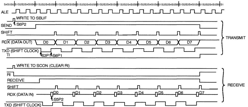
**Figure 23. Serial Port Mode 1. TCLK, RCLK, and Timer 2 are present in the 80C32/80C52, 80C154/83C154 and 83C154D.**
