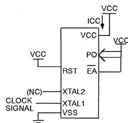
**Figure 11. ICC Test Condition, Power Down Mode.**
