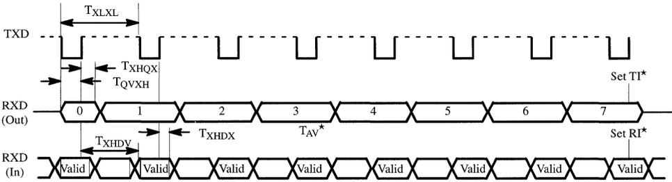
**Figure 7. Serial Port Waveform – Shift Register Mode**
