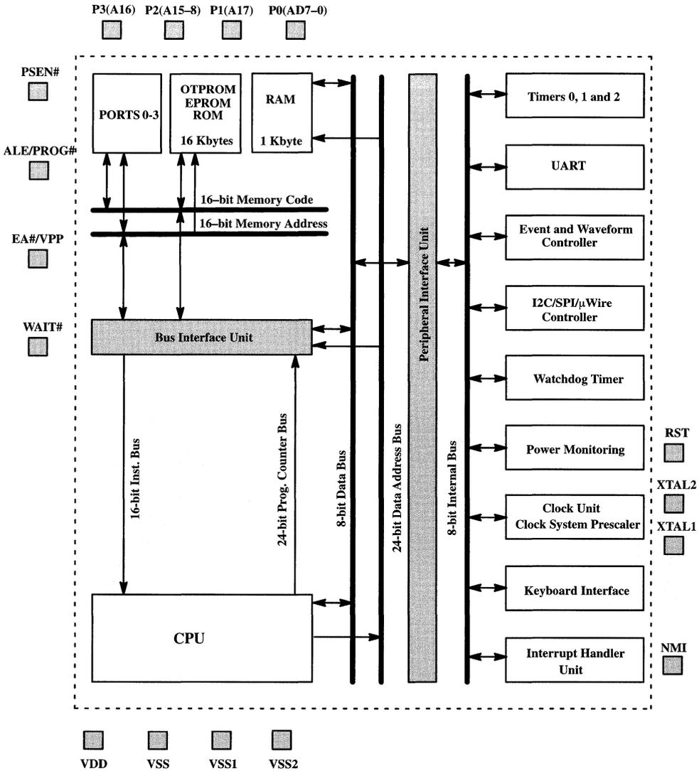
Figure 2. TSC80251G1 Block Diagram
