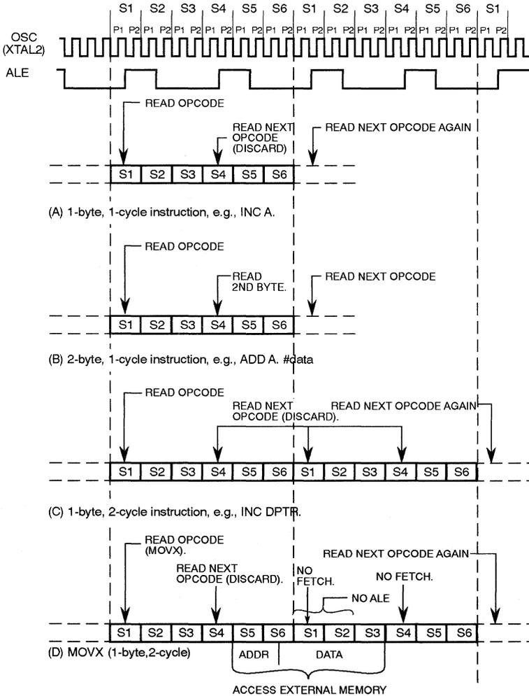
Execution of a one-cycle instruction (Figure 15A and B) begins during State 1 of the machine cycle, when the opcode is latched into the Instruction Register. A second fetch occurs during S4 of the same machine cycle. Execution is completed at the end of State 6 of this machine cycle.
