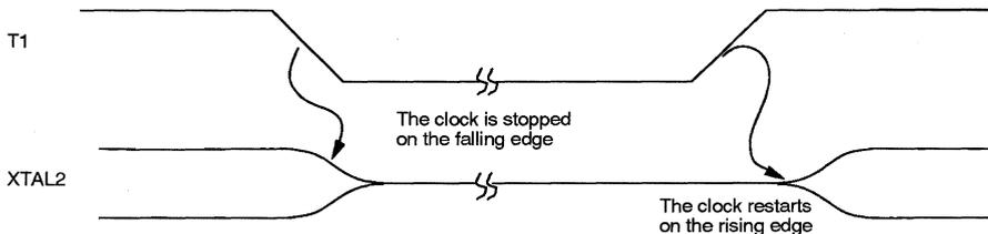
The time takes by the oscillator to restart depends of the crystal and the capacitors connected on both side of the crystal (typically 10 ms).
