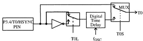
**Figure 14. T0/HSYNC input block diagram**
