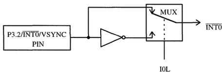
**Figure 13.  $\overline{\text{INT0}}/\text{VSYNC}$  input block diagram**
