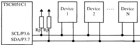
**Figure 15. Typical I<sup>2</sup>C bus configuration**
