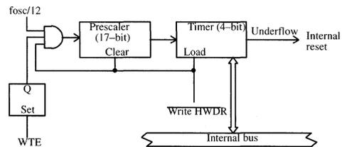
**Figure 9. Watchdog timer block diagram**
