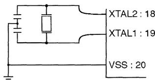
**Figure 6. External Drive Configuration.**
