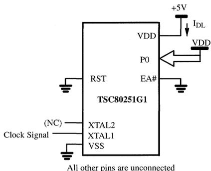
Figure 9.  $I_{DL}$  Test Condition, Idle Mode
