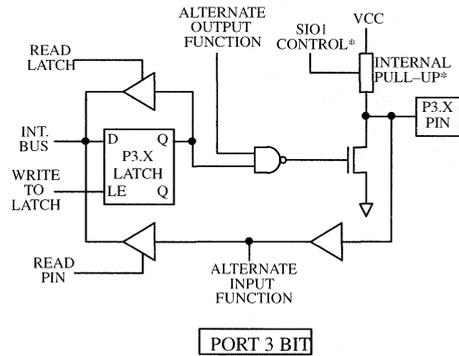
\* Internal pull-up not present on P3.6 and P3.7 when SIO1 is enabled.
