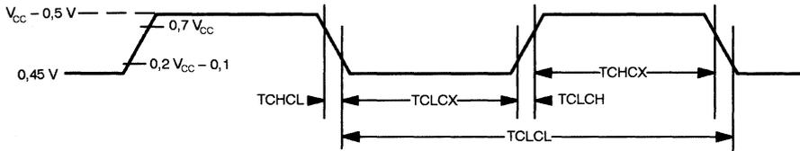
**AC Testing Input/Output Waveforms**
