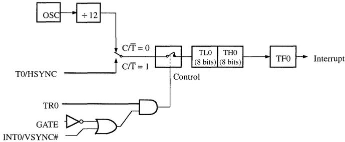
**Figure 5. Timer/Counter 0 in mode 1: 16-bit Counter**
