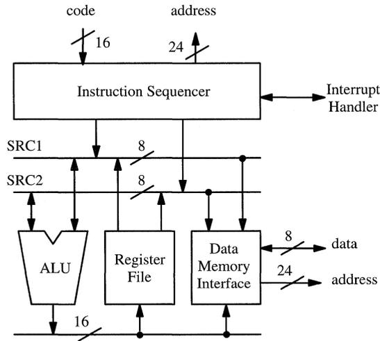
Figure 2. Central Processor Unit Block Diagram
