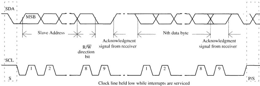
**Figure 16. Complete data transfer on I<sup>2</sup>C bus**
