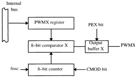
**Figure 12. Pulse width modulated outputs block diagram**
