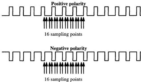
**Figure 8. Hsync polarity detection**
