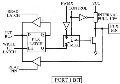
\* Internal pull-up not present on P1.0 to P1.3 when PWM8 to PWM11 are enabled
