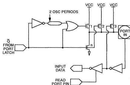
When the port latch contains a 0, all pFETS in figure 4 are off while the nFET is turned on. When the port latch makes a 0-to-1 transition, the nFET turns off. The strong pFET, T1, turns on for two oscillator periods, pulling the output high very rapidly. As the output line is drawn high, pFET T3 turns on through the inverter to supply the IOH source current. This inverter and T form a latch which holds the 1 and is supported by T2.
