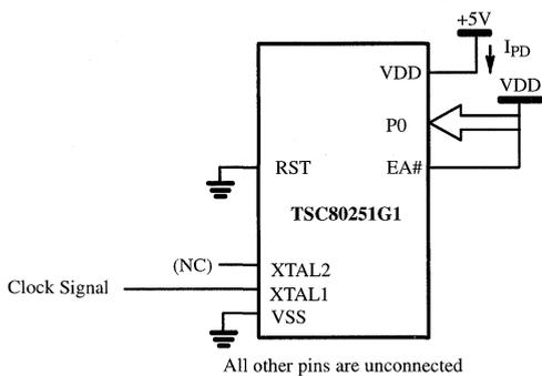
Figure 8.  $I_{DD}$  Test Condition, Power-Down Mode
