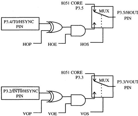
**Figure 14. Buffered HSYNC and VSYNC block diagram**
