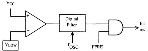
**Figure 10. Power-Fail Reset block diagram**
