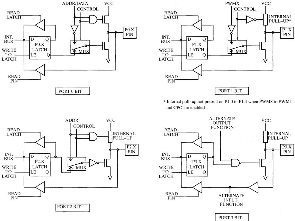
\* Internal pull-up not present on P1.0 to P1.4 when PWM8 to PWM11 and CPO are enabled
