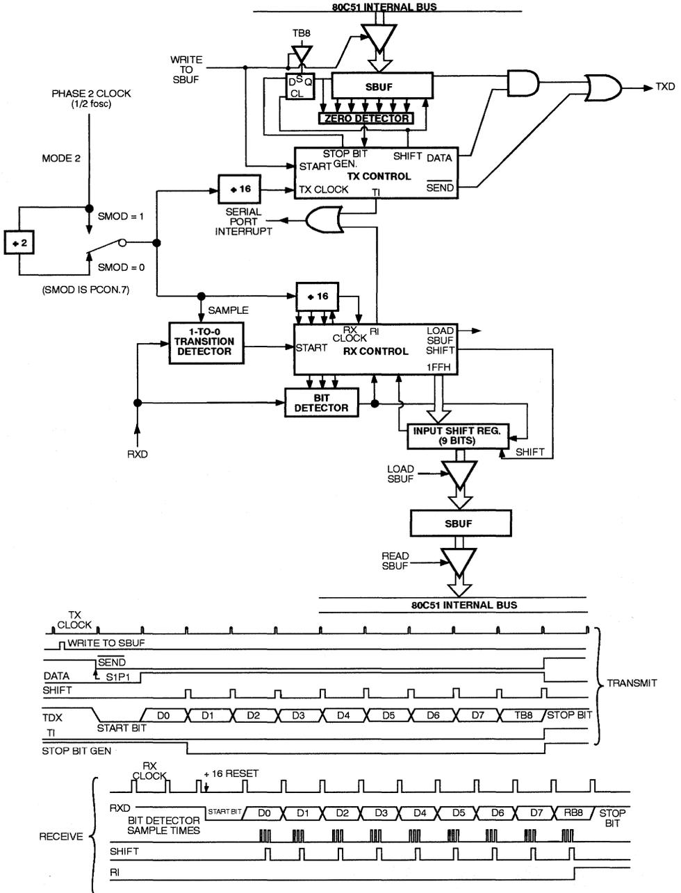
Figure 25. Serial Port Mode 3. TCLK, RCLK and Timer 2 are present in the 80C32/80C52, 80C154/83C154 and in the 83C154D.
