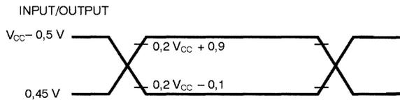
AC inputs during testing are driven at  $V_{CC} - 0.5$  for a logic "1" and  $0.45\text{ V}$  for a logic "0". Timing measurements are made at  $V_{IH\text{ min}}$  for a logic "1" and  $V_{IL\text{ max}}$  for a logic "0".
