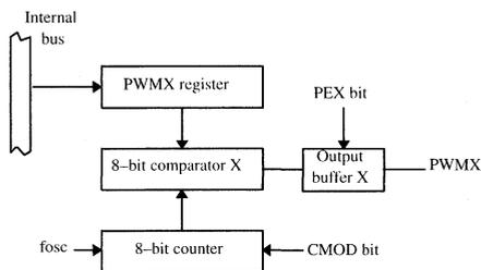
**Figure 10. Pulse width modulated outputs block diagram**
