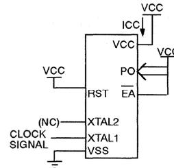
**Figure 17. ICC Test Condition, Power Down Mode.**
