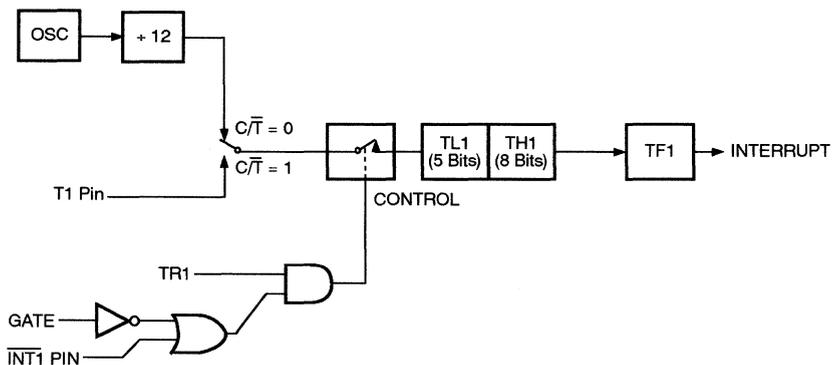
The 13-bit register consists of all 8 bits of TH1 and the lower 5 bits of TL1. The upper 3 bits of TL1 are indeterminate and should be ignored. Setting the run flag ( $TR1$ ) does not clear the registers.
