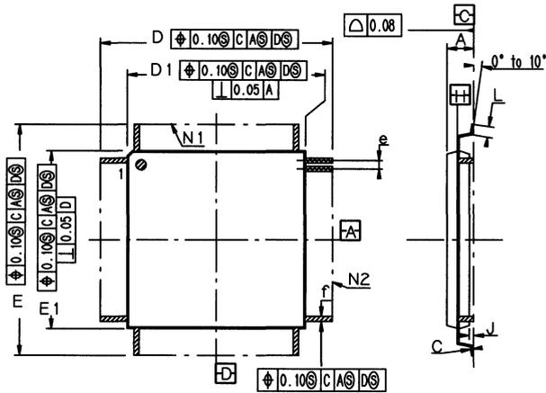
**Figure 5. PQFP Package Size**
