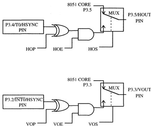
**Figure 12. Buffered HSYNC and VSYNC block diagram**
