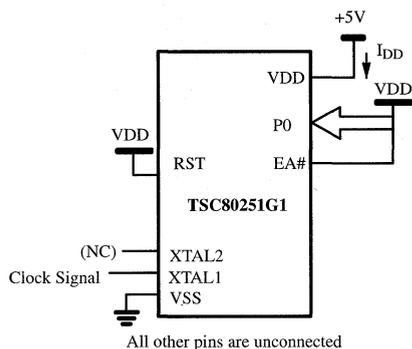
Figure 10.  $I_{DD}$  Test Condition, Active Mode
