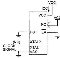
**Figure 16. ICC Test Condition, Active Mode.**
