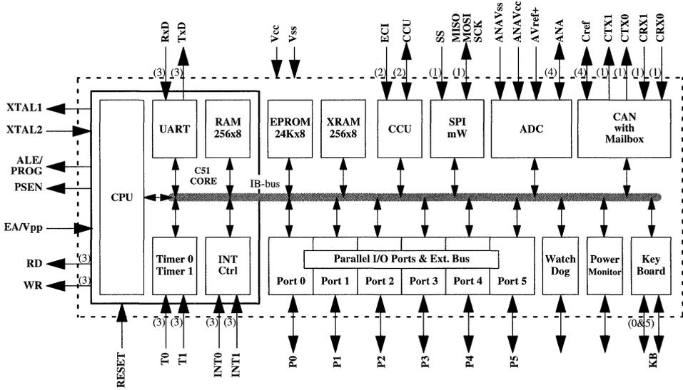
(1): Alternate function of Port 1 (2): Alternate function of Port 2 (3): Alternate function of Port 3 (4): Alternate function of Port 4
