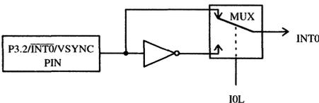
**Figure 15.  $\overline{\text{INT0}}/\text{VSYNC}$  input block diagram**
