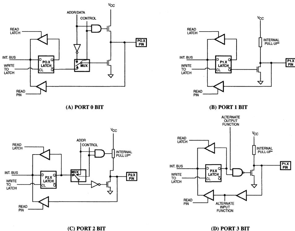
\* See Figure 7. for details of the internal pullup.
