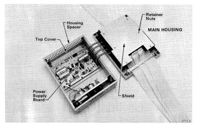
Fig. 2-1. Access to Power Supply board.
