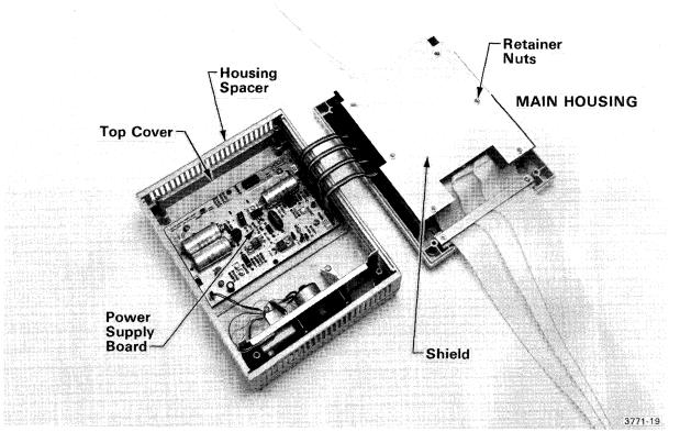
Fig. 4-1. Access to Power Supply board.
