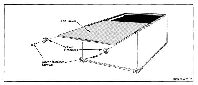
Fig. 3-1. Removal/installation of top cover.
