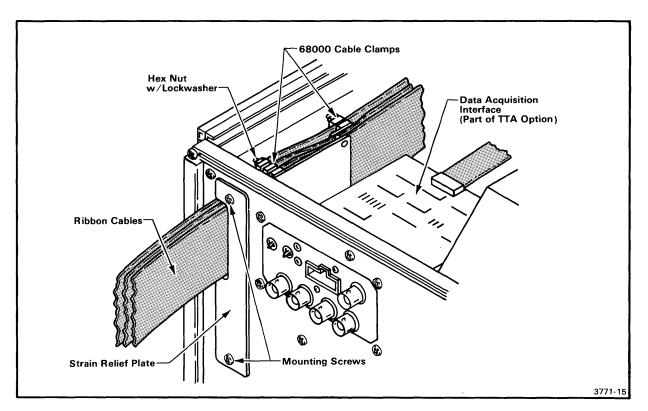
Fig. 3-5. Strain relief plate installation/removal.
