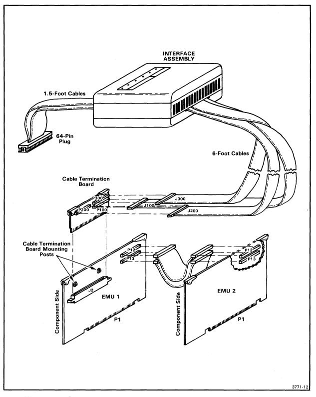
Fig. 3-2. 68000 Emulator Processor with Prototype Control Probe.
