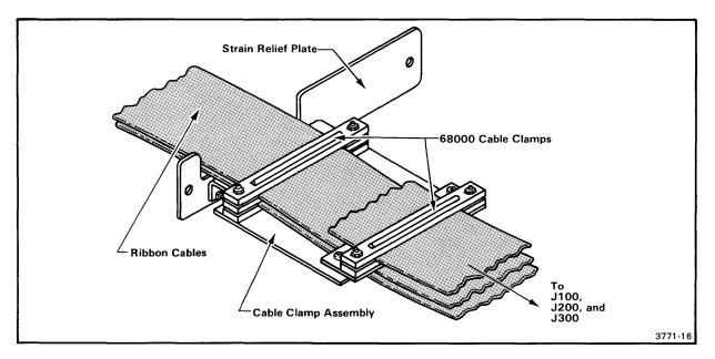
Fig. 3-6. Ribbon cable installation.
