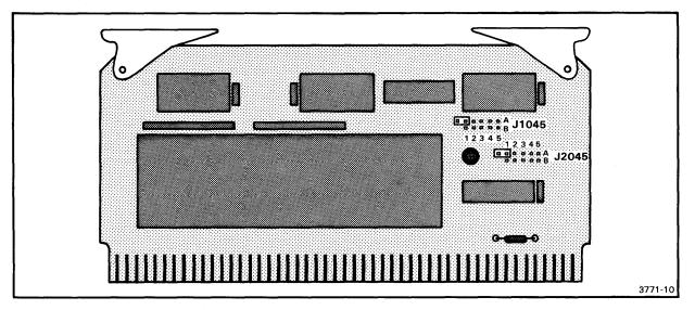
Fig. 2-7. Mobile Microprocessor board jumper locations.
