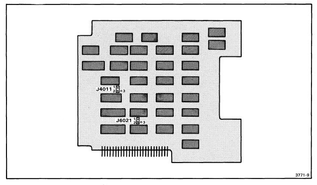
Fig. 2-6. Control board jumper locations.
