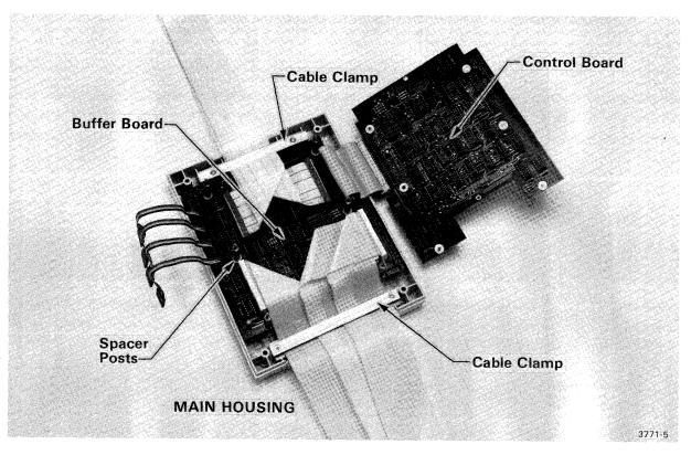
Fig. 2-2. Access to Control board and Buffer board.
