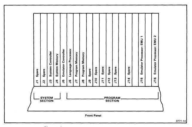
Fig. 3-4. Recommended module arrangement.
