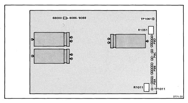
Fig. 4-2. Power Supply board.
