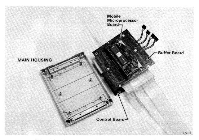
Fig. 2-3. Access to Mobile Microprocessor board.
