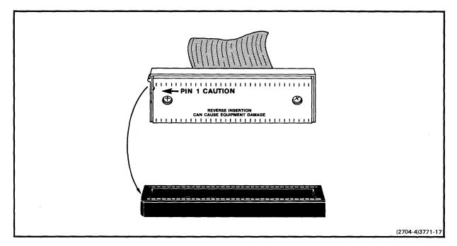
Fig. 3-7. Pin identification and proper plug insertion.
