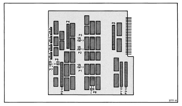
Fig. 2-5. Buffer board jumper locations.
