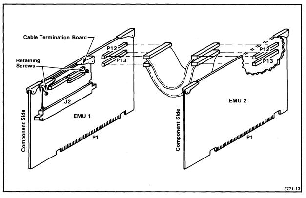
Fig. 3-3. EMU 1/EMU 2 interconnection with Cable Termination board.
