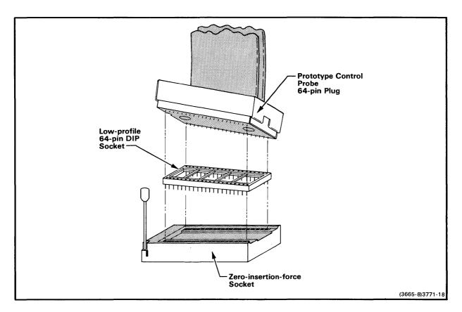
Fig. 3-8. Using a zero-insertion-force socket.
