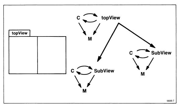
Figure 7. Hierarchy of Model-View-Controllers.
