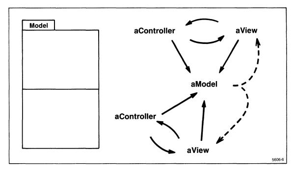
Figure 6. Double Window With Two Model-View-Controllers.
