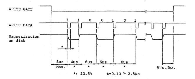
(Fig. 105) WRITE DATA timing (MFM method)
