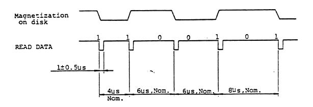
Note: The displacement of any bit position does not exceed ±700nsec from its nominal position. (When PLO separator is used with zero write pre-compensation.)
