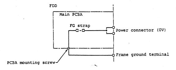
(Fig. 109) Frame ground internal connection
