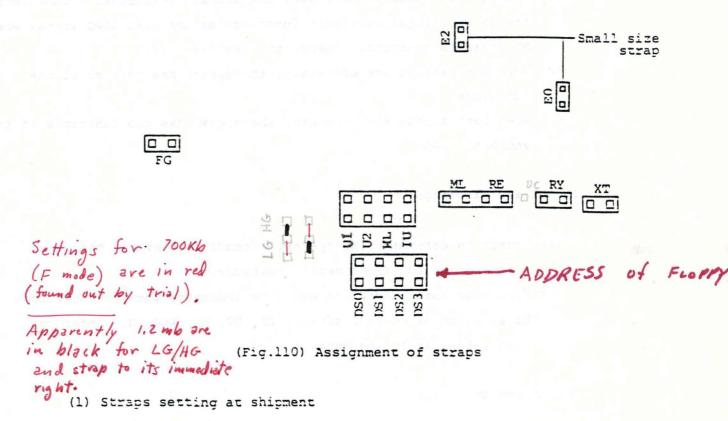
The FDD is shipped with the following straps set to on-state:
