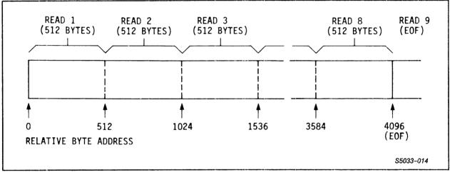
Figure 5-1. Example of Encountering EOF
