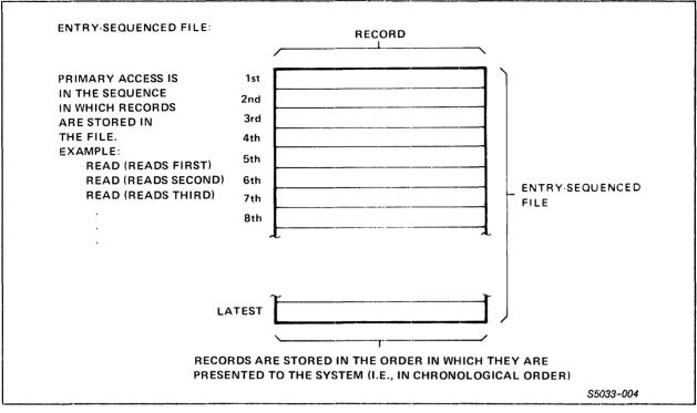
Figure 1-4. Entry-Sequenced File Structure
