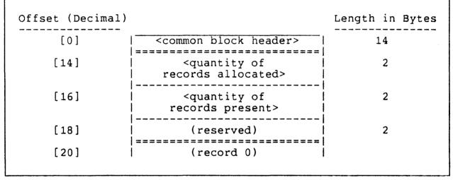
Figure B-6. Header for DP2 Relative Data Block
