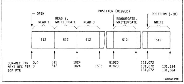
Figure 5-3. Example of File-Pointer Action
