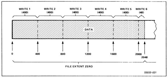
Figure 5-8. Example Showing Extent-Allocation Error
