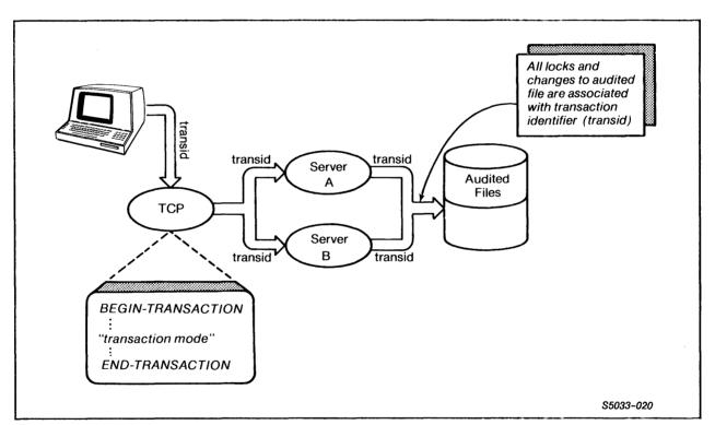
Figure 5-7. Record-Locking by Transaction Identifier
