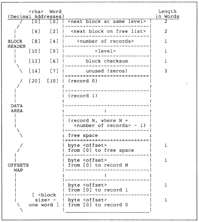
Figure B-1. Block Format for Structured Files (non-DP2 systems)
