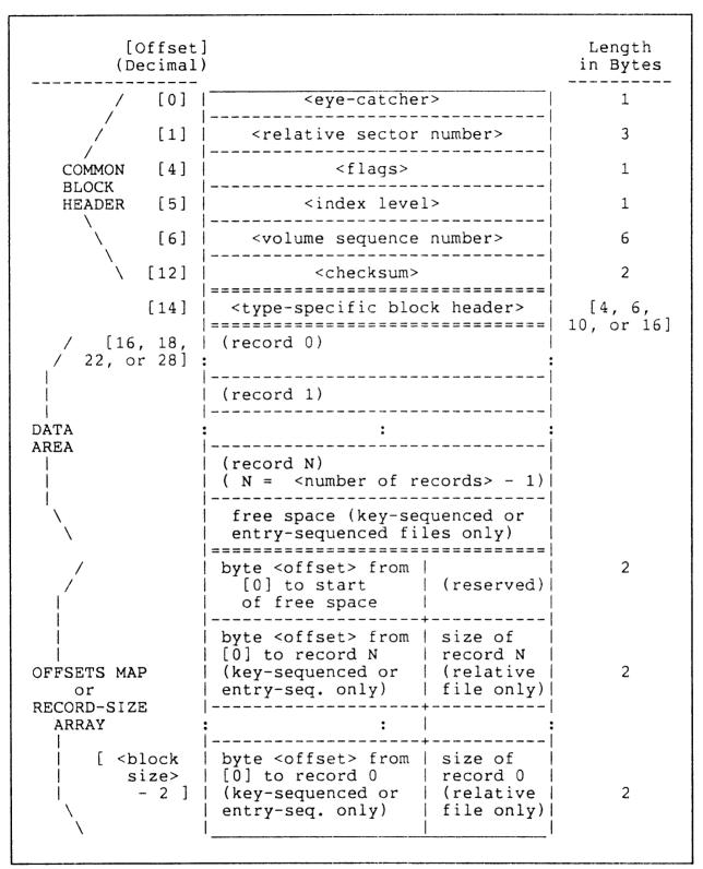
Figure B-2. Block Format for DP2 Structured Files
