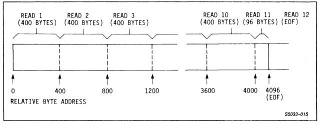
Figure 5-2. Example of Encountering EOF (Short READ)
