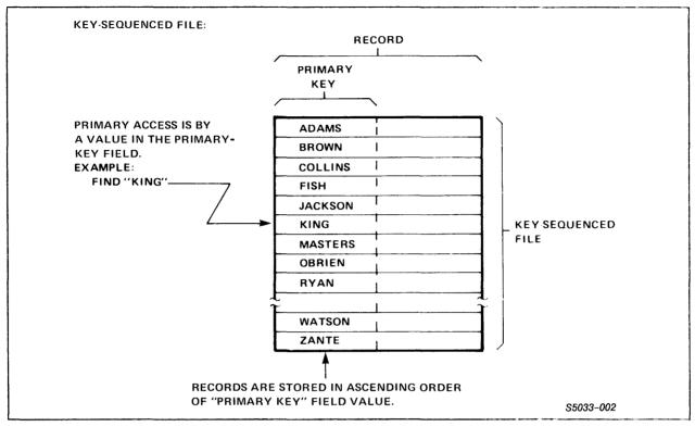
Figure 1-2. Key-Sequenced File Structure
