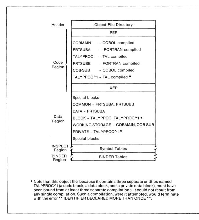
Figure 4-1. Example of BINDER's Object File Format
