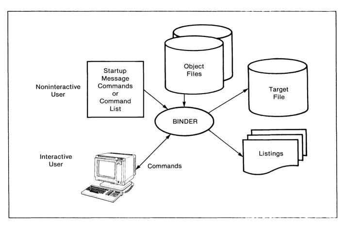
Figure 1-3. Using BINDER in Command-driven Mode
