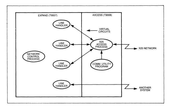
Figure 1-3. A System with Direct-Connect and X.25 Line Handlers
