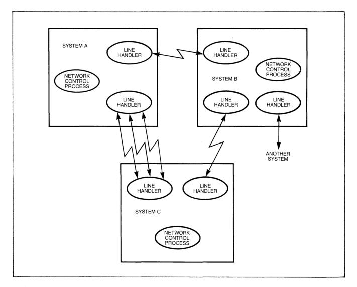
Figure 1-2. A Network Containing Only Direct-Connect Line Handlers
