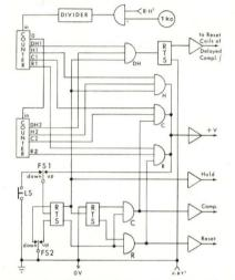
Figure 2. Iterative Operation Logic Control Circuit
