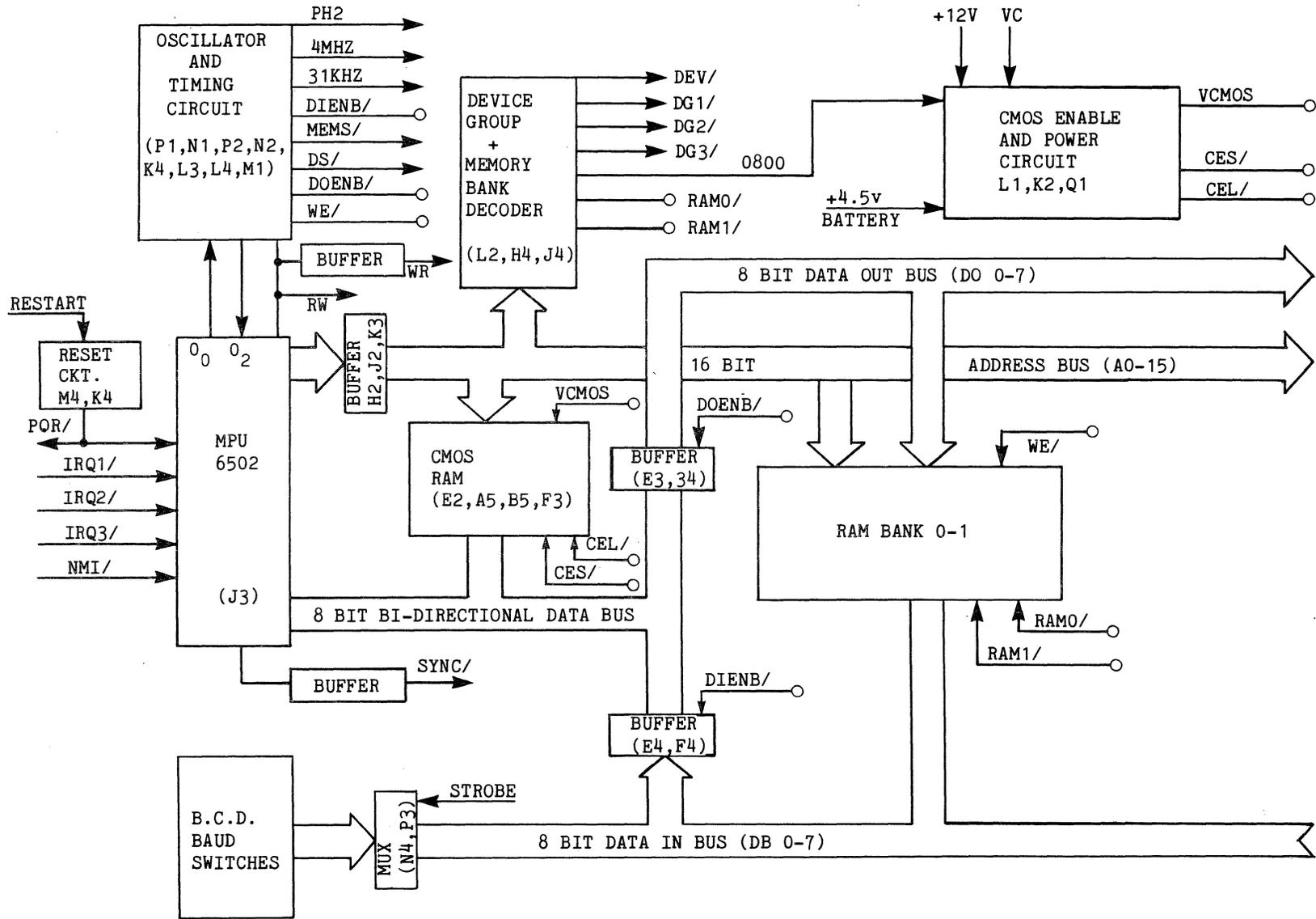
FIGURE #6-1(B) BLOCK DIAGRAM OF THE MP-RAM BOARD FOR Comm-Stor IV
