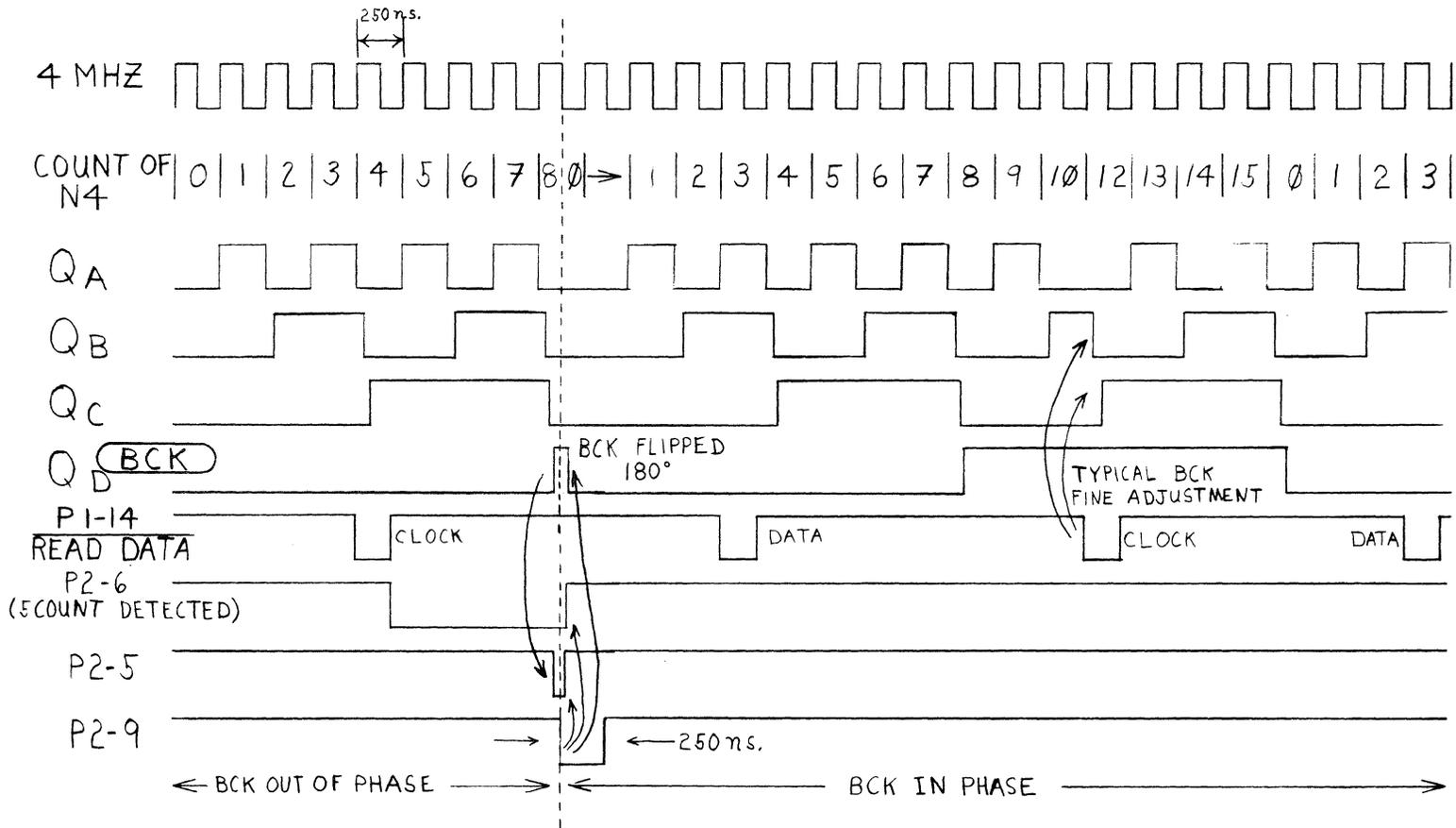
BIT CLOCK GENERATION TIMING DIAGRAM
