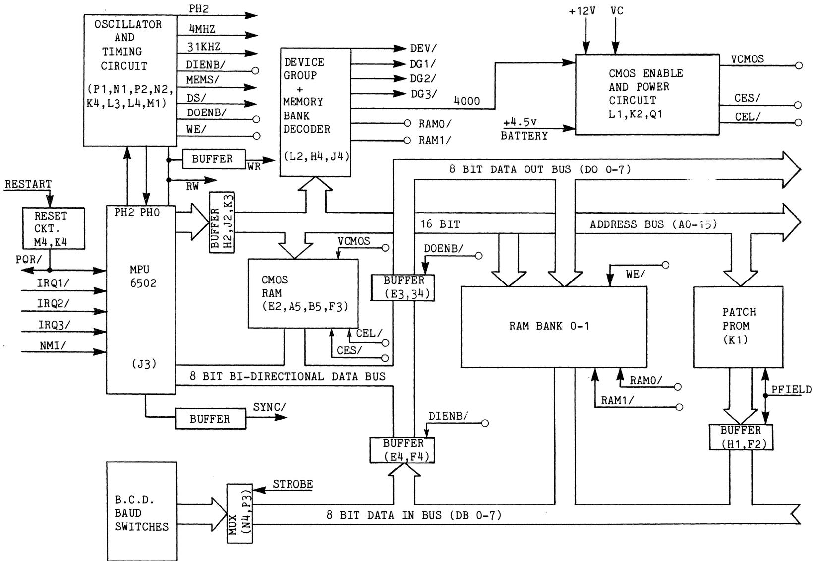
FIGURE #6-1(A) BLOCK DIAGRAM OF THE MP-RAM BOARD FOR Comm-Stor and Comm-Stor II/III
