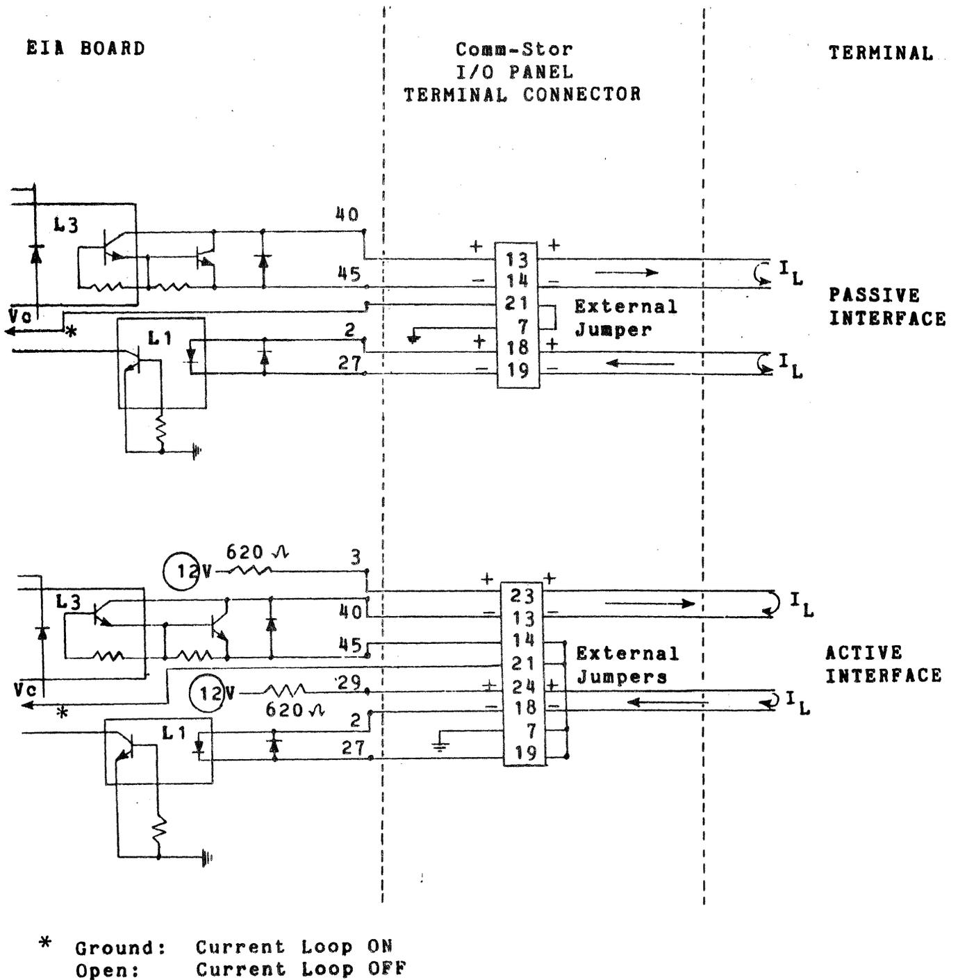
FIGURE #7-4 CURRENT LOOP CONNECTIONS (20 mA)
