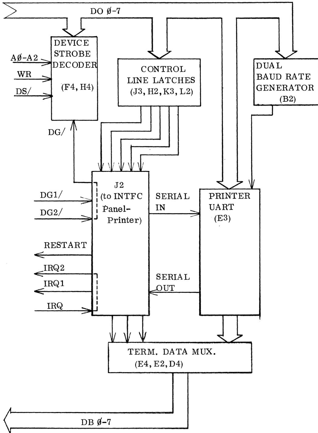
BLOCK DIAGRAM OF PRINTER PORT BOARD
