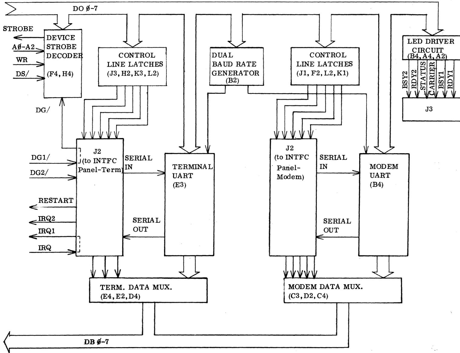
BLOCK DIAGRAM OF THE COMMUNICATIONS PORTS BOARD
