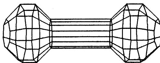
A solid of rotation can be **made** by sweeping a wire face into a sheet (of rotation) and by closing the sheet with the "**R**" command (Rotation Completion. For example a dumbbell shaped object is formed by typing the following commands:
