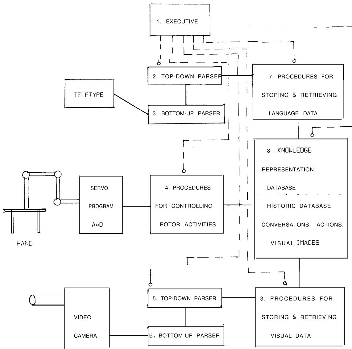
Figure 1. A possible segmentation of a robot.
