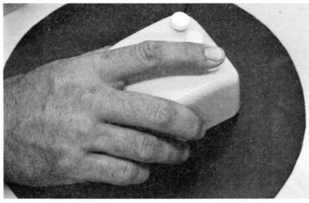
FIGURE 14. The user returns his left hand to the keyset and his right hand to the mouse. To confirm his command to compile the pattern "Research" he presses the right hand button on top of the mouse.
