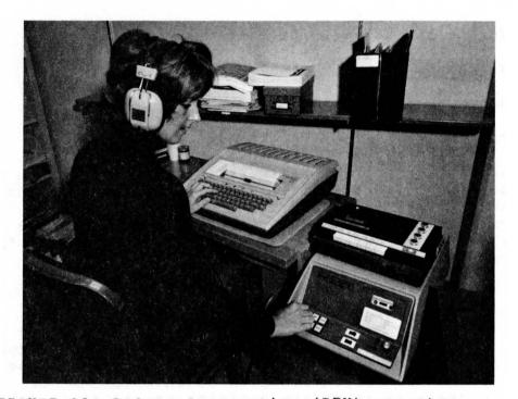
FIGURE 20. Deferred execution (DEX) operator transcribing a meeting. The black box to the operator's right plays an audio tape of the meeting. She types the words on her terminal and the terminal output is recorded by the digital tape machine that she is touching with her right hand. The digital tapes are read onto our disk storage and processed into NLS format at leisure.
