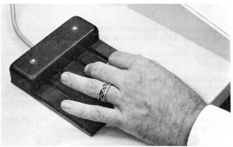
FIGURE 10. User calls the Goto Programs Subsystem by entering the first letter of each command via a keyset. On the keyset he can enter with one hand all characters that can be entered from a keyboard. The other hand is free to use the mouse (below).
