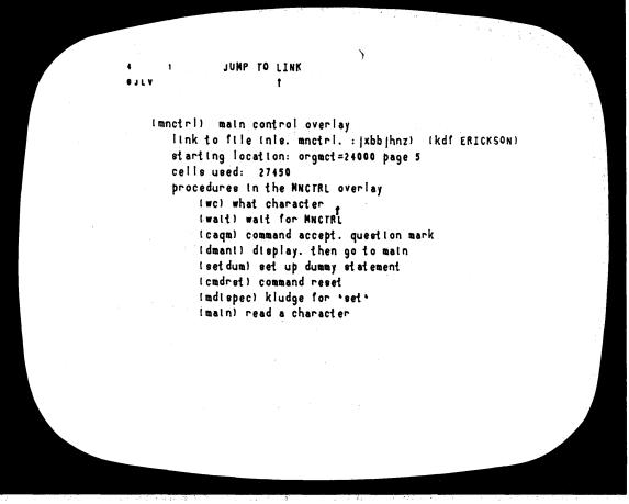
FIGURE III-8 A BRANCH GIVING SUPPORTIVE INFORMATION FOR MAIN-CONTROL (MNCTRL) OVERLAY. Display shows only the first line of each statement. A "Jump to Link" command has been partially specified—no selection has been made.
