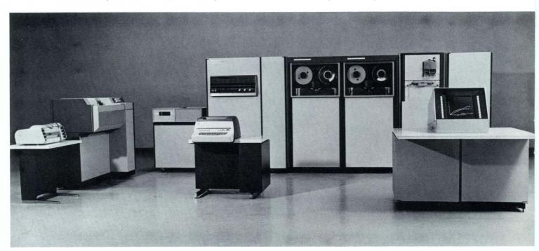
entire 8K-word memory module. Execution of another 1.2-microsecond transfer instruction preserves any protect code by storing it in a general-purpose register. The software for SYSTEMS 86 exploits the speed of the memory protect feature when allocating core in multiprogramming environments.
