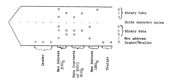
The distinction between RIM and BIN is that any number of Data words may follow an Address word, each filling successive locations with BIN tape while with RIM tape each Data word must be preceded by an Address word. Also, BIN tape often has a check-sum word at the end of the tape. The Bootstrap-loader switch will read either format, but will ignore any check-sums.
