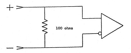
FIGURE 10 : RS 422 DIFFERENTIAL LINE RECEIVER
