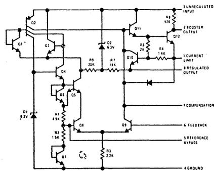
Pin connections shown are for TO-5 package
