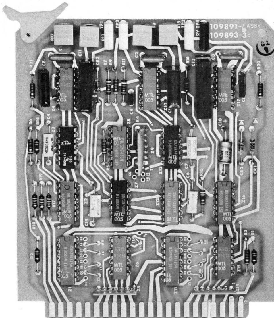
Figure 7-16. Step Motor Driver Card 109891-660 Assembly.
