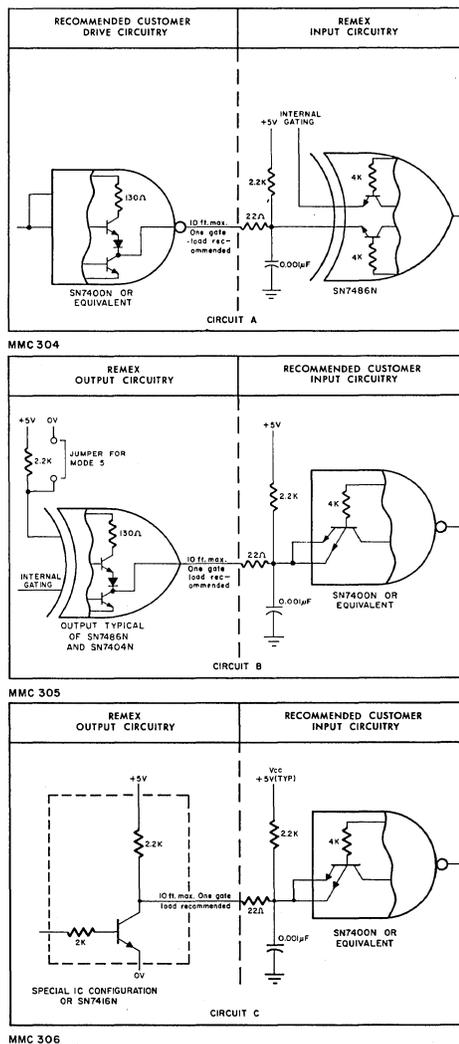
Figure 2-2. Recommended Interface Circuitry.
