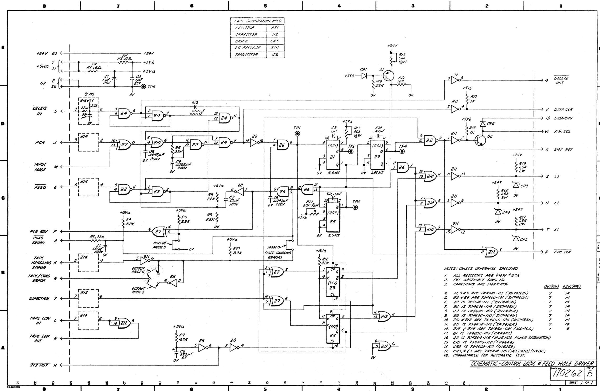
RSM-207V Figure 8-5. Schematic, Control Logic and Feed Hole Driver Card 8-11/8-12 110261
