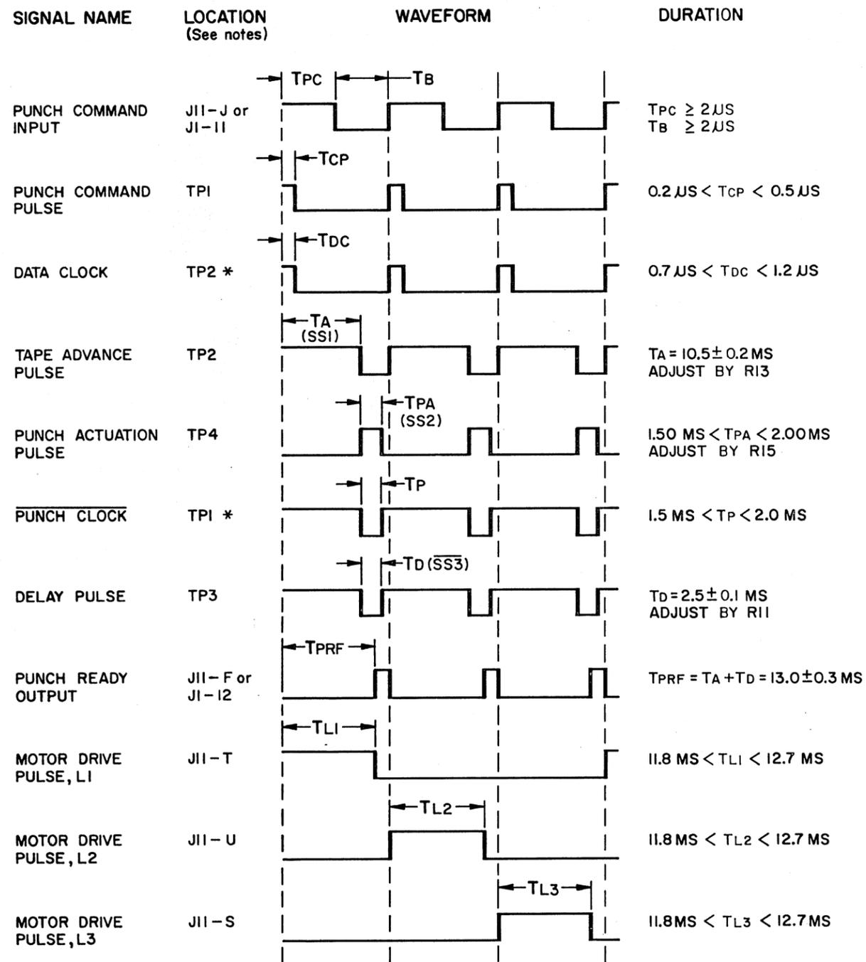
NOTES: 1. ALL LOCATIONS EXCEPT (\*) ARE ON CONTROL LOGIC AND FEED HOLE DRIVER CARD. LOCATIONS MARKED WITH (\*) ARE ON DATA LOGIC AND DRIVER CARD ALTHOUGH THESE SIGNALS ARE GENERATED ON THE CONTROL LOGIC AND FEED HOLE DRIVER CARD.
