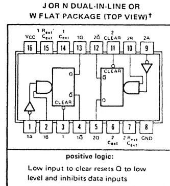
TTL/MONOSTABLE 9602 RETRIGGERABLE RESETTABLE MONOSTABLE MULTIVIBRATOR
