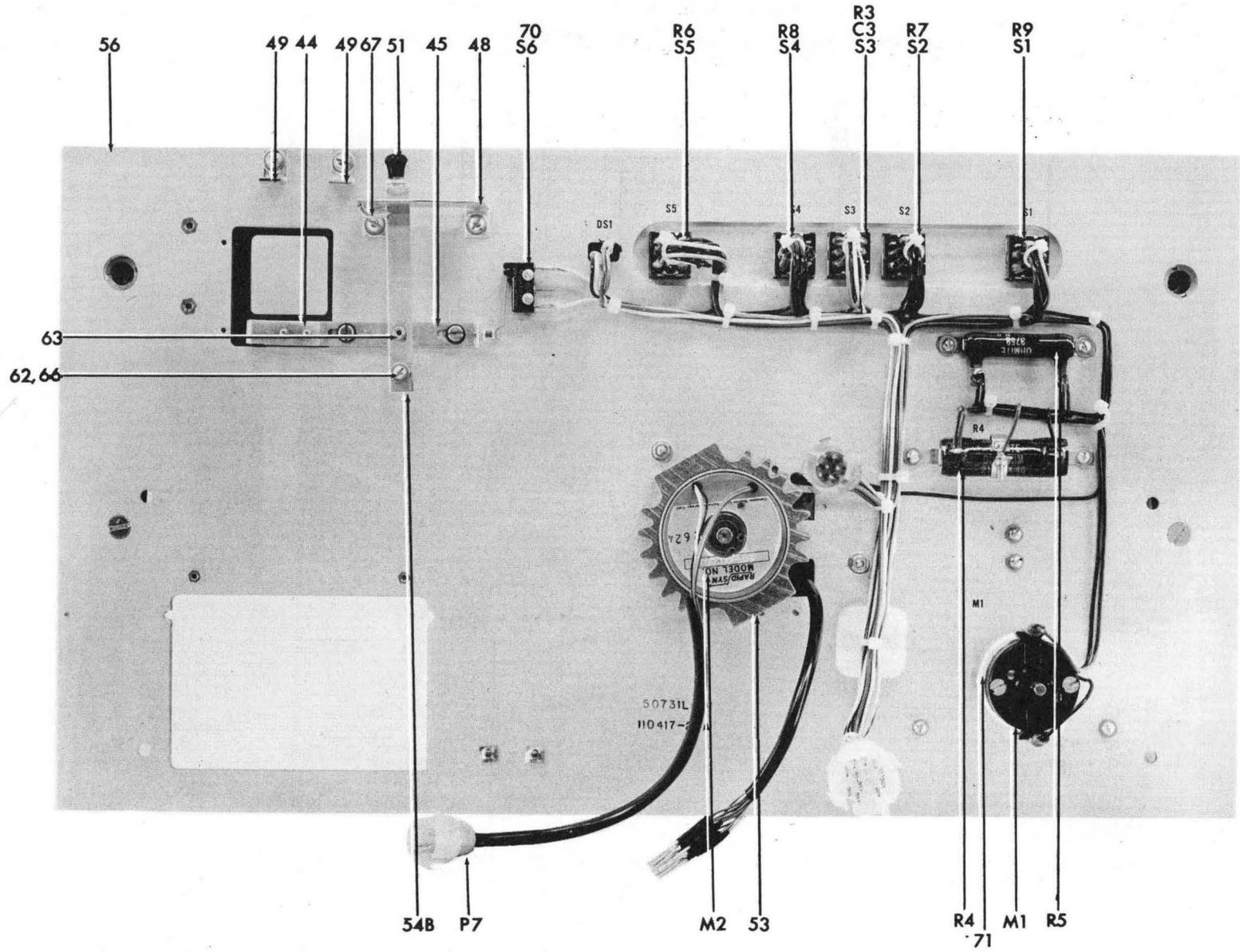
Figure 7-5. RDB3075BCX, Rear View of Front Panel
