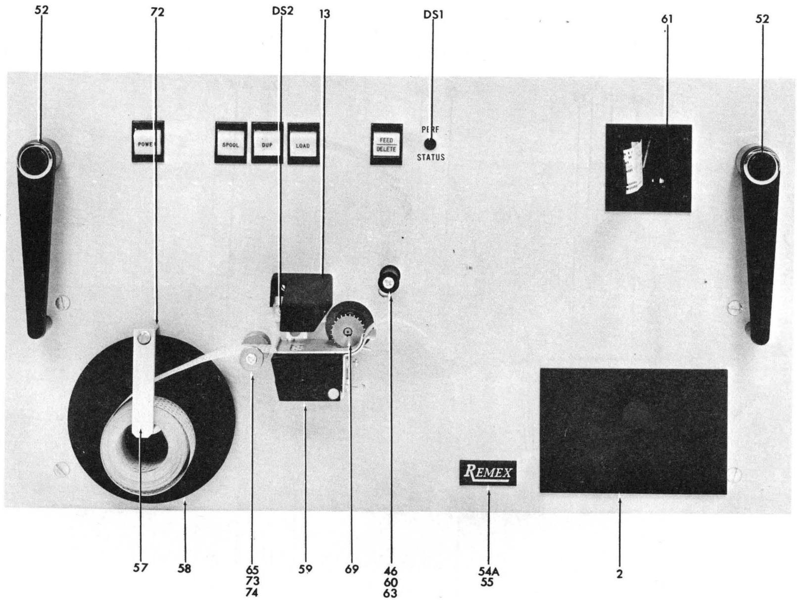
Figure 7-4. RDB3075BCX, Front View of Front Panel
