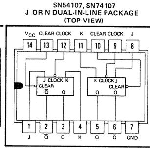
positive logic: Low input to clear sets Q to logical 0.
