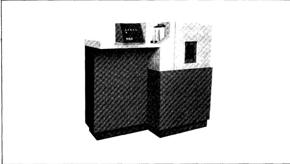
The RCA 8234 Card Punch is an 80-column, row-oriented card punch unit. It is capable of feeding, punching, and checking cards at a rate of up to 100 cards per minute. The 8234 contains an 80-byte storage buffer which provides temporary storage for punched data so that card punching operations can be performed independently of the processor.
