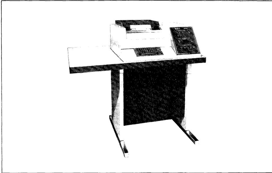
The Model 8097-020 is a free-standing, self-contained unit which provides control to enable system operation in conjunction with the operating system programs. The operator communicates with the system by way of a set of control switches and a console typewriter.
