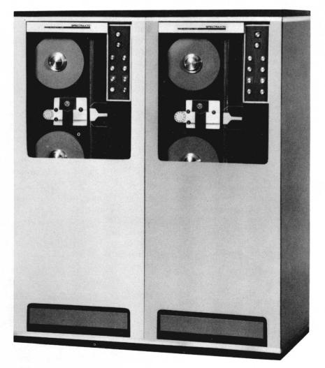
Figure 10. Model 70/432 Magnetic Tape Unit
