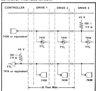
Figure 4. Recommended Controller Interface Circuit.
