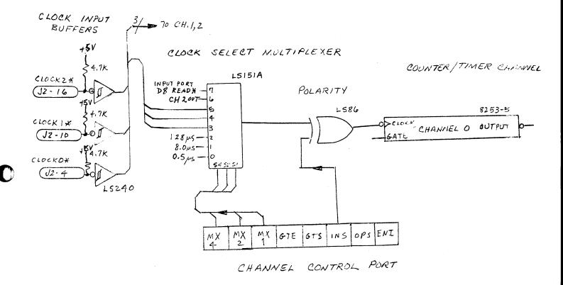
Figure 3-2-A Clock Control Circuit for Channel O (Typical of each channel.)
