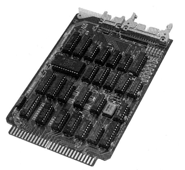
Figure 1-1. 7308 Multichannel Counter/Timer Card.
