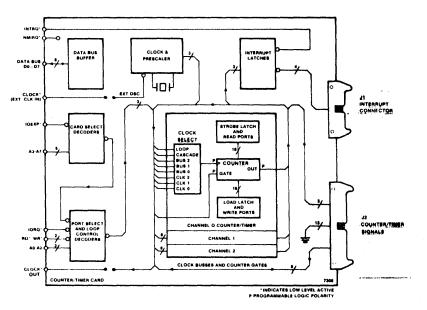
Figure 1-2. Block Diagram of 7308 Multichannel Counter/Timer Card.
