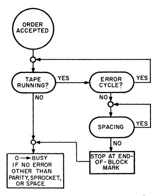
Figure TAC-6. Flowchart of Magnetic Tape Release Order
