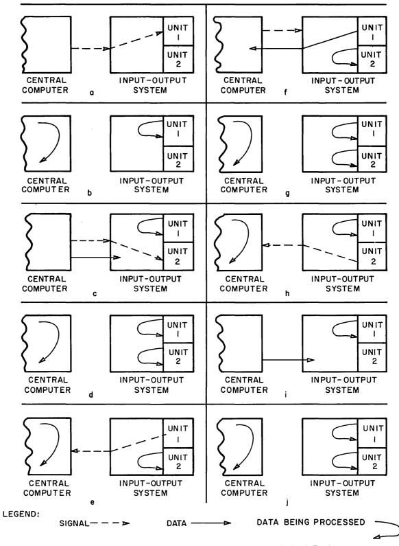
Figure INT-4. General Operation of the Input-Output System
