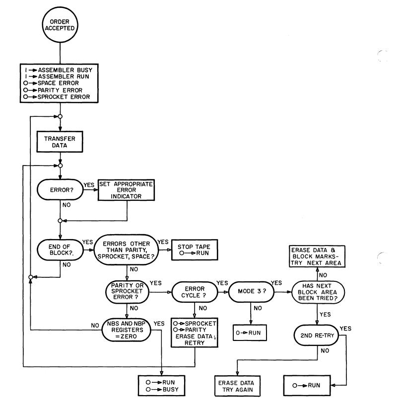
Figure TAC-4. Flowchart of Magnetic Tape Write Order
