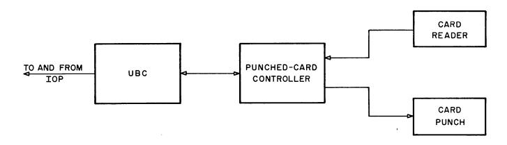
Figure PC-1. Tie-In of Punched-Card System with 2000 System
