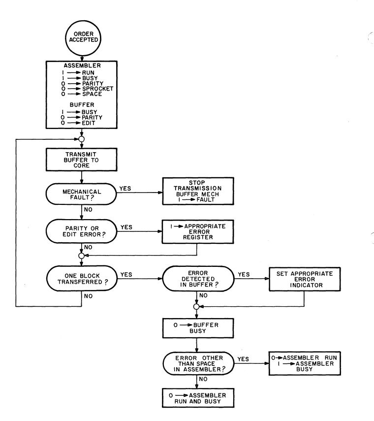
Figure TAC-12. Flowchart of On-Line I-O Order, Buffer to Core
