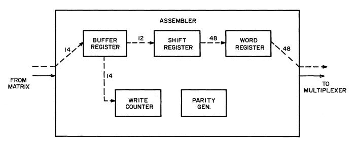
Figure IOP-4. Data Flow in Assembler During Input Order
