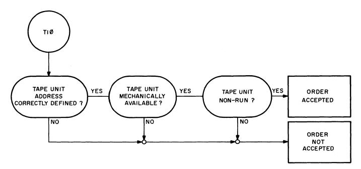
Figure IOP-9. Flowchart of Class D Magnetic Tape Order Acceptance
