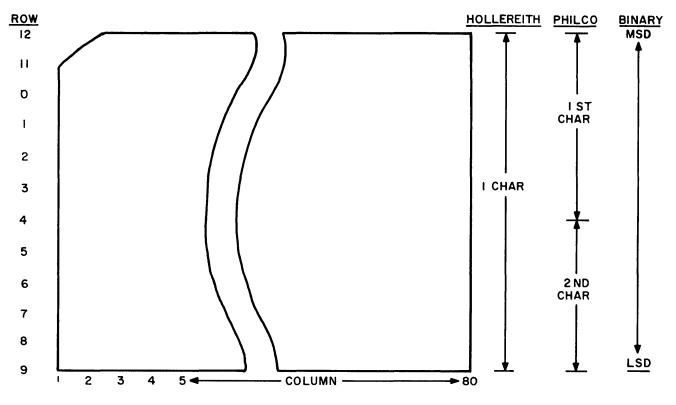
Figure PC-2. Punched-Card Format
