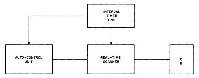
Figure RT-1. Real-Time System, Simplified Block Diagram
