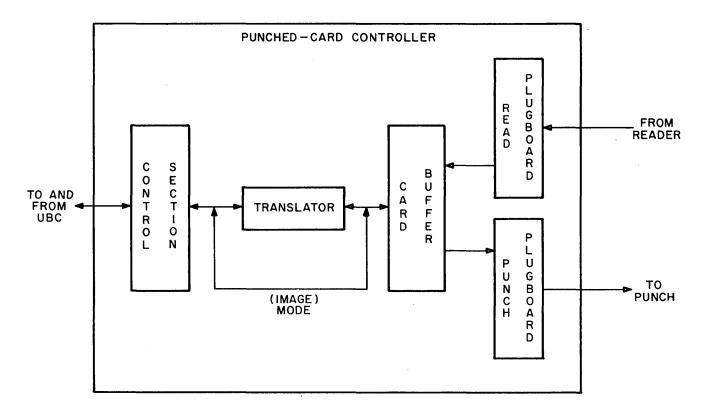
Figure PC-3. Principal Components of Punched-Card Controller
