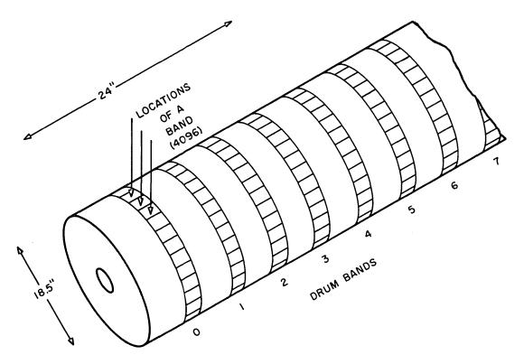
Figure DR-1. Simplified Drawing of Drum Showing Drum Bands and Data Locations of These Bands
