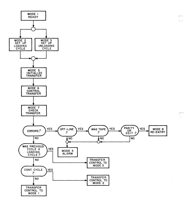
Figure UBC-3. Flowchart of UBC Operating Modes
