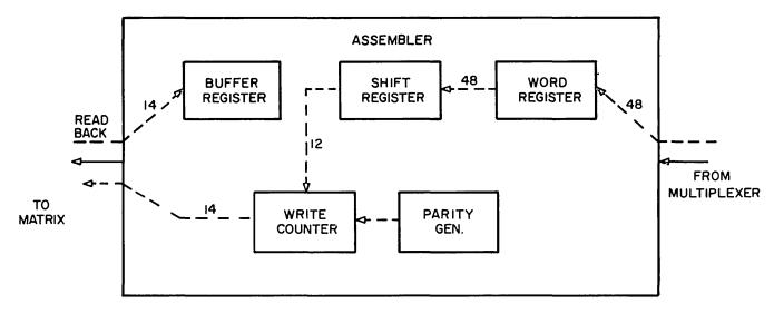
Figure IOP-5. Data Flow in Assembler During Output Order
