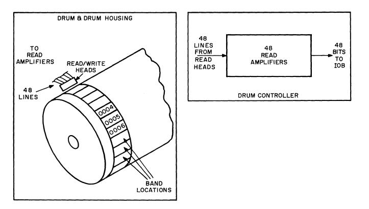
Figure DR-4. Data Flow During Reading Operation
