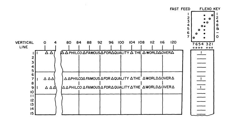
Figure PR-3. Use of Printer Layout Sheet
