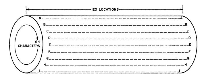
Figure PR-5. Print Roll of High-Speed Printer
