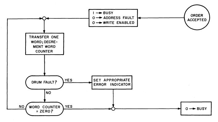
Figure TAC-16. Flowchart of I-O Order, Core to Drum
