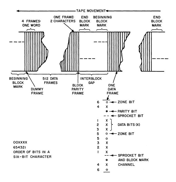
Figure MT-2. Magnetic Tape Format
