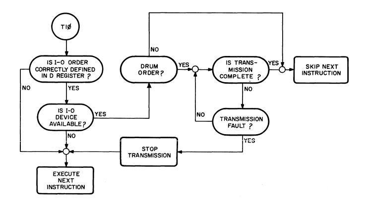
Figure INT-3. Flowchart of the Operations Performed Following the Execution of the TIO Instruction.
