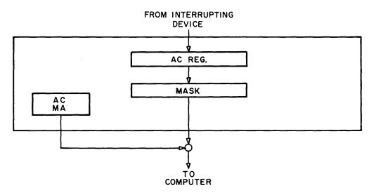
Figure RT-2. Registers of Auto-Control Unit
