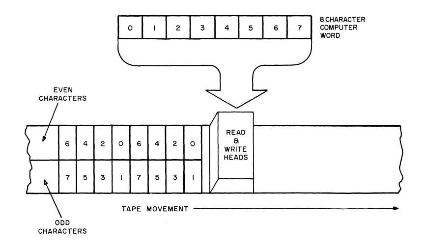
Figure MT-3. Arrangement of Characters on Tape
