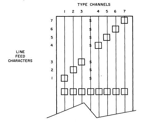
Figure PR-1. Vertical Format Tape Loop
