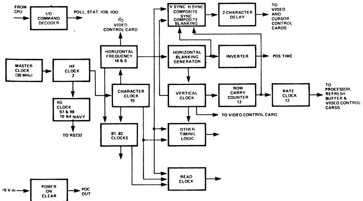
Figure 4-9. Timing control card block diagram.
