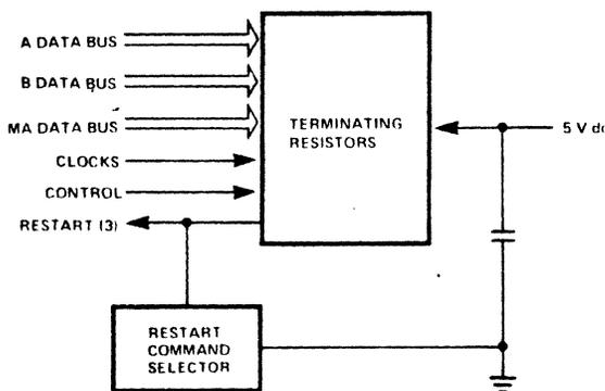
Figure 4-23. Terminator card block diagram.
