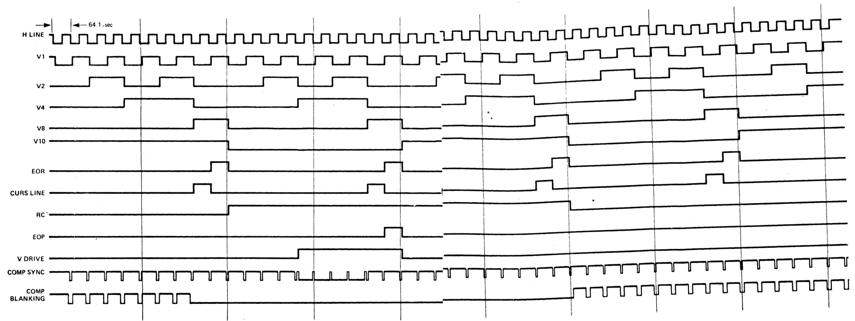
Figure 4-11b. Timing control card timing diagram.
