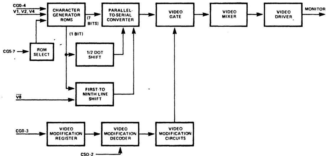
Figure 4-20. Video control card block diagram.
