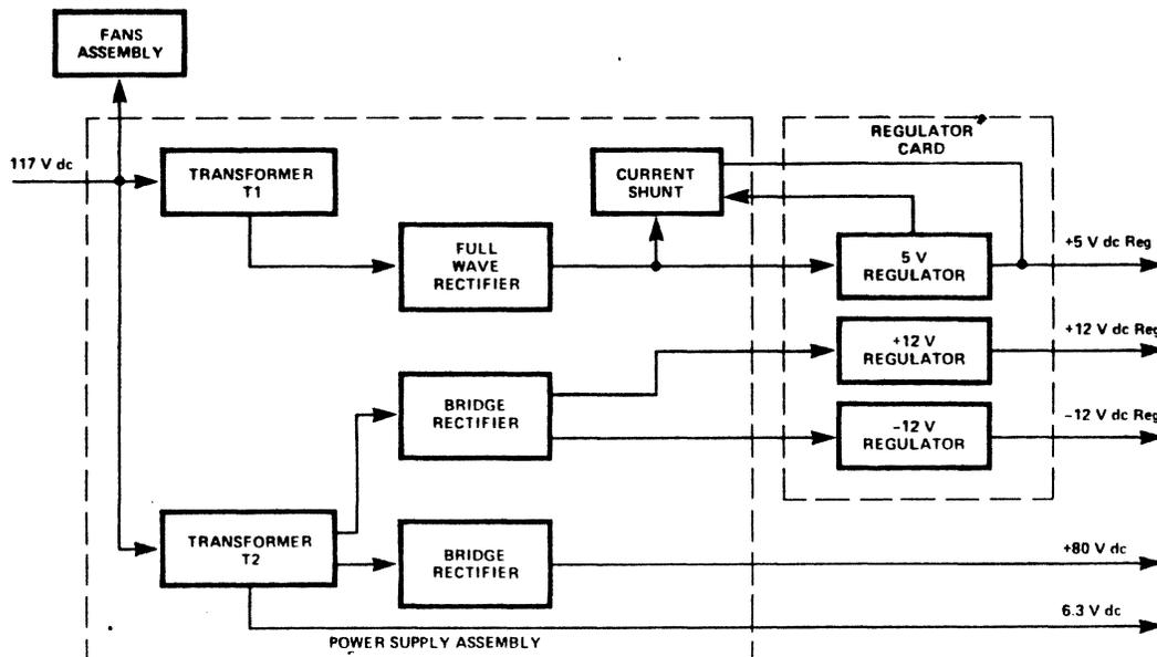
Figure 4-6. Power supply block diagram.
