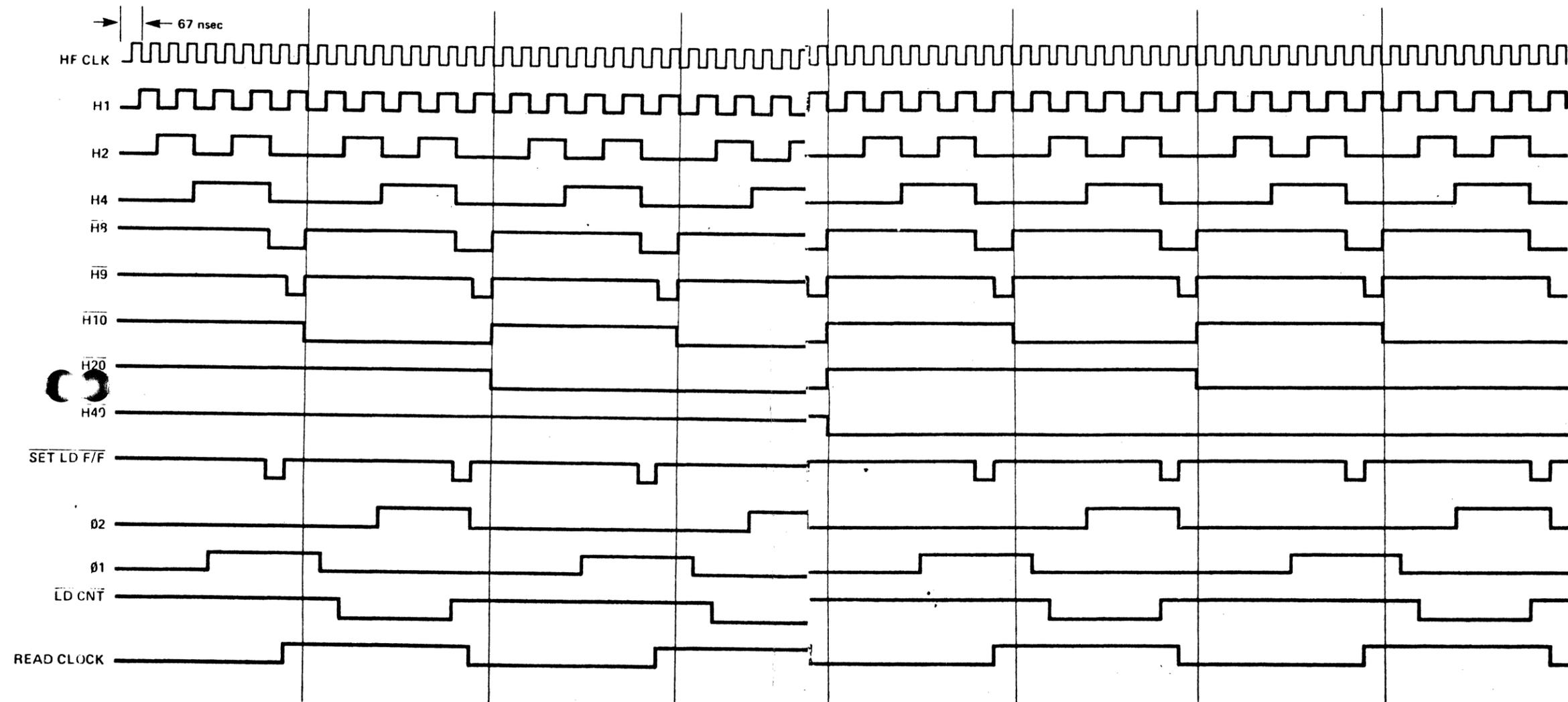
Figure 4-10. Timing control card timing diagram.
