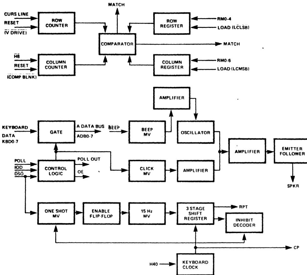
Figure 4-19. Cursor control card block diagram.
