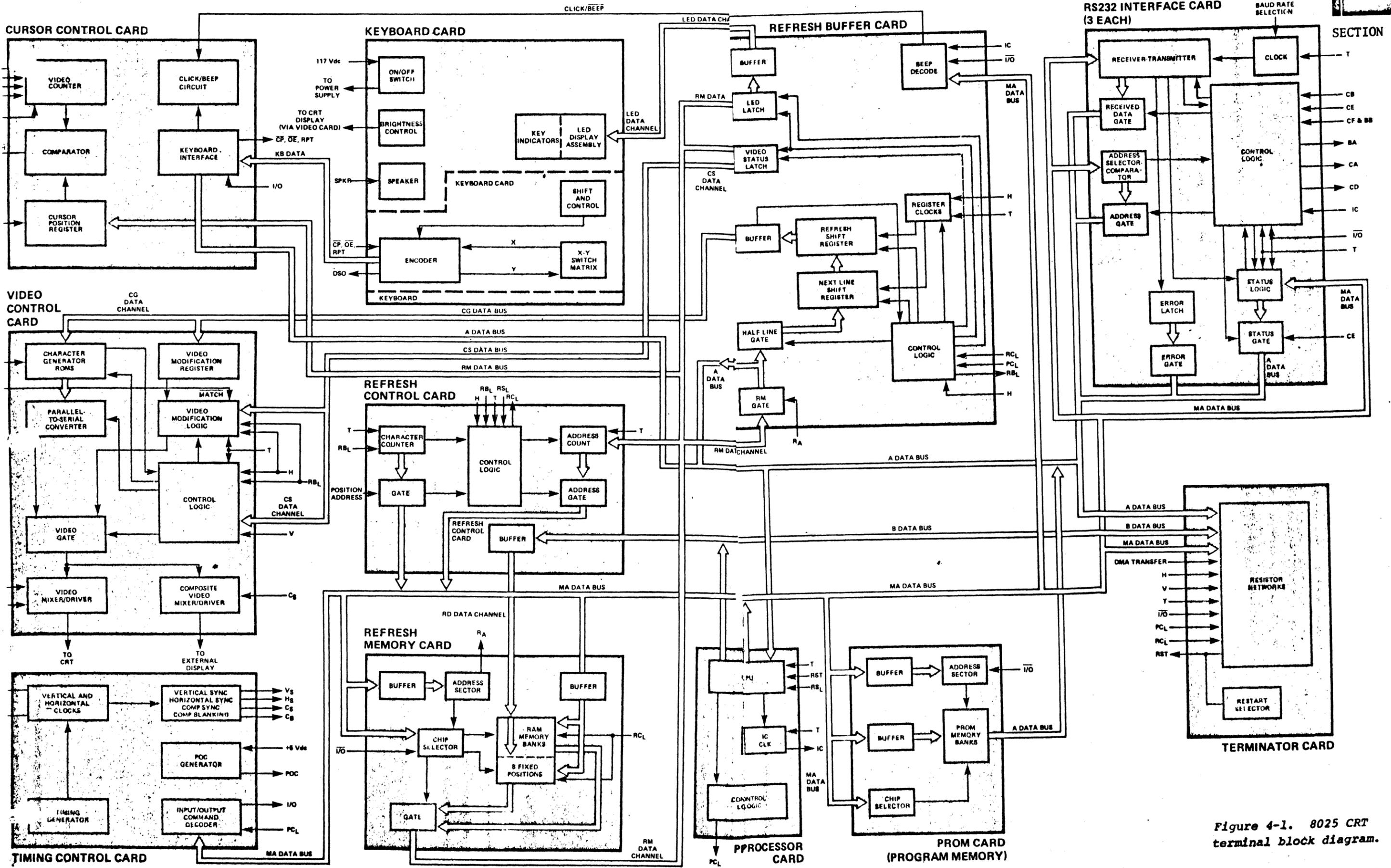
Figure 4-1. 8025 CRT terminal block diagram.
