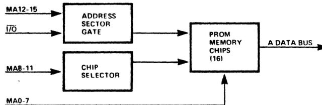
Figure 4-14. Buffered PROM card block diagram.
