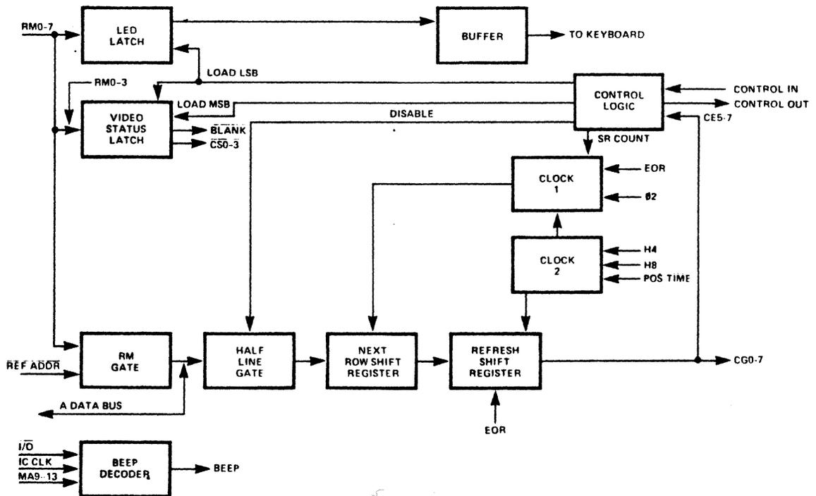
Figure 4-16. Refresh buffer card block diagram.
