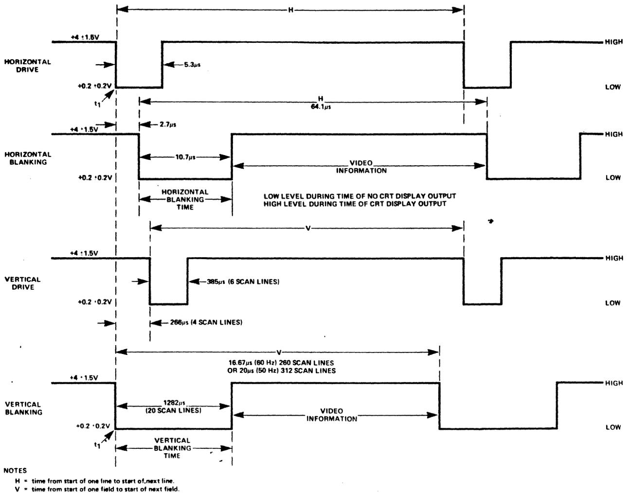
Figure 4-8. CRT waveforms.
