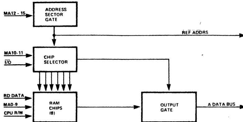
Figure 4-15. Buffered RAM memory card block diagram.
