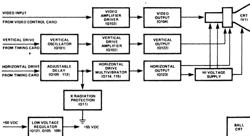
Figure 4-7. CRT display block diagram.
