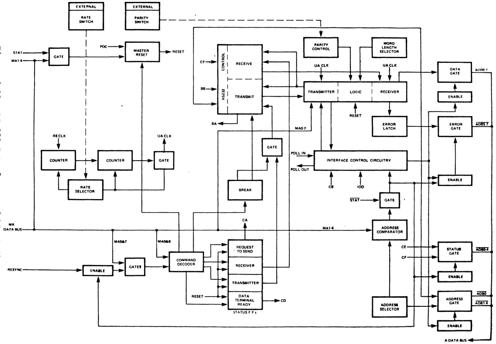
Figure 4-22. RS-232 Interface card block diagram.
