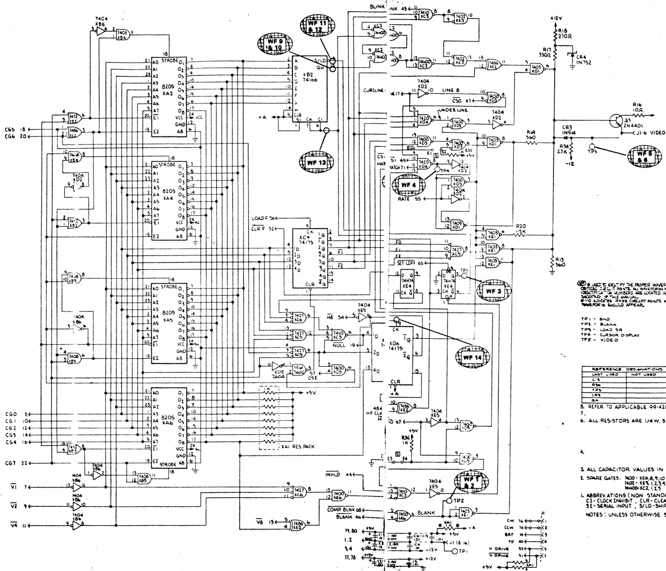
⊗ USED TO IDENTIFY THE PROPER WAVEFORM FOR SPECIFIC CIRCUIT POINTS. ALL WAVEFORMS WITH COMMON IDENTIFICATION NUMBERS ARE LOCATED IN SECTION 6, TROUBLESHOOTING OF THIS MANUAL. ⊗ INDICATES OTHER CIRCUIT POINTS WHERE THE SAME WAVEFORM SHOULD APPEAR.
