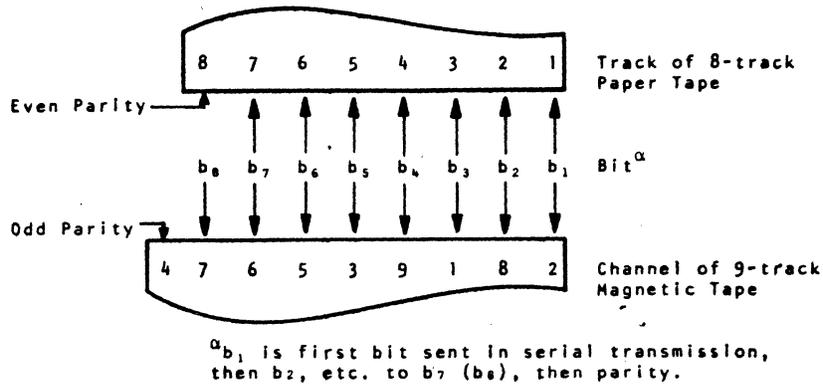
Figure 10-1. Tape track assignments for ISO/ASCII codes.
