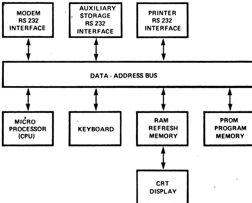
Figure 1-4. 8025 CRT terminal, simplified block diagram.
