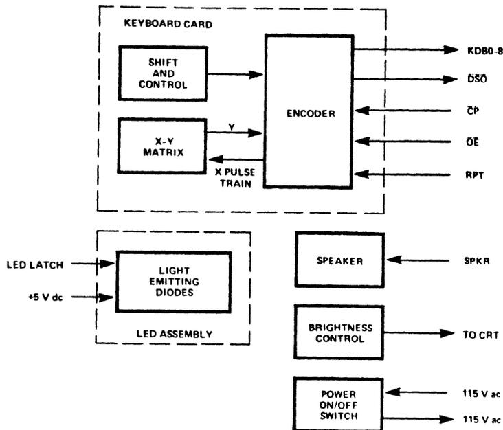
Figure 4-21. Keyboard block diagram.
