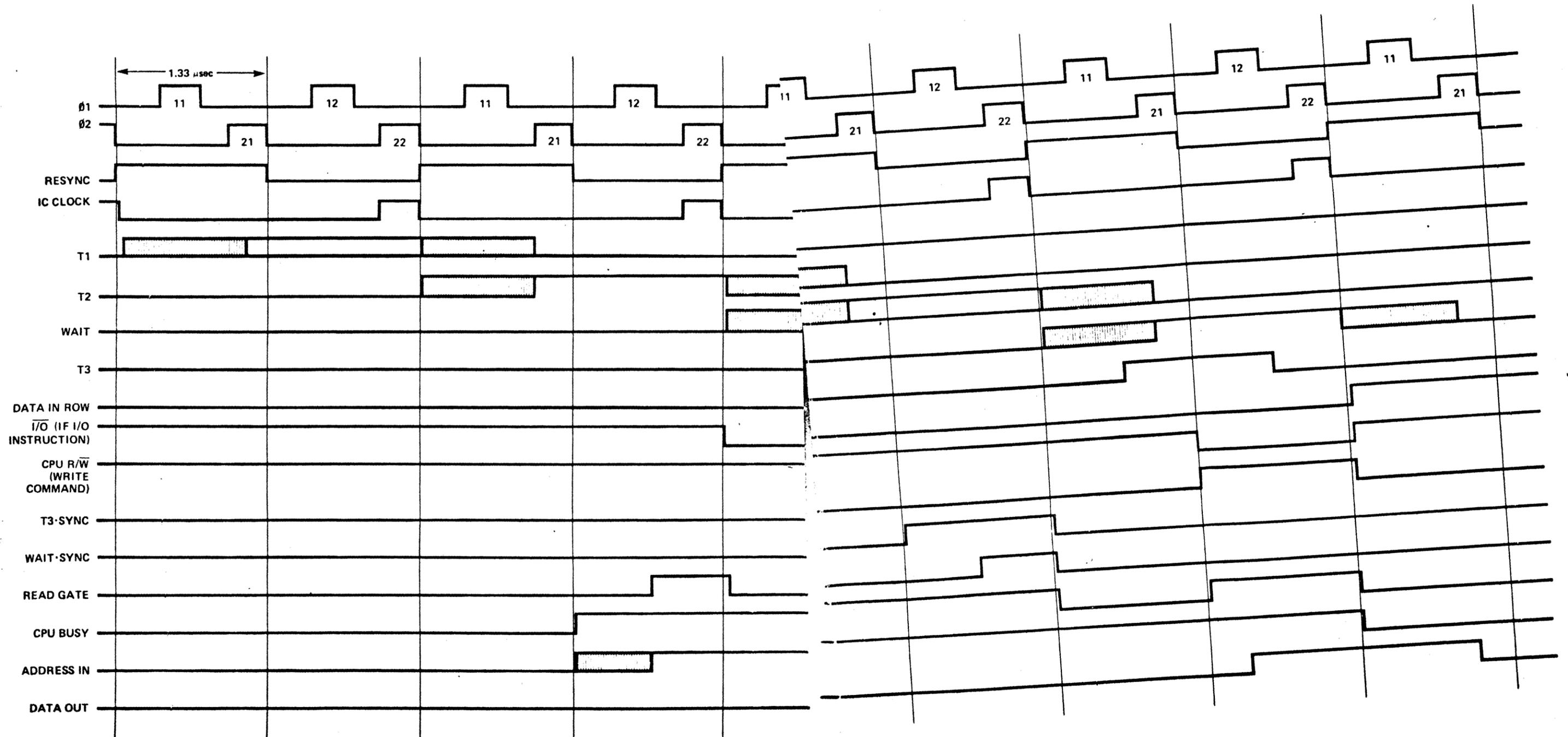
Figure 4-13. Processor card (CPU) timing diagram.
