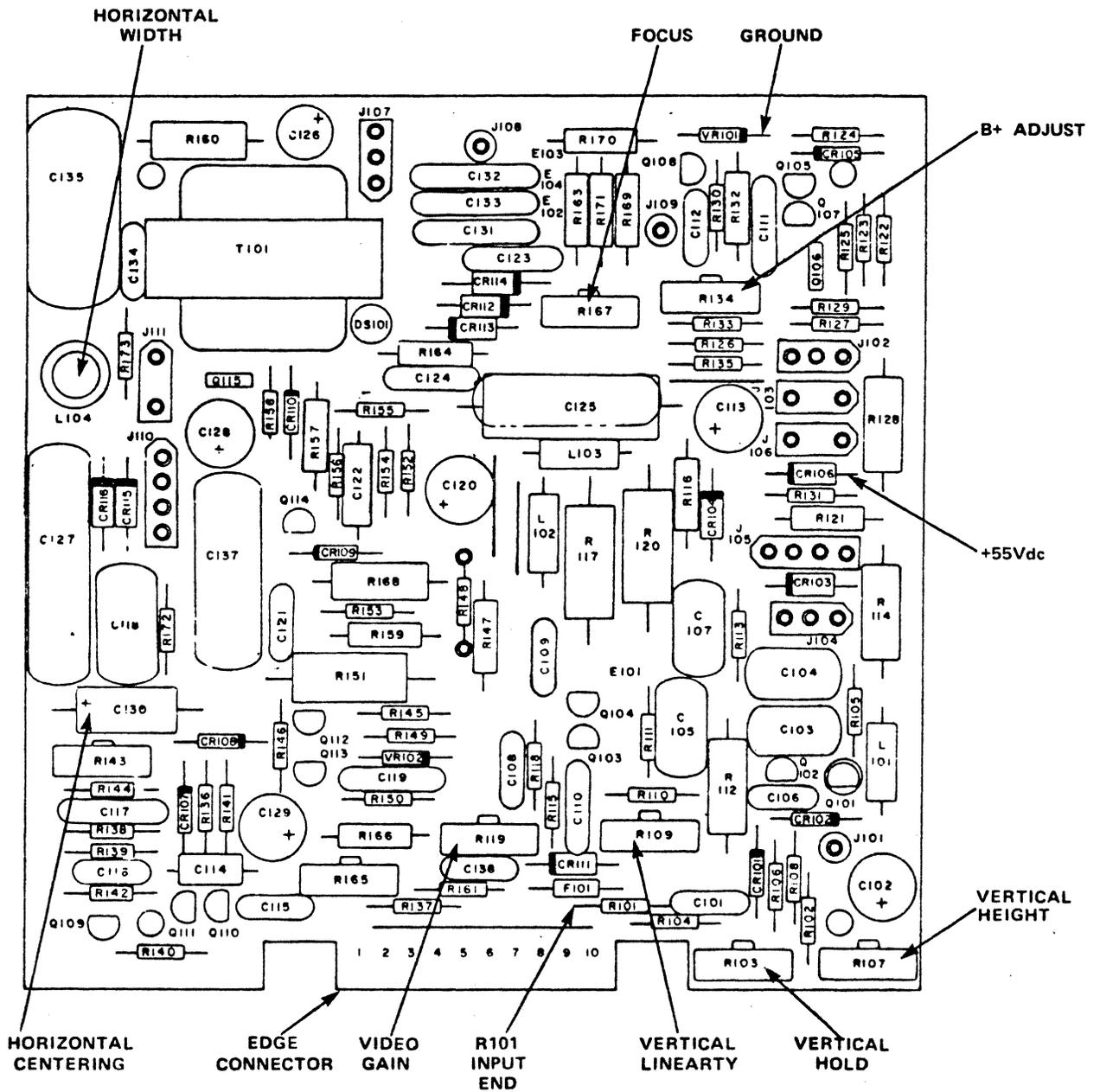
Figure 7-4. Monitor Deflection Card: CRT adjustment and "test point" locations.
