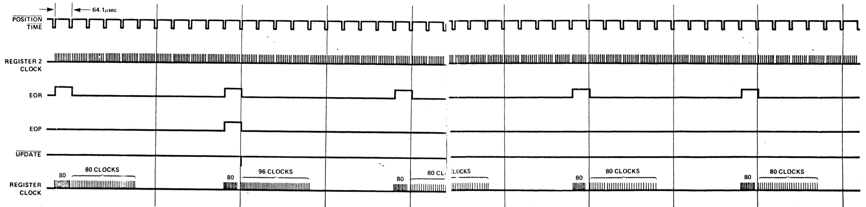
Figure 4-17b. Refresh buffer/control card timing diagram.
