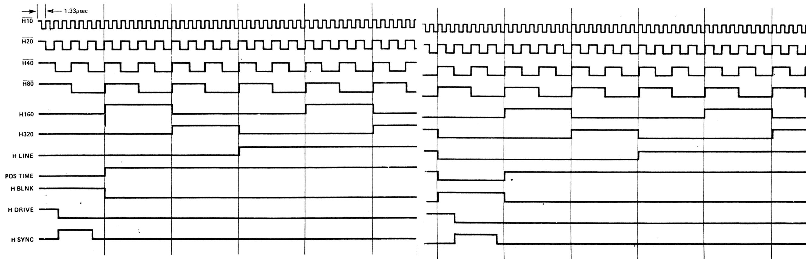
Figure 4-11a. Timing control card timing diagram.
