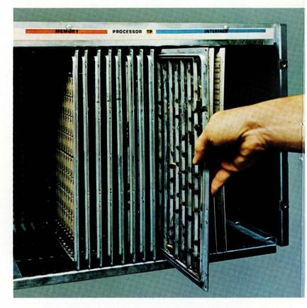
High speed, proven reliability and modularity are the keywords that describe the NCR 399 modular core memory. The memory of the basic system can be expanded in 2K increments up to 16K bytes, and in 4K increments from 16K to 32K, in your office as your requirements increase. It's no longer necessary to buy larger equipment that you really need to allow for growth or to have to change equipment when growth is more rapid than anticipated. An NCR 399 can grow as you grow.
