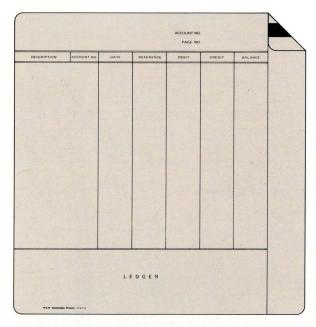
Hard copy records have always been the foundation of accounting systems. The NCR 399 builds upon this foundation by providing this fundamental accounting record in a conventional readable form in combination with electronically encoded information on a magnetic stripe on the back of each ledger. This combination offers the advantage of random access to current and historical data.
