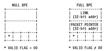
If the envelope is full, the packet pointer field contains a valid pointer. The length is fixed at 32 bits and is a pointer to a command packet data structure.
