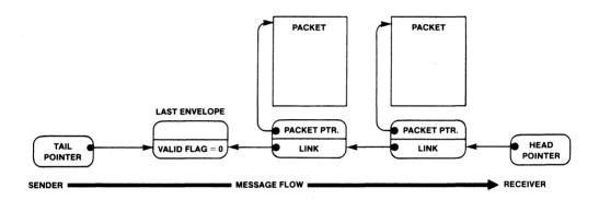
The BPP does not define how the pipes are physically implemented, except that they must reside in a region of RAM shared between the communicating processors. Also, the system design must provide some means for the host processor to transmit the initial TAIL and HEAD pointers to the slave processor when a new queue is established.
