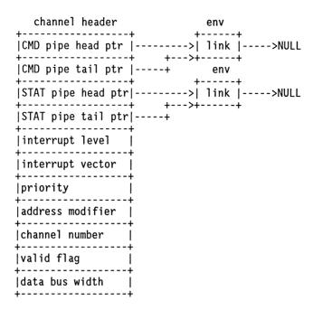
The rest of the fields in the channel header are initialized with the appropriate values, except for the valid flag and the channel number. The channel number and valid flag are set by the MVME327A at the successful completion of the create channel command.
