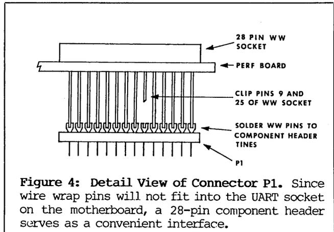
Figure 4: Detail View of Connector P1. Since wire wrap pins will not fit into the UART socket on the motherboard, a 28-pin component header serves as a convenient interface.
