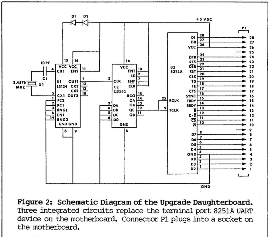
**Figure 2: Schematic Diagram of the Upgrade Daughterboard.** Three integrated circuits replace the terminal port 8251A UART device on the motherboard. Connector P1 plugs into a socket on the motherboard.
