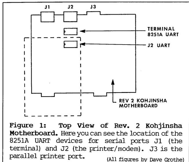
**Figure 1: Top View of Rev. 2 Kohjinsha Motherboard.** Here you can see the location of the 8251A UART devices for serial ports J1 (the terminal) and J2 (the printer/modem). J3 is the parallel printer port. (All figures by Dave Grothe)
