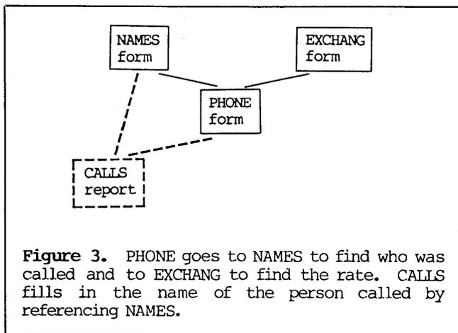
**Figure 3.** PHONE goes to NAMES to find who was called and to EXCHANG to find the rate. CALLS fills in the name of the person called by referencing NAMES.
