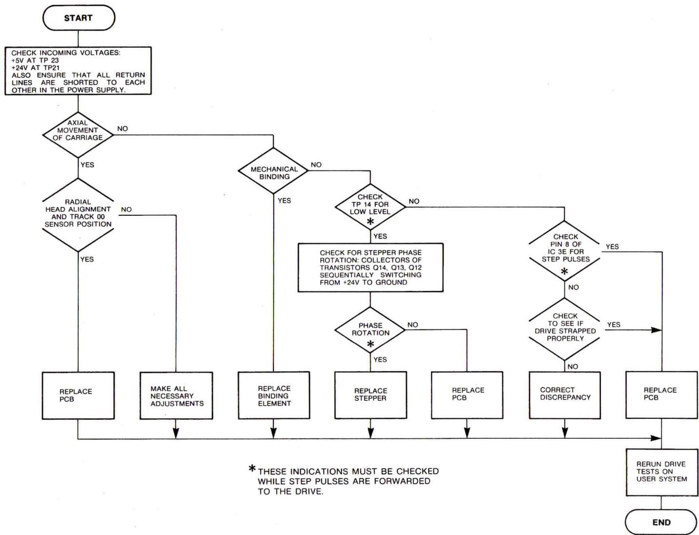
FIGURE 4-21. HEAD POSITION ACTUATOR DIAGNOSTIC FLOWCHART
