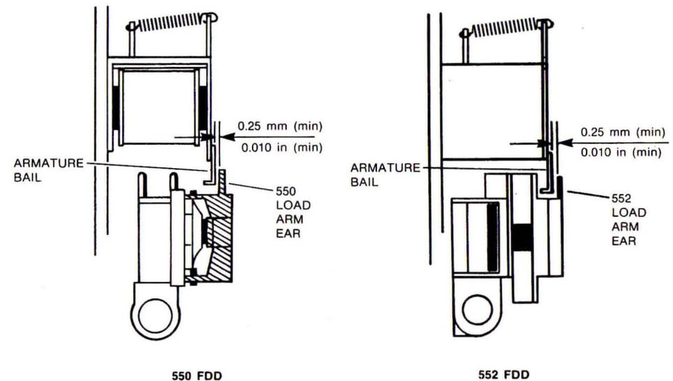
FIGURE 4-15. BAIL AND LOAD ARM CLEARANCE
