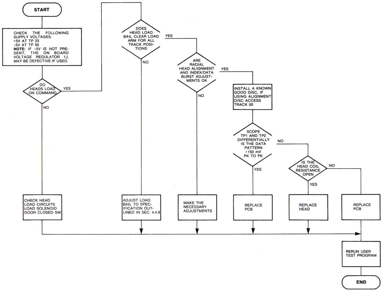
FIGURE 4-22. READ CIRCUIT DIAGNOSTIC FLOWCHART
