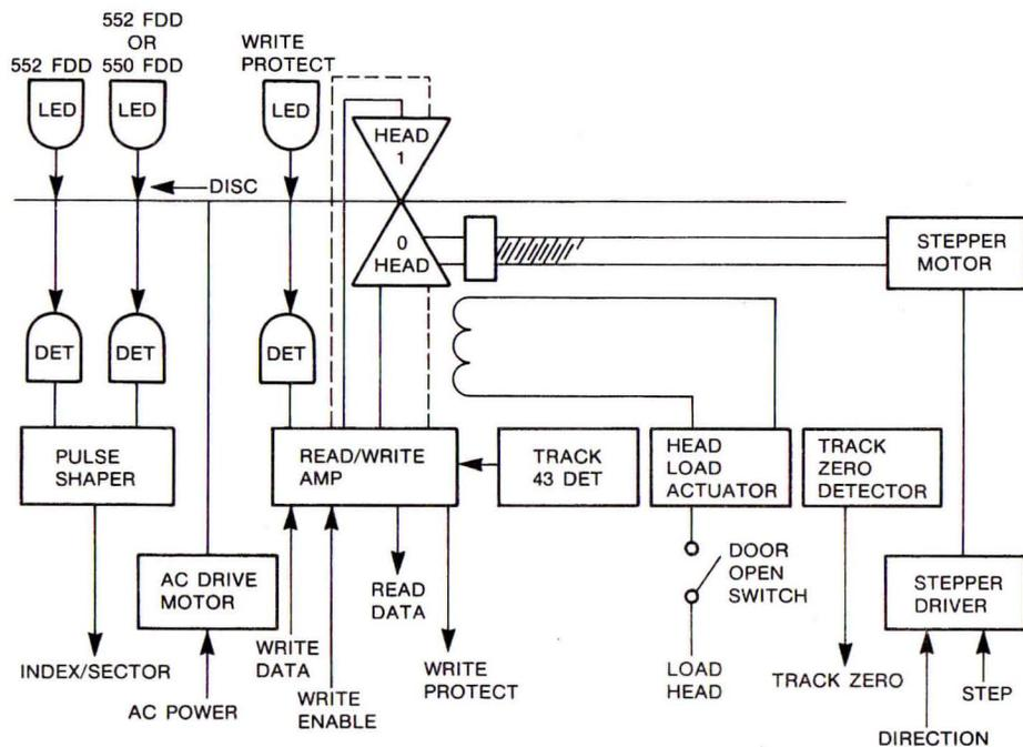
FIGURE 4-10. PCB FUNCTIONAL BLOCK DIAGRAM
