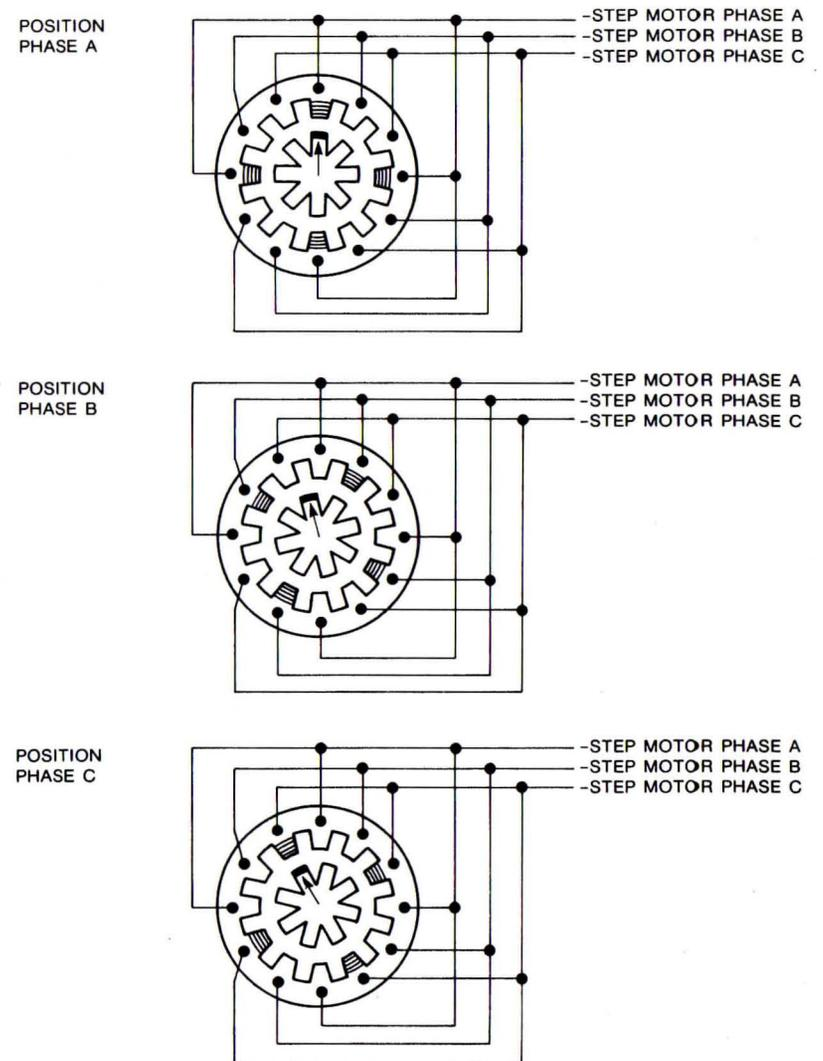
FIGURE 2-2. STEPPER MOTOR PHASE WINDINGS
