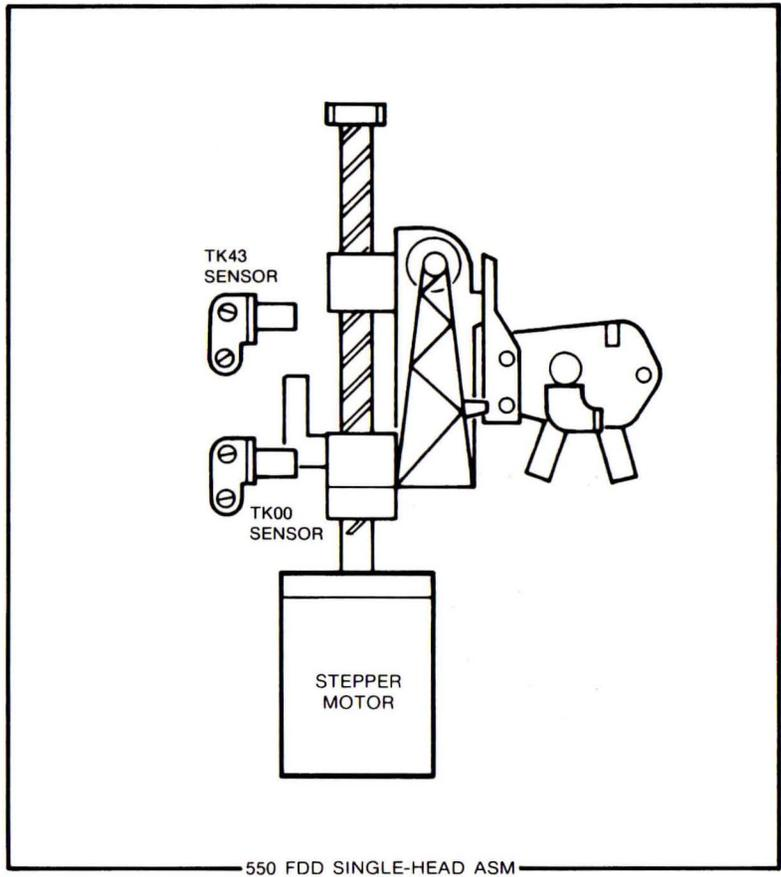
FIGURE 1-2. 550/552 FLEXIBLE DISC DRIVE FUNCTIONAL DIAGRAM (Part 2 of 2)
