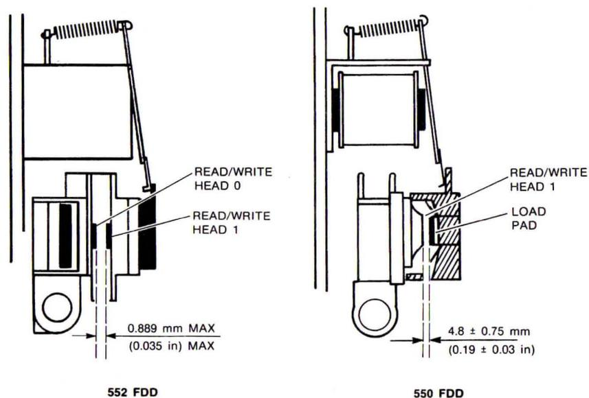
FIGURE 4-16. READ/WRITE HEAD AND LOAD PAD CLEARANCE
