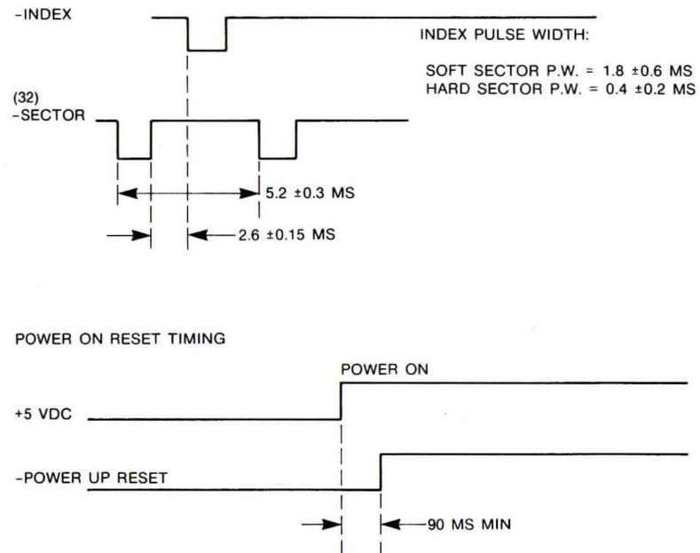
FIGURE 2-11. INDEX/SECTOR TIMING AND POWER UP RESET TIMING
