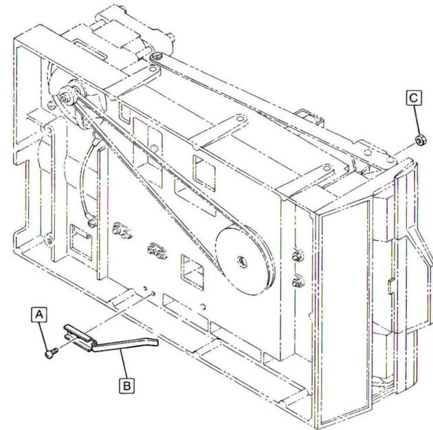
FIGURE 4-9. EJECT SPRINGS REMOVAL AND REPLACEMENT
