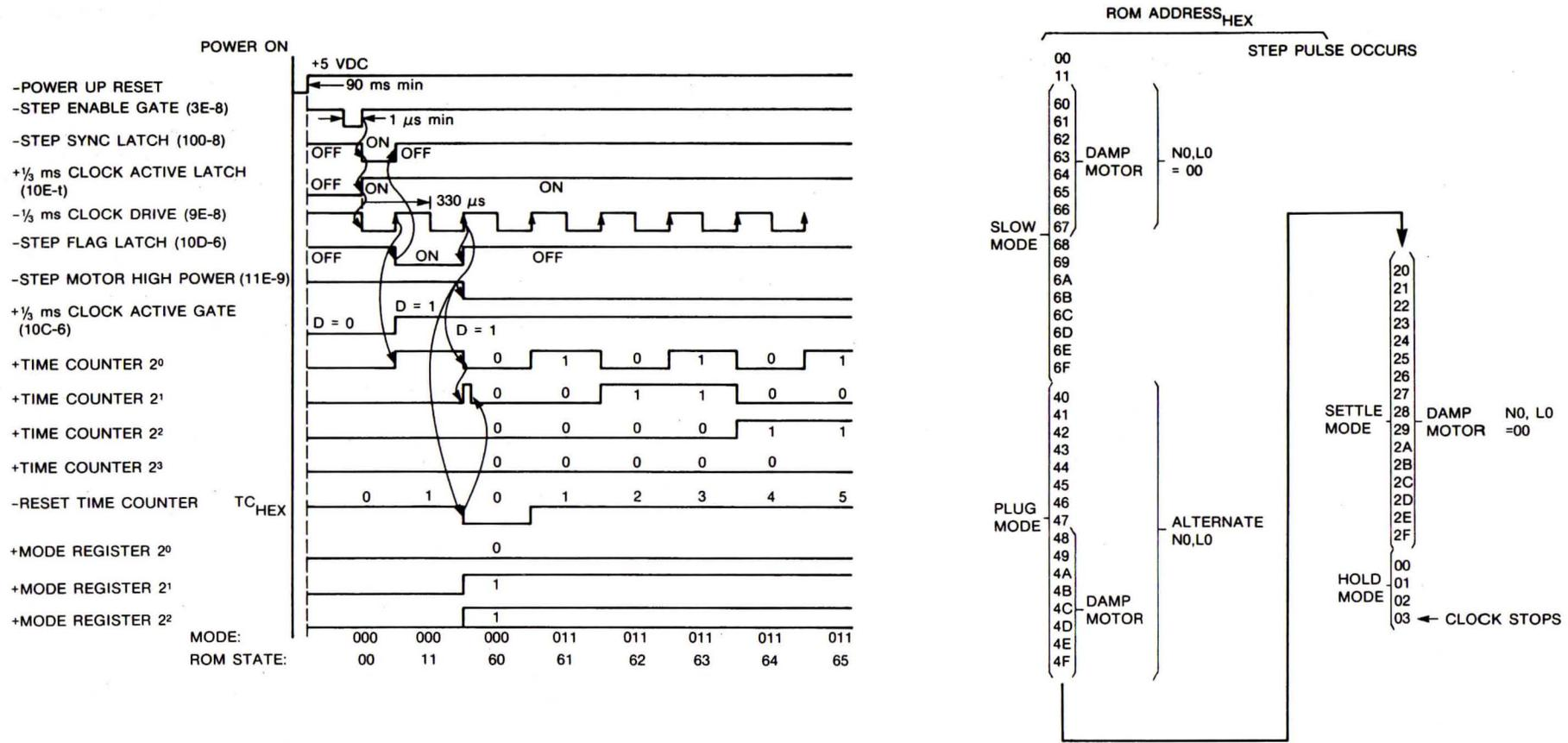
FIGURE 2-5. STEP SYNCHRONIZATION TIMING AND ONE STEP ROM SEQUENCE
