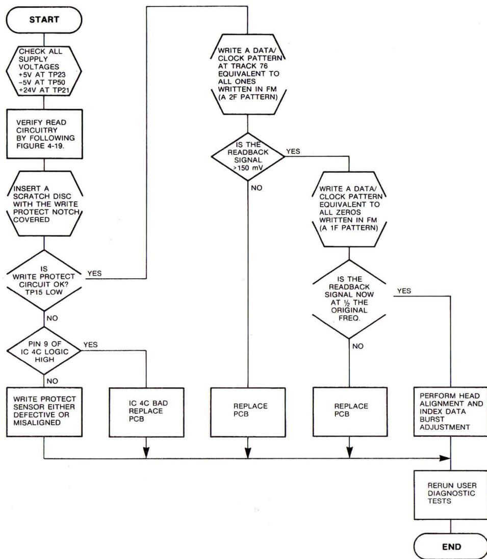
FIGURE 4-23. WRITE CIRCUIT DIAGNOSTIC FLOWCHART
