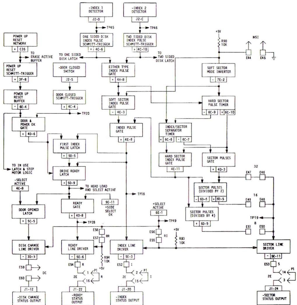
FIGURE 6-4. DISC LOAD, READY, INDEX AND SECTOR FUNCTIONS
