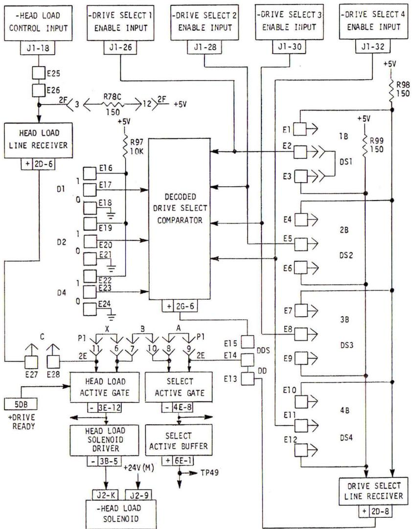
FIGURE 6-1. HEAD LOAD AND DRIVE SELECT FUNCTIONS
