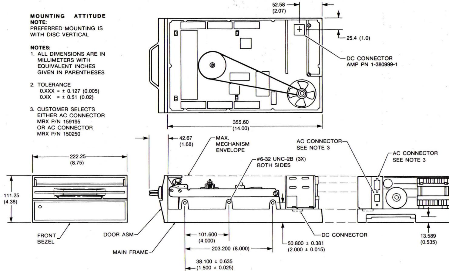
FIGURE 1-1. 550/552 FLEXIBLE DISC DRIVE MOUNTING AND AC PLUG INFORMATION
