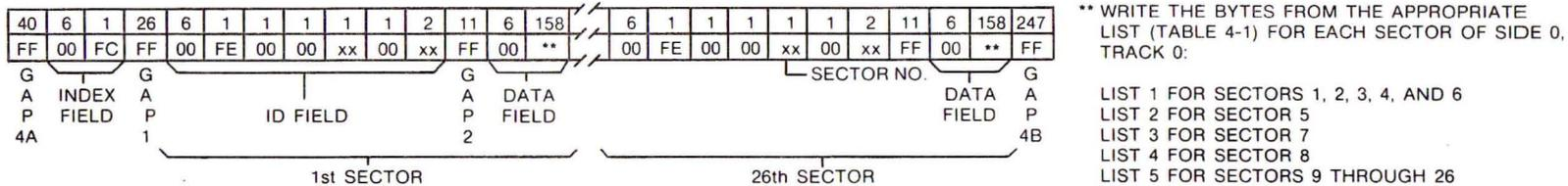
**FIGURE 5-3. IBM TWO-SIDED, 26-SECTOR (256-BYTE RECORD) FORMAT**
