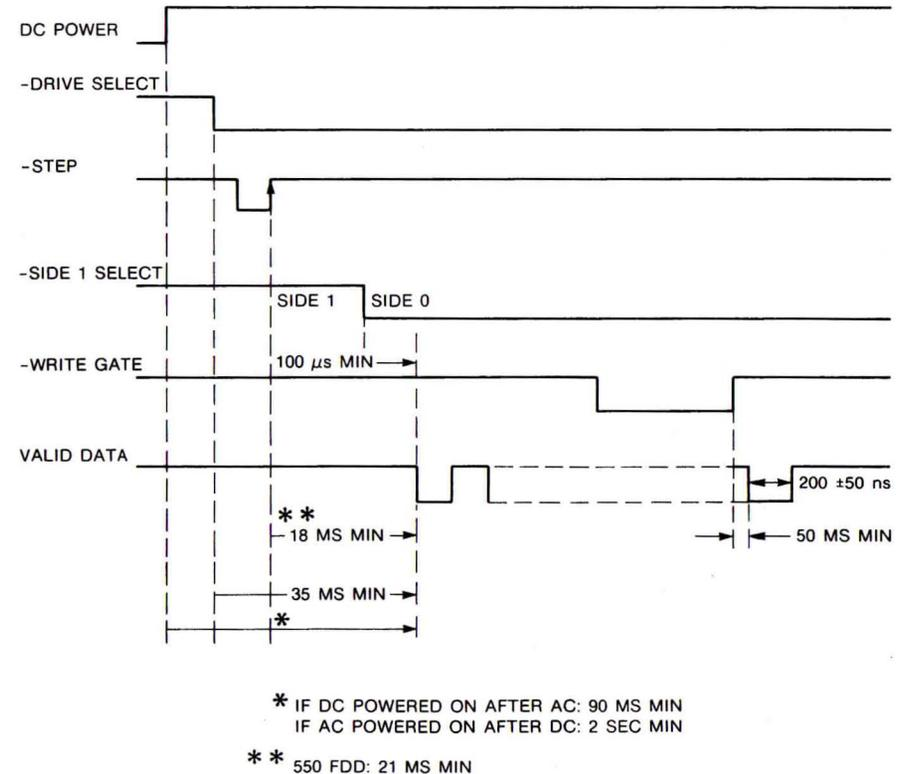
FIGURE 2-6. 552 FLEXIBLE DISC DRIVE SIDE SELECT TIMING
