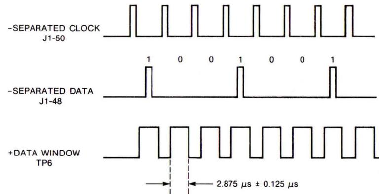
FIGURE 4-20. TP6 OUTPUT (+DATA WINDOW)
