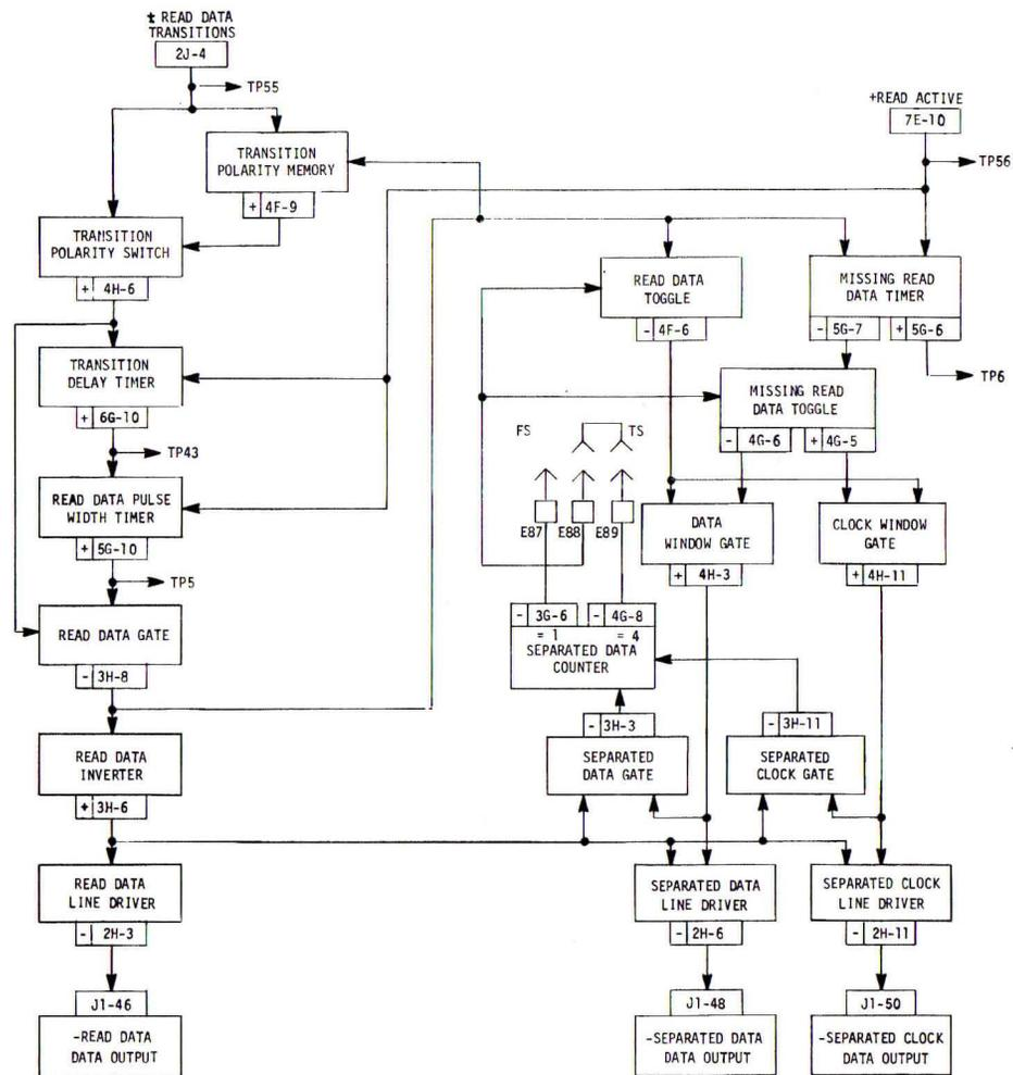
FIGURE 6-8. READ DATA OUTPUT FUNCTION
