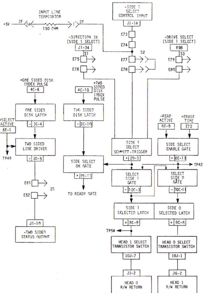
FIGURE 6-3. DISC TYPE AND SIDE SELECT FUNCTIONS
