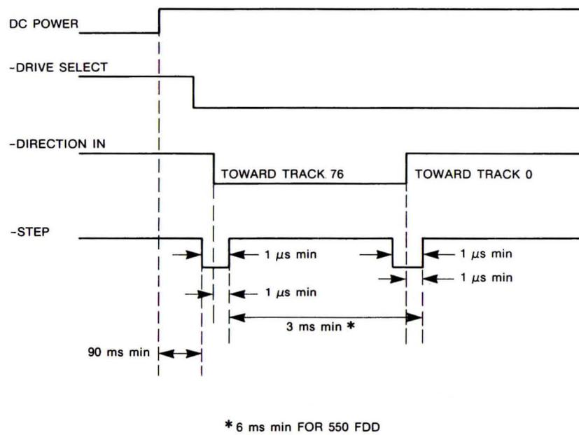
FIGURE 2-1. TRACK ACCESS TIMING
