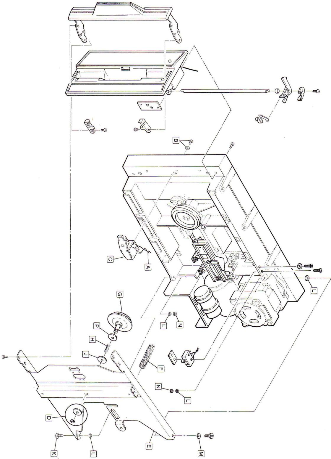
**FIGURE 4-5. PROGRAM CONTROLLED DOOR LOCK, CLAMP, AND CARRIER ASSEMBLY REMOVAL AND REPLACEMENT**
