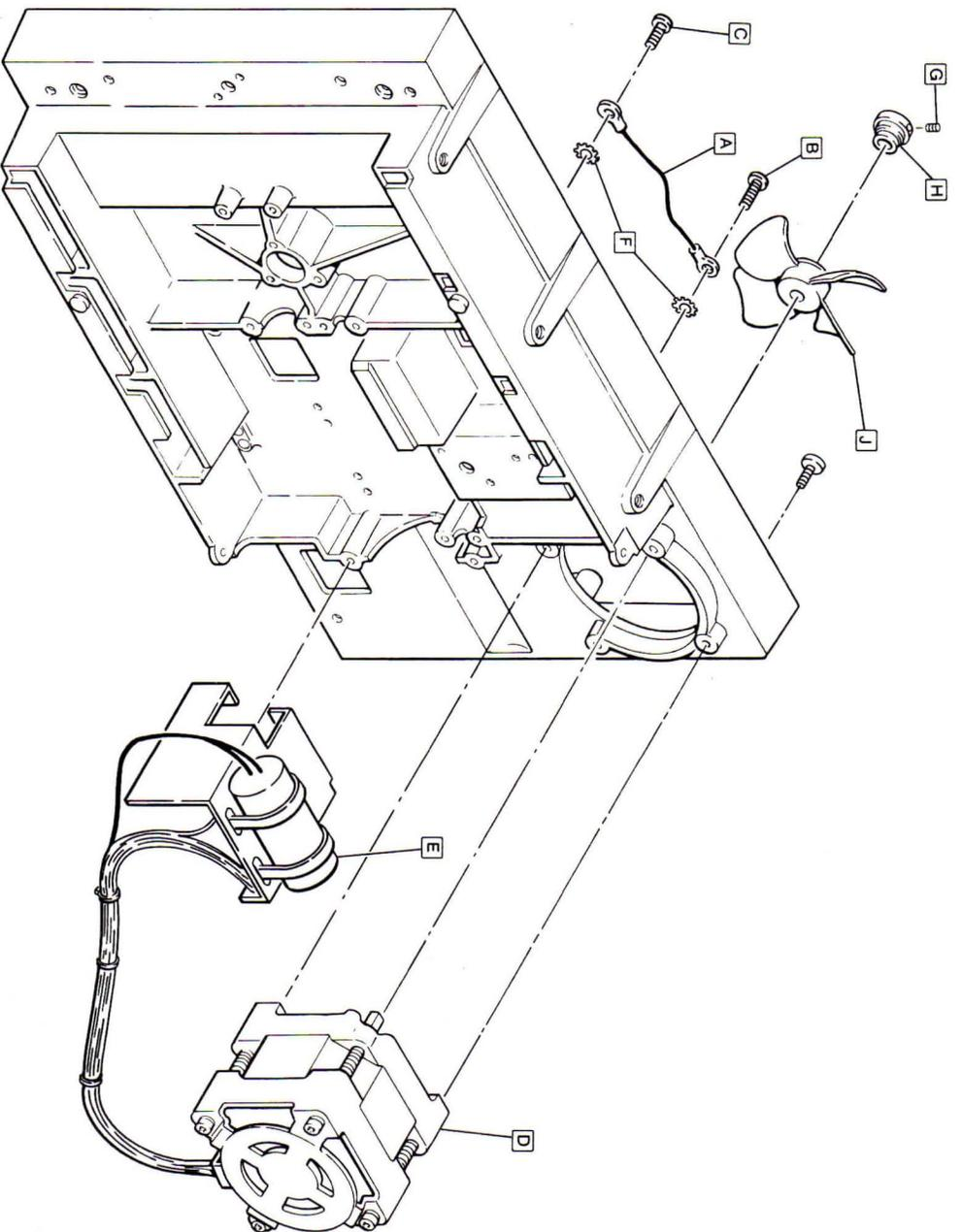
FIGURE 4-7. DRIVE MOTOR CAPACITOR, DRIVE PULLEY AND FAN ASSEMBLY REMOVAL AND REPLACEMENT
