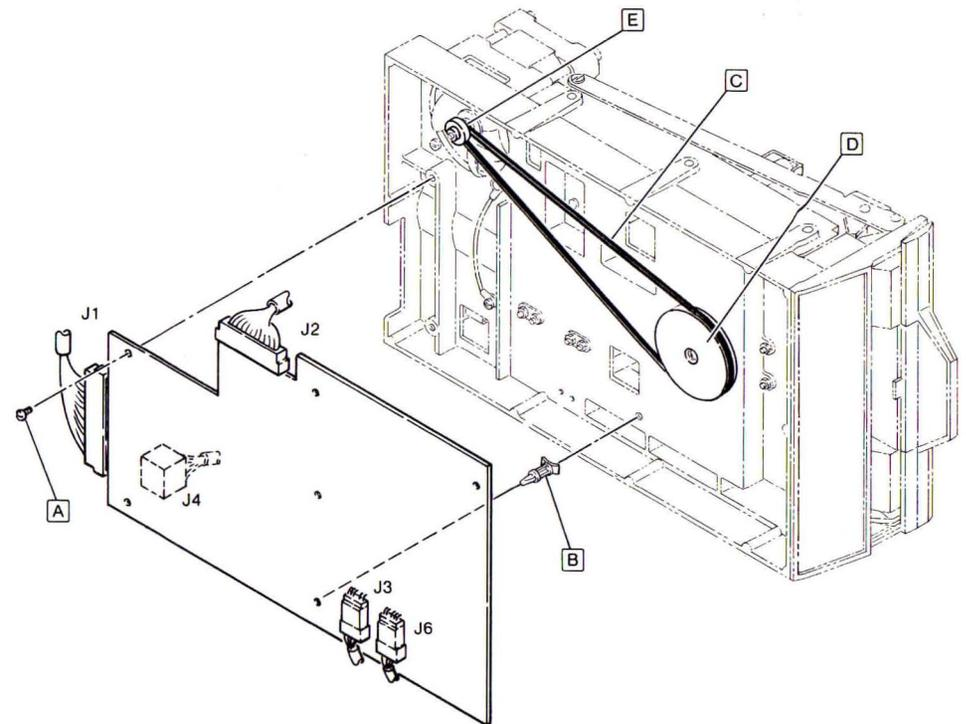
FIGURE 4-2. PRINTED CIRCUIT BOARD (PCB) AND DRIVE BELT REMOVAL AND REPLACEMENT
