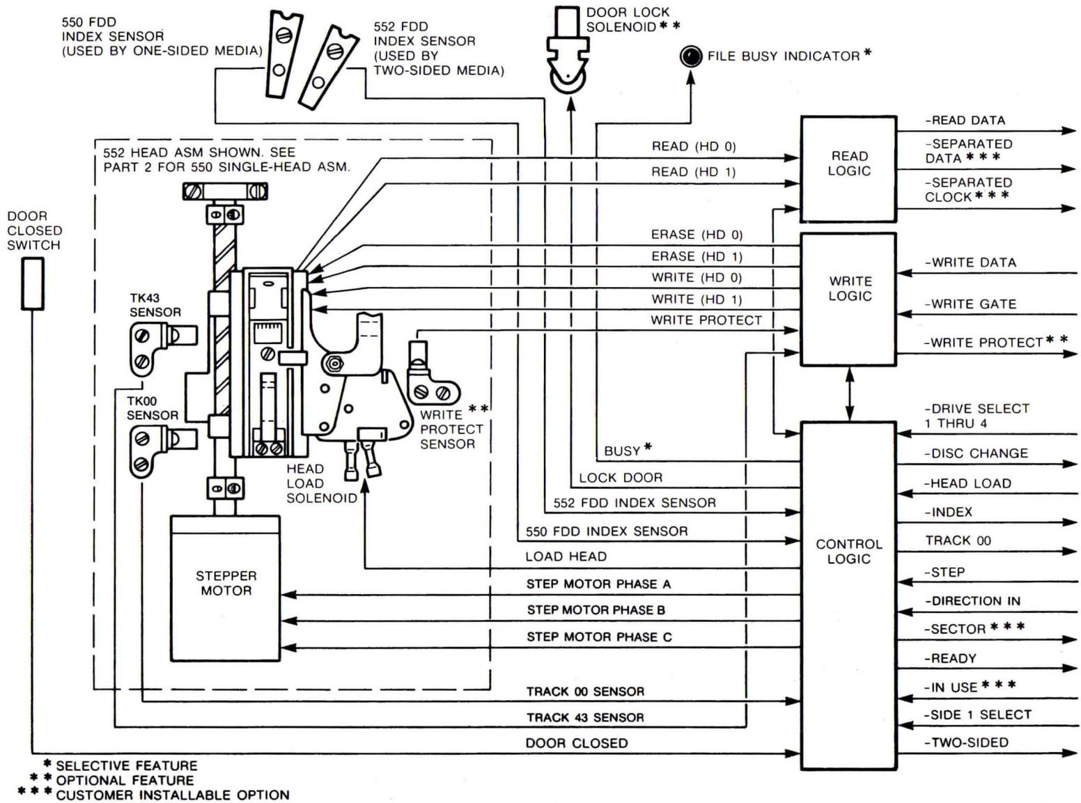
FIGURE 1-2. 550/552 FLEXIBLE DISC DRIVE FUNCTIONAL DIAGRAM (Part 1 of 2)
