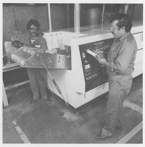
Memorex sub-assembly plant in Nogales, Mexico utilizes new equipment in their wave soldering system.
