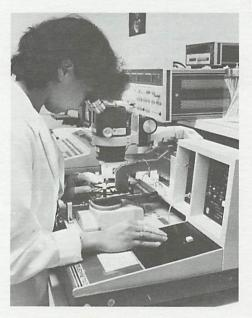
Thin-film head technology requires a whole new testing system—statistical process control analysis. Here a technician uses a wafer probe tester to check the characteristics of a wafer full of thin-film heads.
