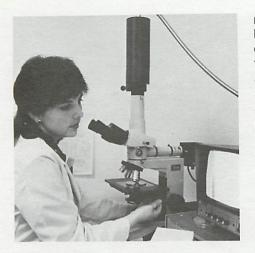
This video measuring system is used to determine the thin-film head track width from pole to pole on each head contained on individual wafers.
