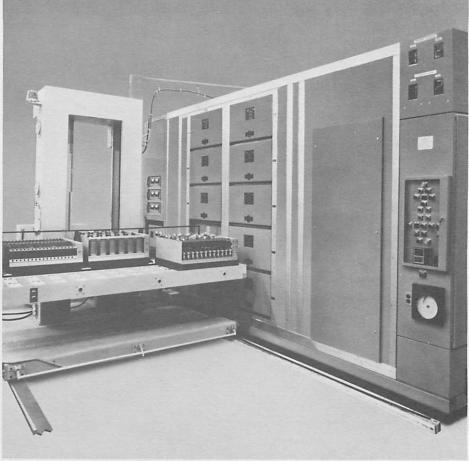
New "burn-in" equipment, as shown above, has been designed specifically for Memorex. Known as the Production Burn-In Facility for PCB's, this new equipment will be installed mid summer 1983.
