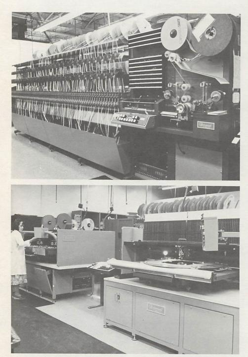
(Top) Receiving many reels of standard PCB components, a single reel is produced by this computerized sequencer machine. The machine is programmed to arrange the components, in a specific logical order, for use on the automatic insertion equipment. (Bottom) These automatic insertion machines are programmed to place components on the blank PC boards.
