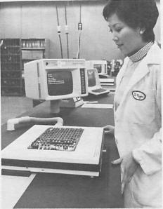
The "today" look (above) and the new "tomorrow" look (left) in circuit board test equipment typify some of the capital expenditures being made on the 3680 program. These PCB instruments test each individual component and assembly on every board. It tests all the possible combinations to check the functionality of the board to a very high level of accuracy.
