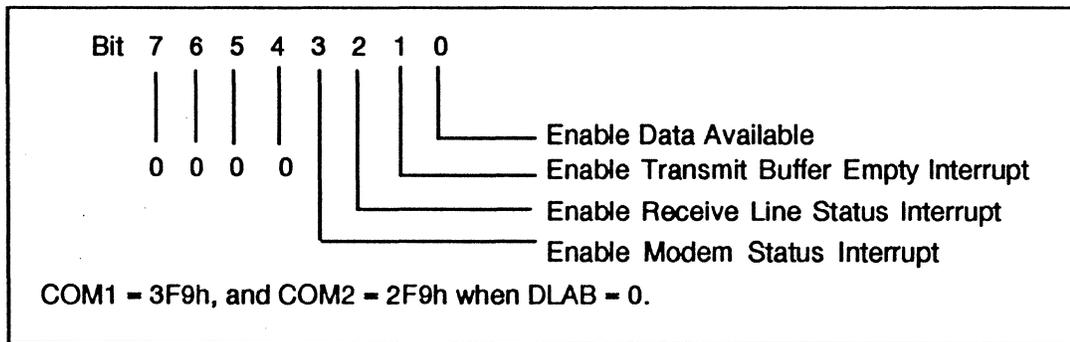
**Figure 2-72. Interrupt Enable Register**
