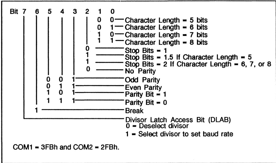
Figure 2-74. Line Control Register
