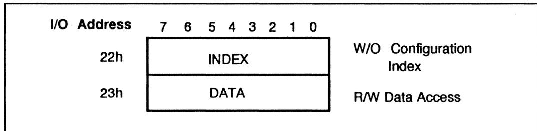
Figure 2-21. Configuration Register Access Ports
