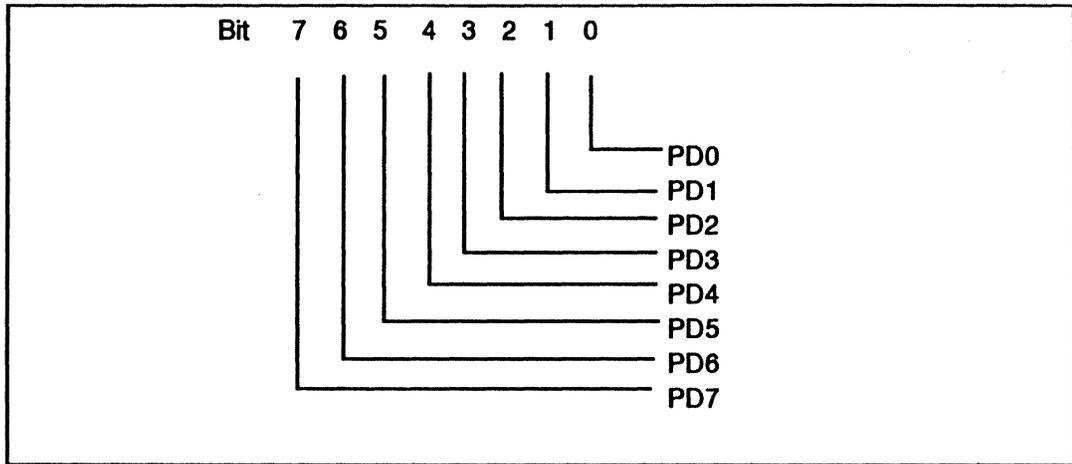
**Figure 2-68. Parallel Port Data Register**
