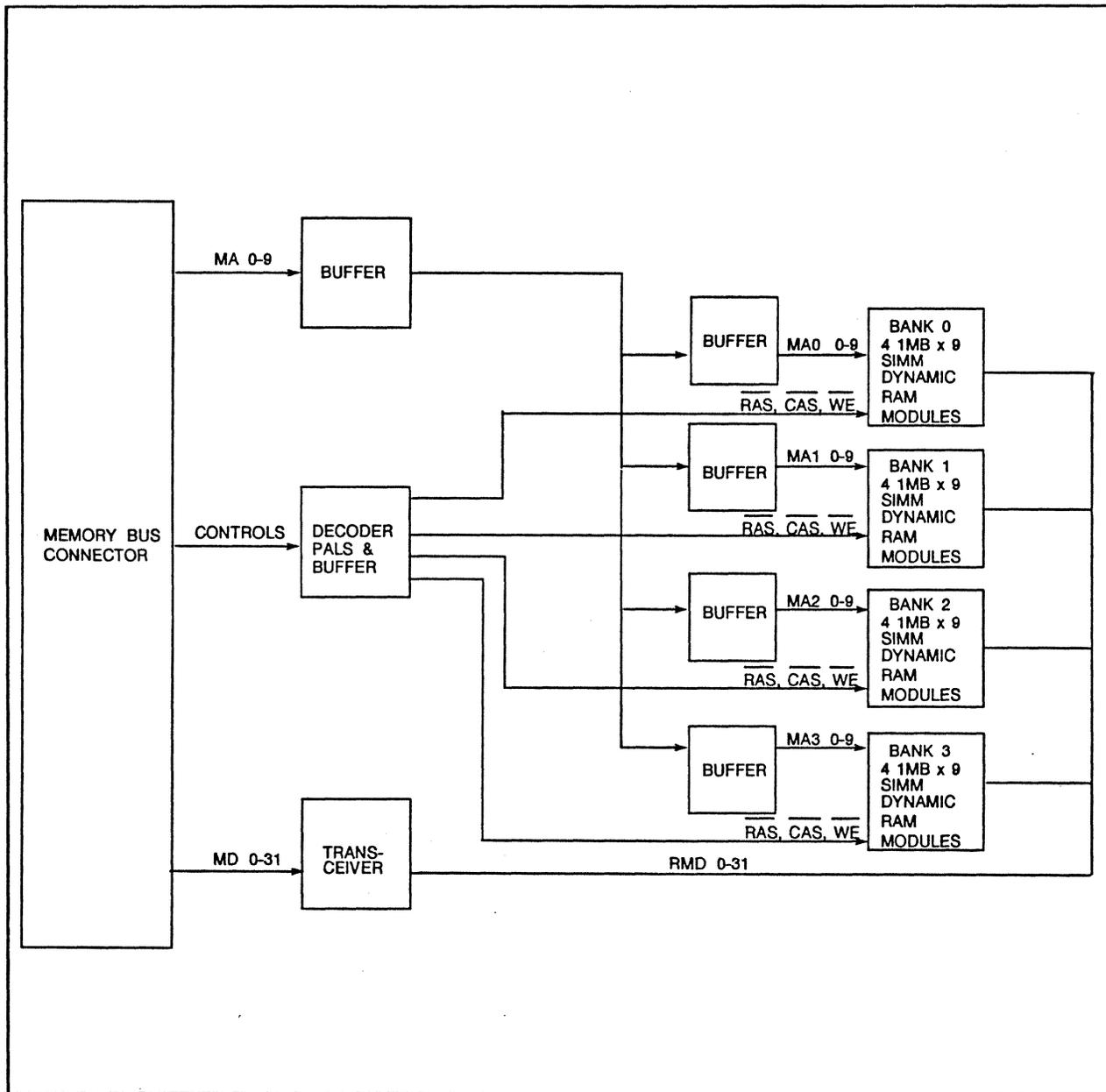
Figure 5-1. Memory Board Block Diagram
