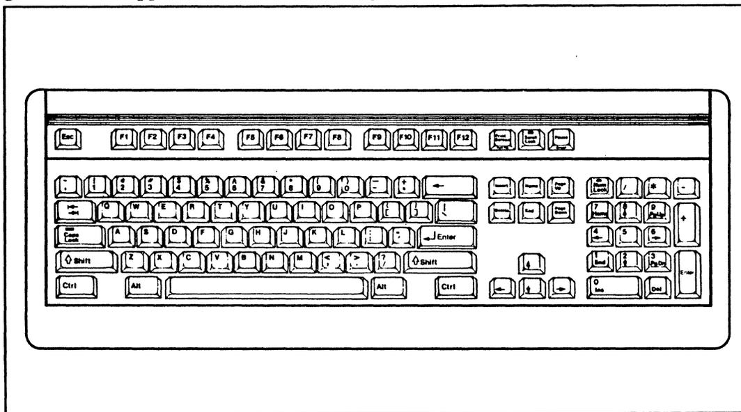
**Figure 4-2. Enhanced AT-Type Keyboard Layout**
