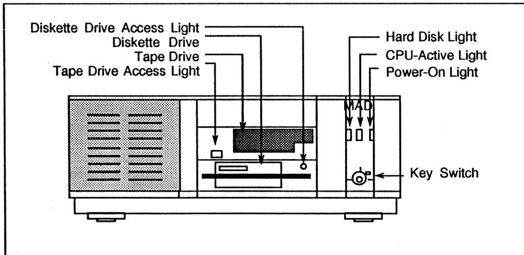
Figure 1-1. Typical System Unit
