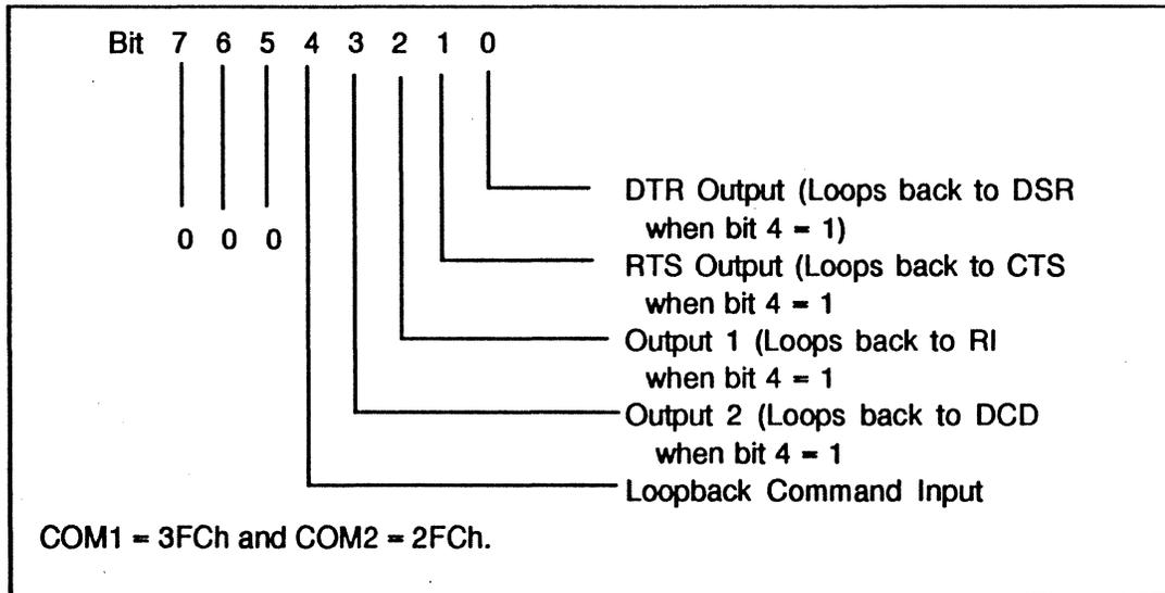
Figure 2-75. Modem Control Register
