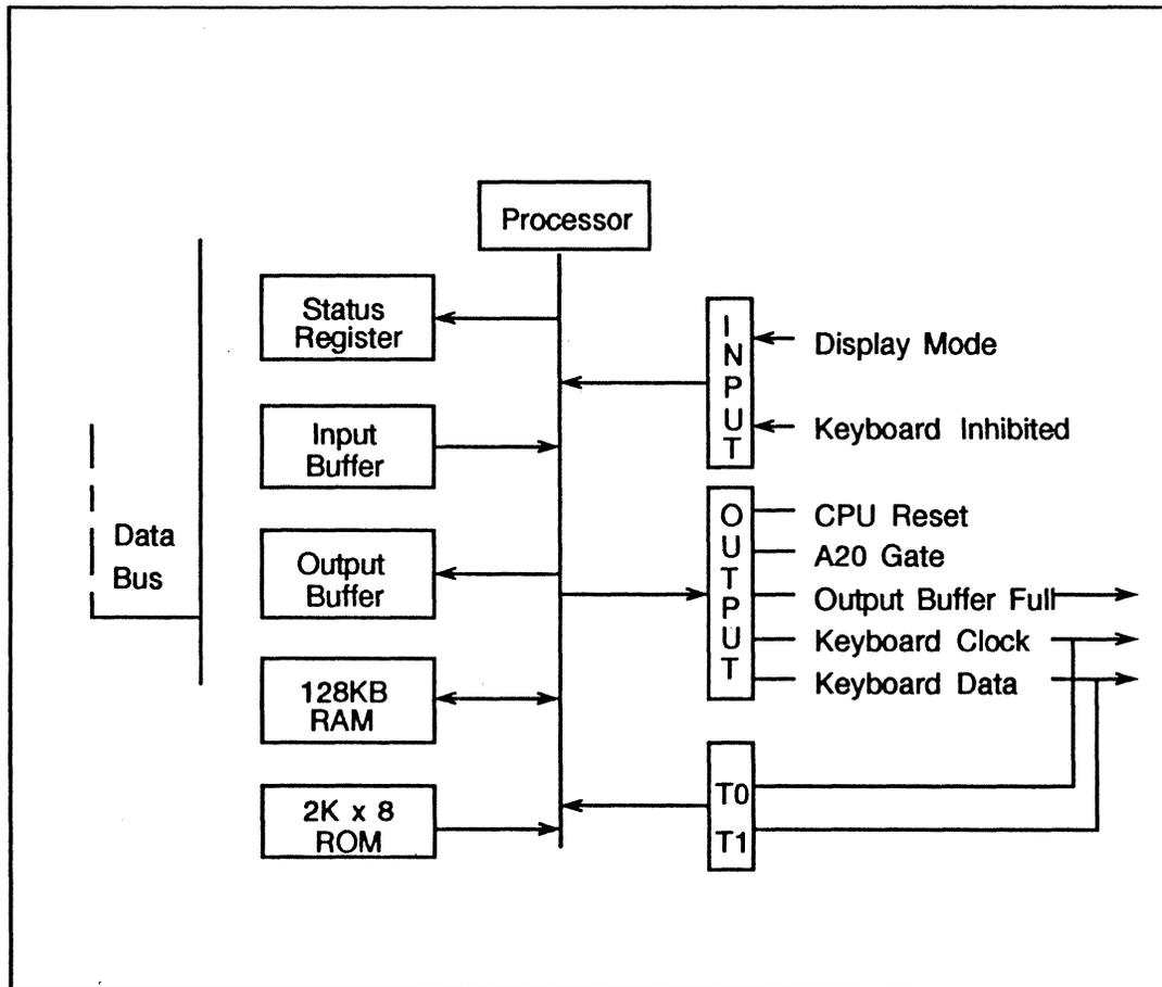
Figure 4-1. Keyboard Controller Block Diagram.
