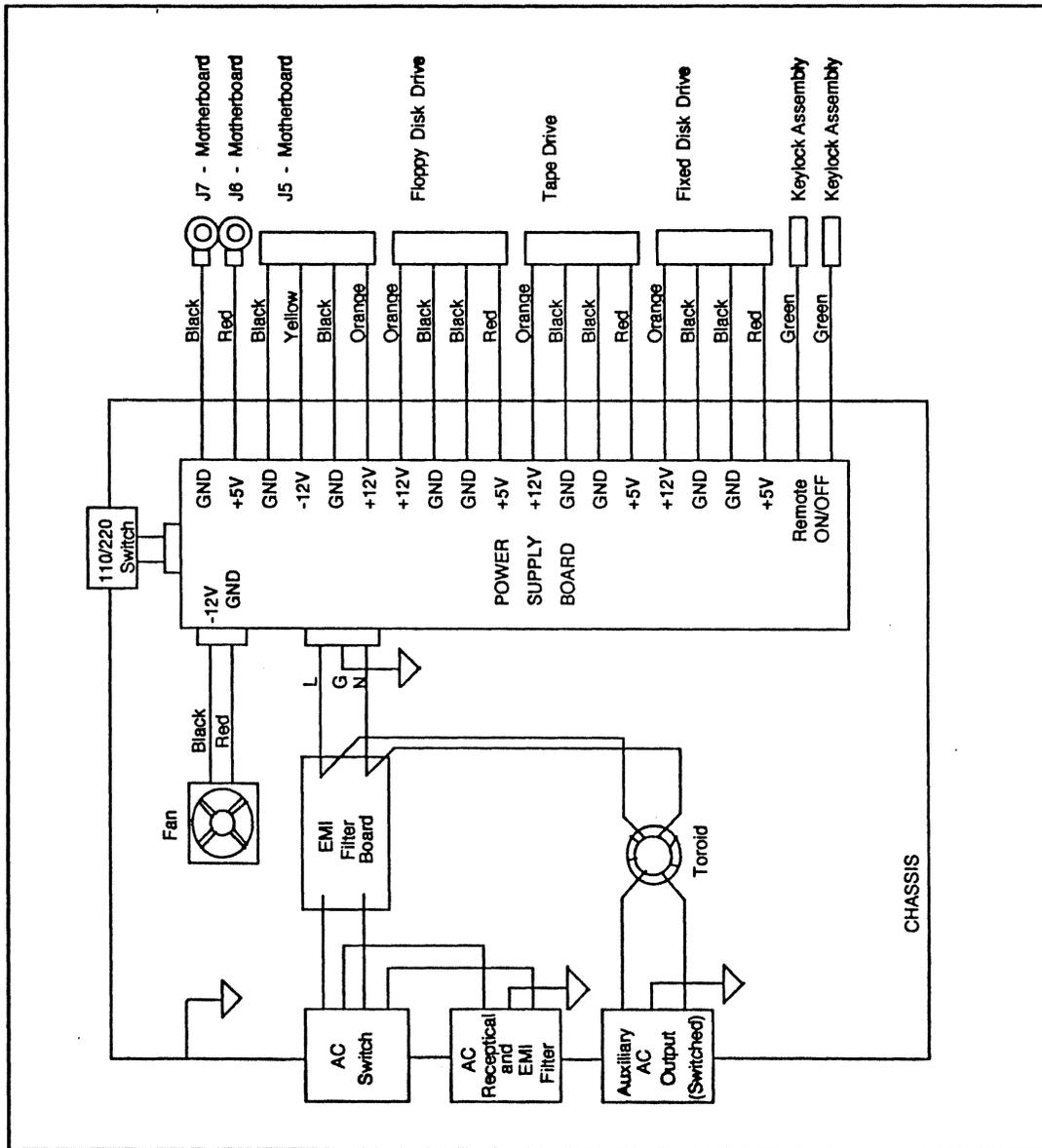
Figure 7-1. Power Supply Block Diagram
