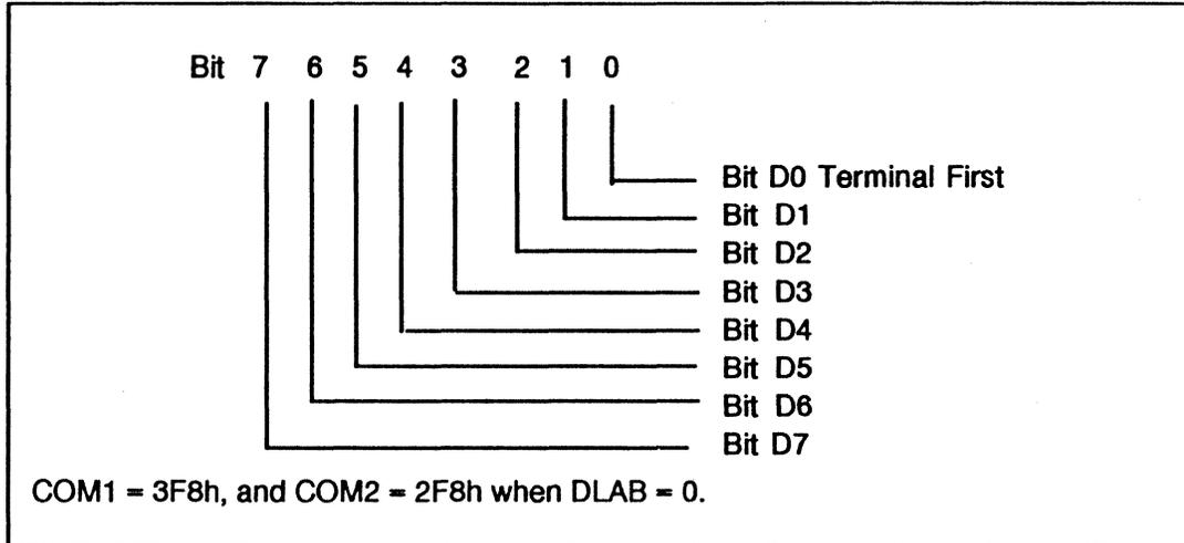
**Figure 2-71. Transmit/Receive Buffer Register**
