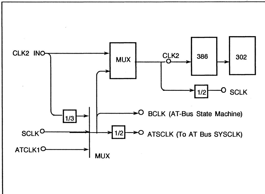
Figure 2-23. CLK2 and ATCLK Clock Selection
