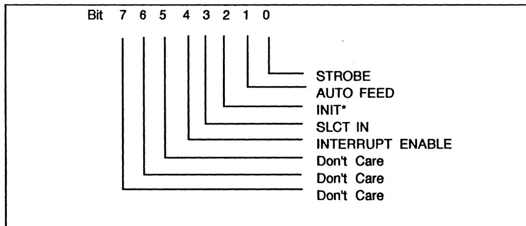
Figure 2-67. Parallel Port Control Register
