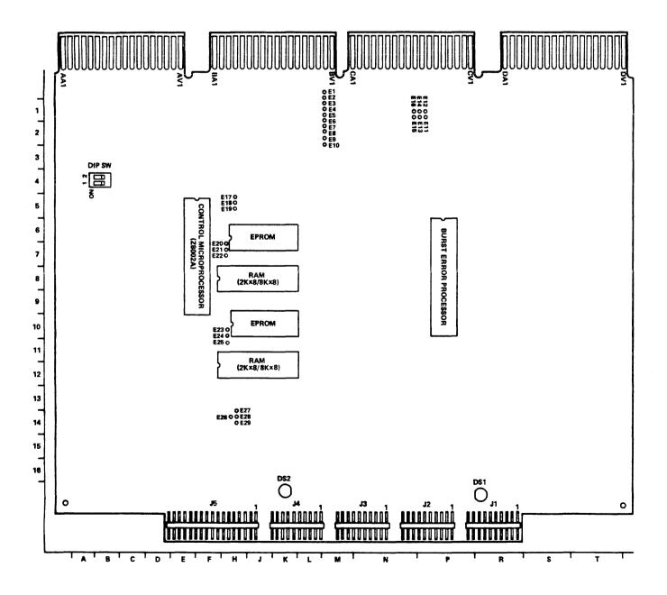
Figure 3-1. RL101 Board Layout
