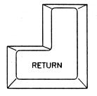
This key is used instead of the (Control M) combination to send the ASCII carriage return code  $\langle CR \rangle$ .
