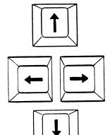
These keys generate codes that move the cursor in the direction of the arrows on the keys, one character cell per keystroke. When these keys are held down their codes are generated repeatedly.
