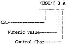
This command would cause the terminal to move the cursor up 3 lines. The "3" is interpreted as a number of lines in relation to the "A", which indicates cursor movement upwards.
