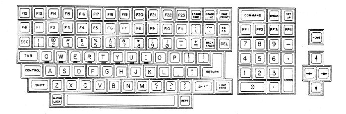
The keys grouped immediately to the left of the cursor pad are arranged in six rows. The top two rows contain special purpose keys whose functions are discussed below. The bottom four rows constitute a numeric keypad similar to those found on standard office machines.
