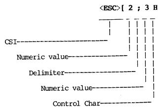
This command would cause the terminal's cursor to move to line 2, column 3. Note that the final character "H" indicates cursor movement in terms of lines and columns; accordingly, it determines the number of numeric values which are included.
