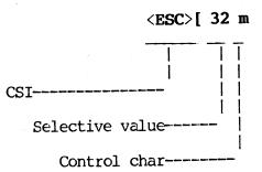
This command would cause the terminal to display subsequently received text with the foreground color green. Note that "32" indicates foreground display in green only in relation to "m". Foreground display in green is treated here as a subfunction of a general function called "select graphic rendition".
